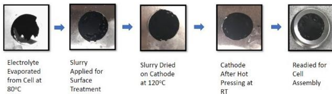
Figure 2: Cathode treatment evolution for moderate surface damage.
