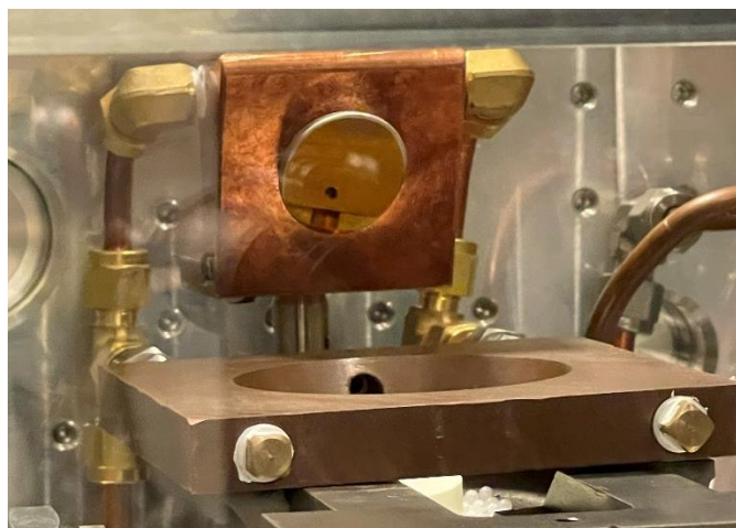
Supplemental Figure 7: New water-cooled mirror holder with a flat mirror installed. Even with the flat mirror partially occluding the light source, the water cooling was sufficient to keep the mirror cool and intact.
