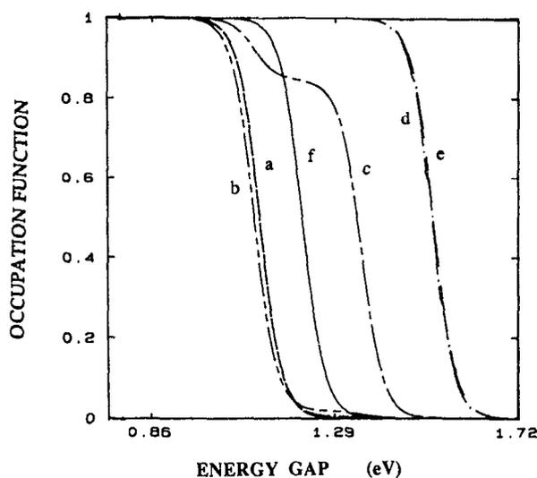
FIG. 8. Occupation function at  $x = 0.81$  for  $\psi_{DS} = 2.5$  V and  $\psi_G$  turning on to 5.0 V. Each curve is for a different time: (a)  $10^{-14}$  s, (b)  $10^{-6}$  s, (c)  $10^{-5}$  s, (d)  $10^{-4}$  s, (e)  $10^{-1}$  s to steady state. (f) Equilibrium occupation function.
