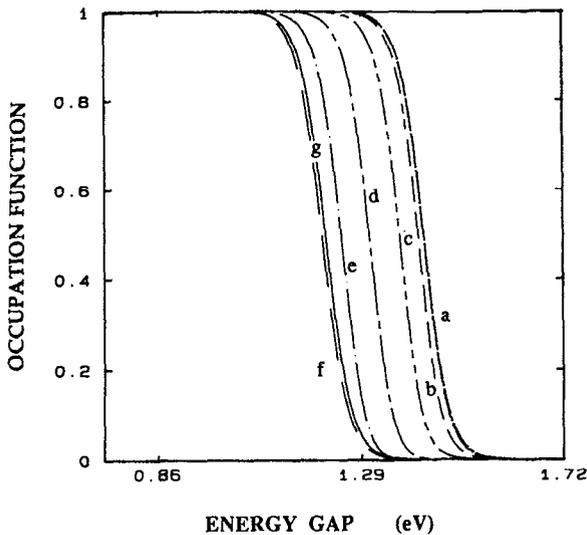
FIG. 11. Occupation function at  $x = 0.5$  for  $\psi_{DS} = 2.5$  V and  $\psi_G$  turning on to 5.0 V. Each curve is for a different time: (a)  $10^{-14}$  s, (b)  $10^{-7}$  s, (c)  $10^{-6}$  s, (d)  $10^{-5}$  s, (e)  $10^{-4}$  s, (f)  $10^{-1}$  s to steady state. (g) Equilibrium occupation function.
