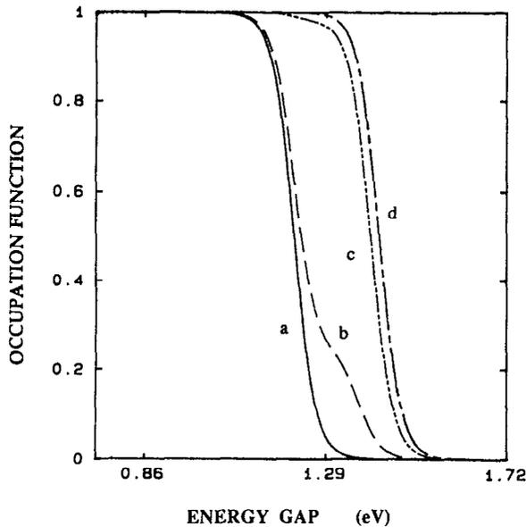
FIG. 4. Occupation function at  $x = 0.23$  for  $\psi_{DS} = 0.25$  V and  $\psi_G = 0.50$  V. Each curve is for a different time: (a)  $10^{-14}$  s (b)  $10^{-6}$  s (c)  $10^{-5}$  s (d)  $10^{-3}$  s to steady state. Energy of 1.72 eV is located at the mobility edge of the conduction band.
