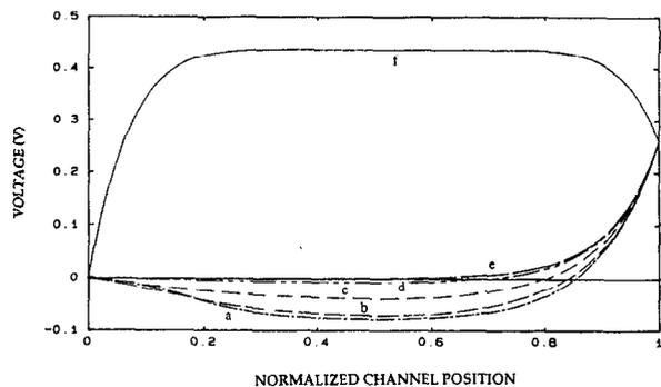
FIG. 9. Electrostatic potential vs distance for  $\psi_{DS} = 0.25$  V and  $\psi_G$  turning off from 0.50 V to zero. (a)  $10^{-14}$  s, (b)  $10^{-8}$  s, (c)  $10^{-7}$  s, (d)  $10^{-6}$  s, (e)  $10^{-5}$  s to steady state. (f) Voltage before gate was turned off.
