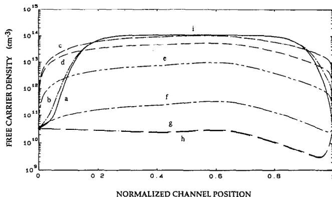
FIG. 10. Free-electron concentration vs distance for  $\psi_{DS} = 0.25$  V and  $\psi_G$  turning off from 0.50 V to zero. Each curve is for a different time: (a)  $10^{-14}$  s, (b)  $10^{-10}$  s, (c)  $10^{-8}$  s, (d)  $10^{-7}$  s, (e)  $10^{-6}$  s, (f)  $10^{-5}$  s, (g)  $10^{-4}$  s, (h)  $10^{-1}$  s to steady state. (i) Free-carrier density before gate was turned off.
