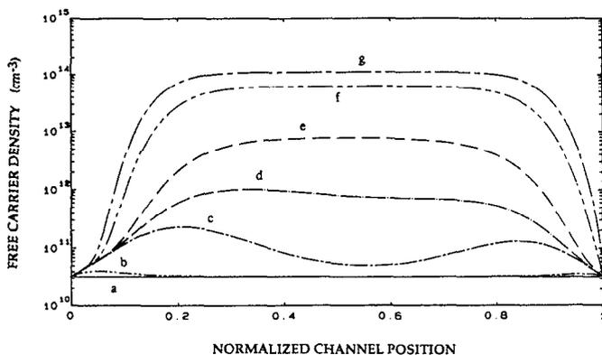
FIG. 2. Free-electron concentration vs distance for  $\psi_{DS} = 0.25 \text{ V}$  and  $\psi_G = 0.50 \text{ V}$ . Each curve is for a different time: (a)  $10^{-14} \text{ s}$ , (b)  $10^{-10} \text{ s}$ , (c)  $10^{-8} \text{ s}$ , (d)  $10^{-7} \text{ s}$ , (e)  $10^{-6} \text{ s}$ , (f)  $10^{-5} \text{ s}$ , (g)  $10^{-4} \text{ s}$  to steady state.
