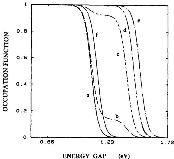
FIG. 7. Occupation function at  $x = 0.5$  for  $\psi_{DS} = 2.5$  V and  $\psi_G$  turning on to 5.0 V. Each curve is for a different time: (a)  $10^{-14}$  s, (b)  $10^{-7}$  s, (c)  $10^{-6}$  s, (d)  $10^{-5}$  s, (e)  $10^{-4}$  s to steady state. (f) Equilibrium occupation function.
