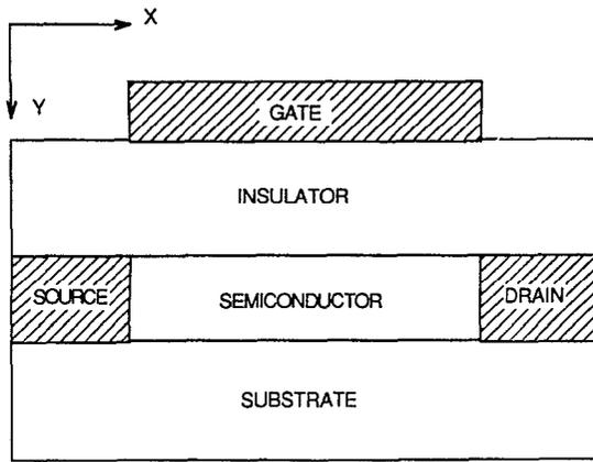
FIG. 1. Device geometry of *a*-Si:H thin-film transistor under consideration.
