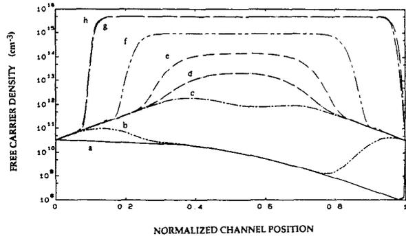
FIG. 6. Free-electron concentration vs distance for  $\psi_{DS} = 2.5$  V and  $\psi_G$  turning on to 5.0 V. Each curve is for a different time: (a)  $10^{-14}$  s, (b)  $10^{-10}$  s, (c)  $10^{-8}$  s, (d)  $10^{-7}$  s, (e)  $10^{-6}$  s, (f)  $10^{-5}$  s, (g)  $10^{-4}$  s, (h)  $10^{-2}$  s to steady state.
