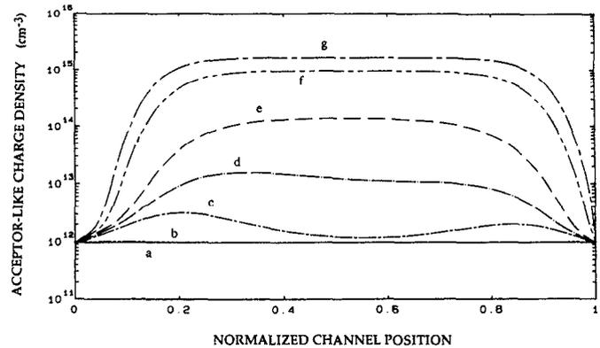
FIG. 3. Charged acceptorlike state concentration vs distance for  $\psi_{DS} = 0.25 \text{ V}$  and  $\psi_G = 0.50 \text{ V}$ . Each curve is for a different time: (a)  $10^{-14} \text{ s}$ , (b)  $10^{-10} \text{ s}$ , (c)  $10^{-8} \text{ s}$ , (d)  $10^{-7} \text{ s}$ , (e)  $10^{-6} \text{ s}$ , (f)  $10^{-5} \text{ s}$ , (g)  $10^{-4} \text{ s}$  to steady state.
