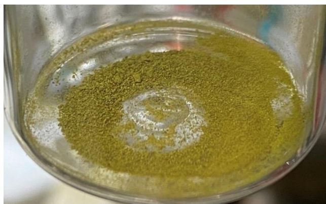
Figure S1. (a) As-synthesized DMF washed crystals of LiMnPS 4 synthesized from metathesis route ( \text{Li}_3\text{PS}_4 + \text{MnCl}_2 ).
