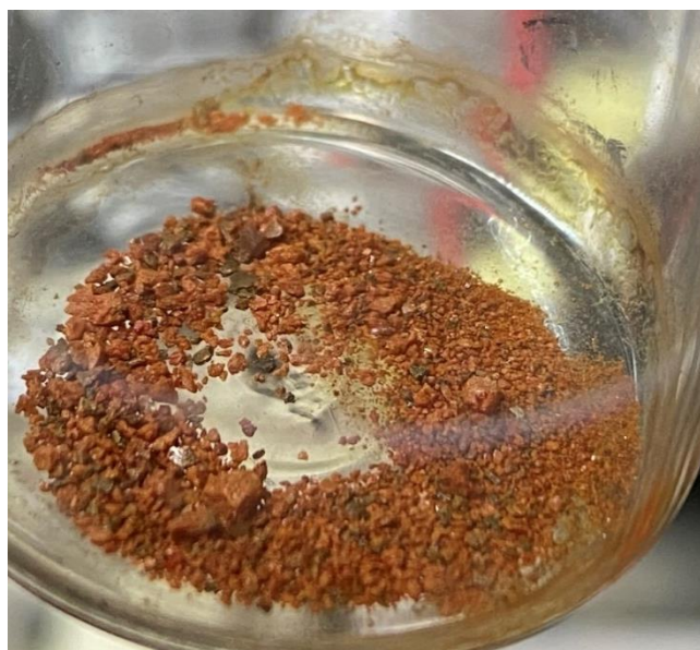
Figure S1. As-synthesized, DMF-washed crystals of \text{Na}_8\text{Mn}_2(\text{Ge}_2\text{Se}_6)_2 .
