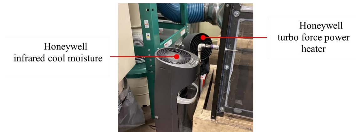
Figure 4. The Honeywell turbo force power heater and the Honeywell infrared cool moisture humidifier
