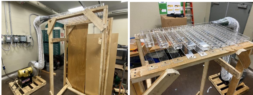
Figure 5. Laboratory built CAC based on optimum design from CFD simulations
