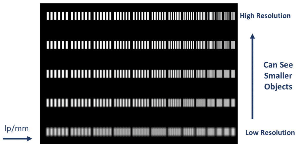
Figure 1.6. The resolving power of an X-ray imaging system is commonly measured through a test pattern. [97]
