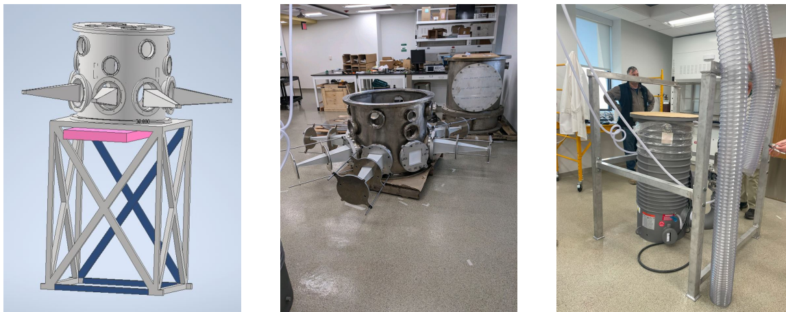
Figure 2.7. The new, state-of-the-art rotational spectrometer under construction at Missouri S&T as part of an NSF MRI grant. From left to right: Figure 1.) Initial CAD design for the chamber and stand. Figure 2.) The chamber as of the time of writing. Figure 3.) The stand as of the time of writing.
