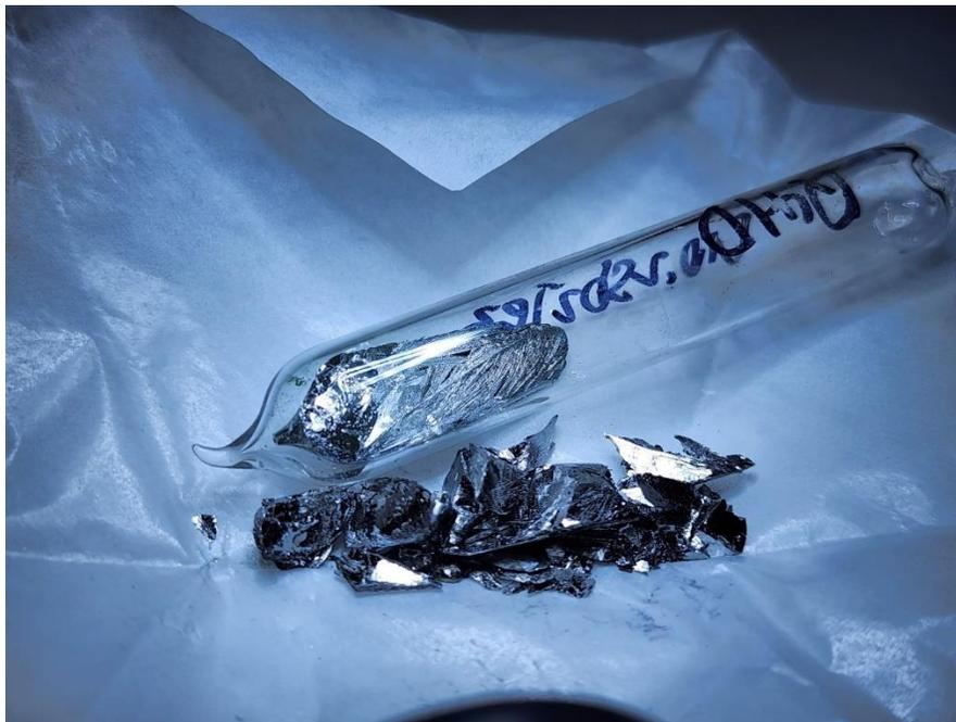
Figure 3-5 Samples of  $\text{Cr}_{0.2}\text{Sb}_2\text{Te}_3$
