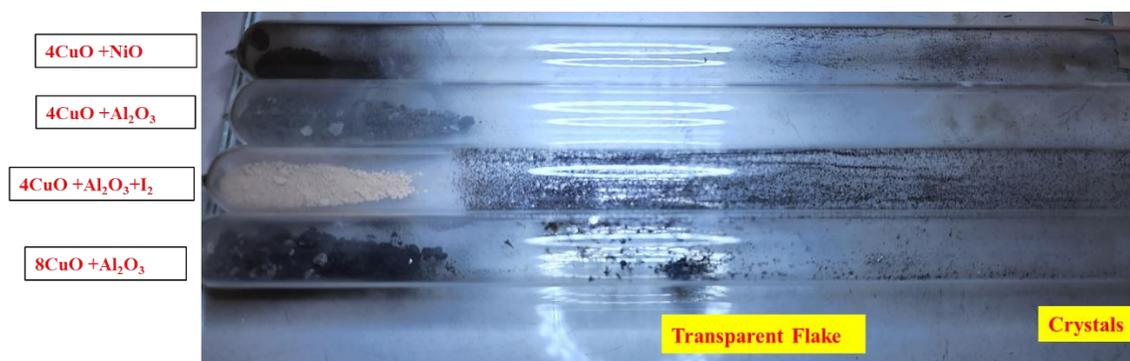
Figure 5-8 Results after Crystal Thermal Transport
