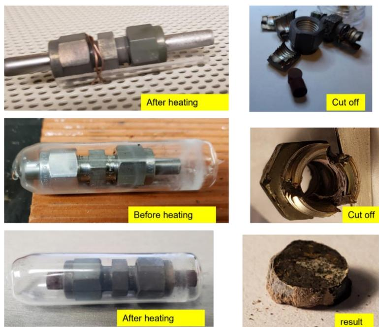
Figure 5-4 Results of Pressure-Seal Swagelok
