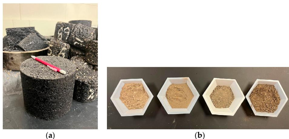
**Figure 2.** (a). Compacted HMA (b). Crushed HMA increasing in asphalt percent from left to right (4.5, field, 5.5, 6%).
