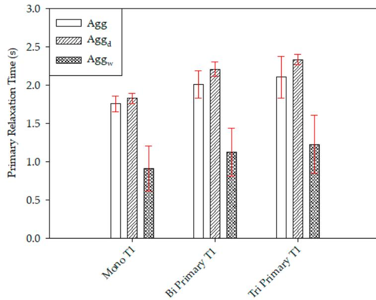
**Figure 6.** T<sub>1</sub> comparison of the aggregate in normal, dry, and wet conditions with standard deviation (red bars).
