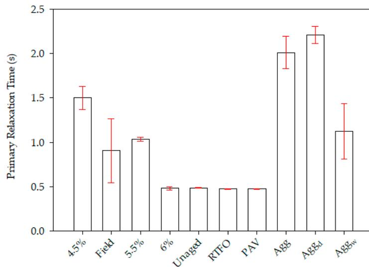
**Figure 7.** T<sub>1</sub> relaxation times from the biexponential fit of field HMA, lab HMA (4.5%, 5.5 6%), unaged binder, aged binders (PAV, RTFO), and aggregate (normal, dry, wet) with standard deviation (red bars).
