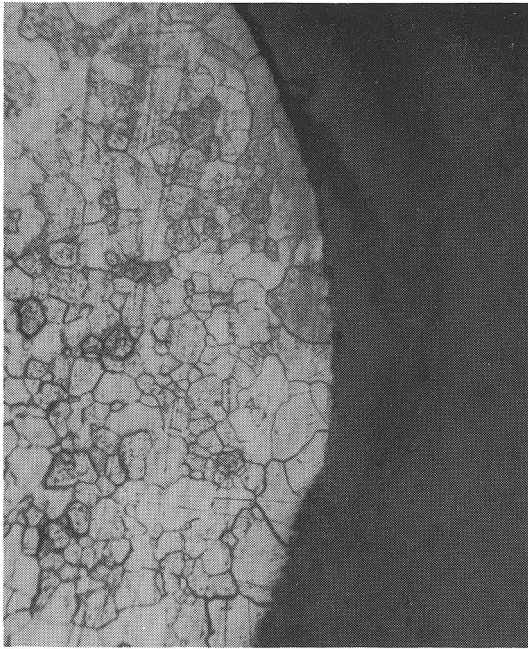
Figure 48. Molybdenum Surface, UE-1. (125x), Murakami's Reagent.
