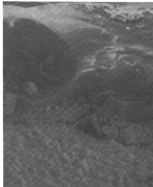
Figure 67. SEM Photomicrograph of Interface Showing Oxide Layer and Texture of Underlying Molybdenum Surface. (1000x).
