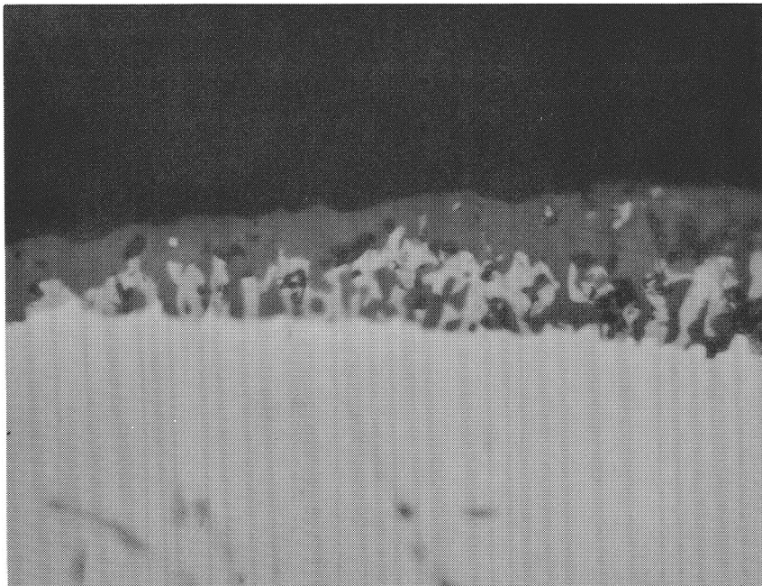
Figure 21. Slag-Metal Interface, Mo r -2B. (1300x), unetched.
