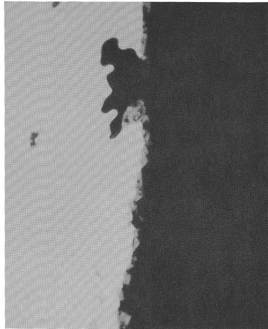
Figure 65. Slag-Metal Interface Showing Pitting Corrosion, A Four-Hour Test in UE Slag, p_{O_2}=10^{-7} atm. (1000x), unetched.
