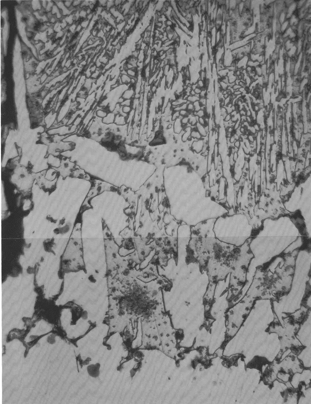
Figure 34. Alloy on Cathode Pin, Upper Section, 1400°C. (1300x), nital etch.
