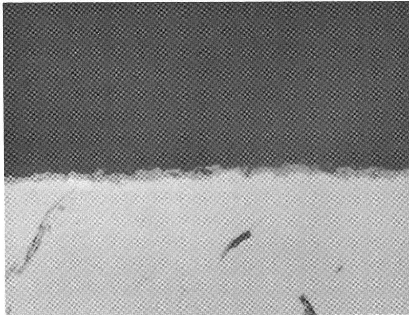
Figure 19. Slag-Metal Interface, Mo \gamma -2T. (1300x), unetched.
