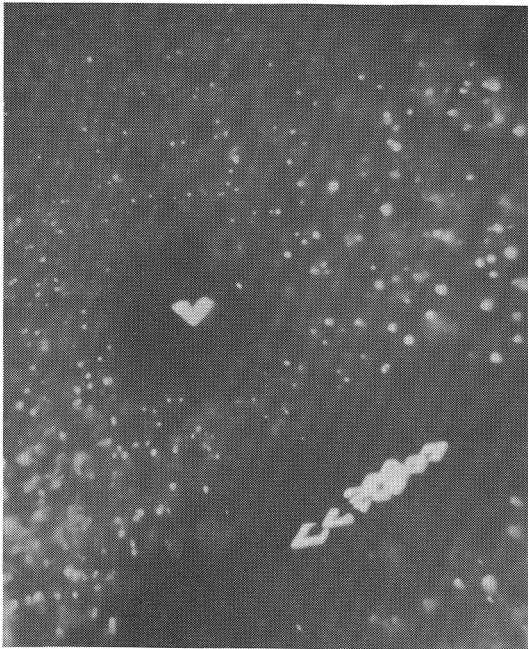
Figure 56. Precipitate and Debris in Slag Between Electrodes, Electrical Current Tests. (1300x), unetched.
