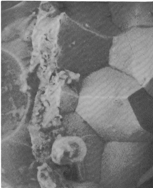
Figure 66. SEM Photomicrograph of Molybdenum-Slag Interface Showing Oxide Reaction Layer. (1500x).
