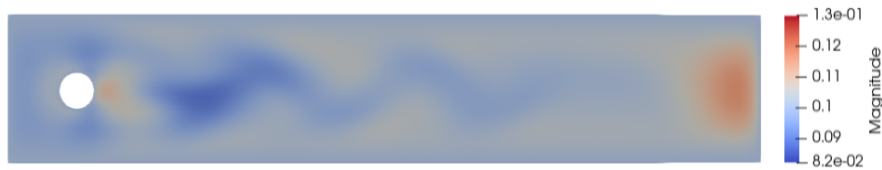
Figure 1.22. Algorithm (1.3.1) solution when \epsilon = 0 for magnetic field at time T = 8.8 with \nu = 0.001 , \gamma = 0.1 and \Delta t = 0.001 .
