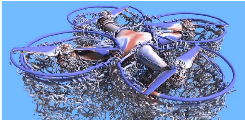
Figure 2.1. Simulation of UAV Downwash, where the White Areas below the UAV Represent Locations with Pressures that Vary from Ambient Pressure [119]
