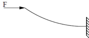
Figure 5.11 Compliant Segment of Class 1A Slider-Crank, CFM with Reaction Force.
