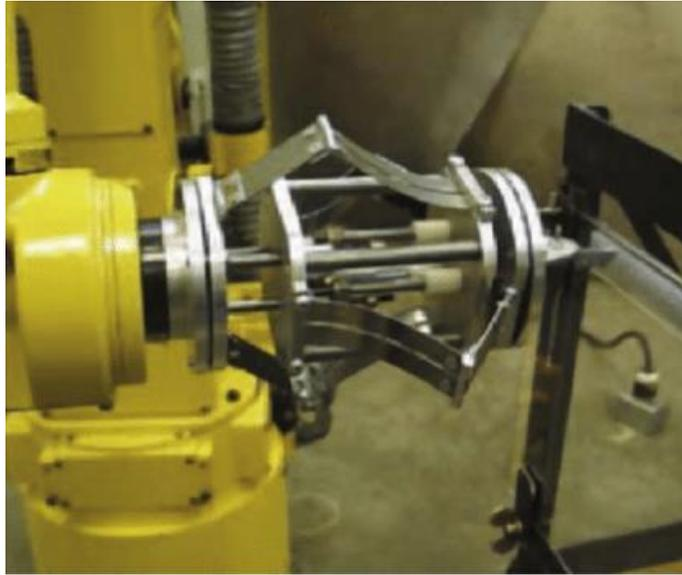
Figure 1.12 Constant-Force Robot End Effector [42]
