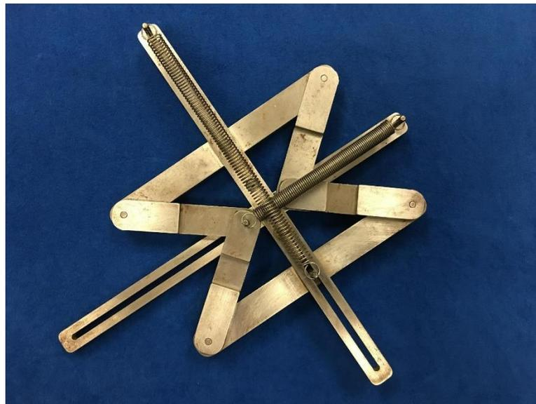
Figure 1.8 SIPMOP Constant Force Mechanism [21, 22]
