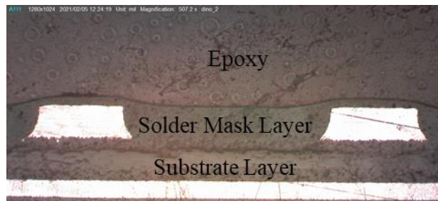
Figure 1.2. Cross-section of a pair of coupled microstrip.
