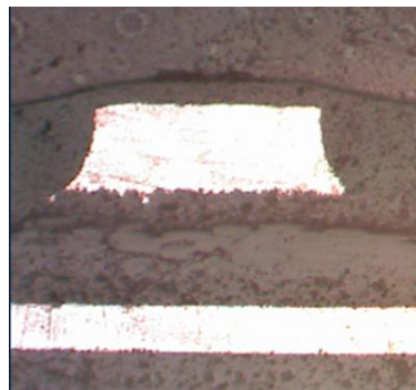
Figure 13. The cross-sectional geometry for the microstrip.
