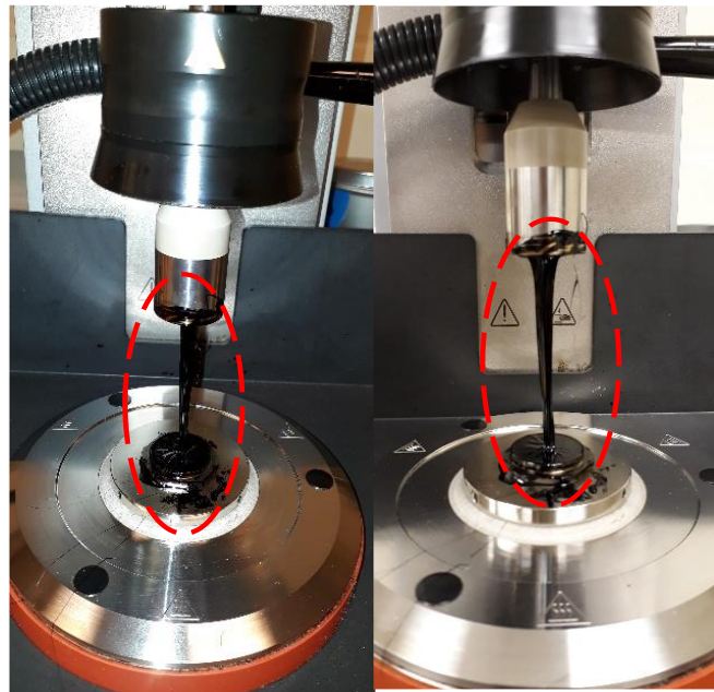
Figure 8. The elasticity of EAB from a mix containing ECR.
