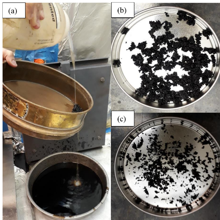
Figure 1. Dissolution test process; (a) Colorless filtrate at the end of the washing process, (b) Extracted CRM particles after the washing process, and (c) Extracted CRM particles after drying in the oven.
