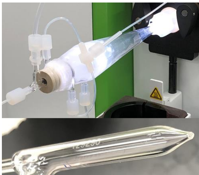
Figure 1.3. Top: Single cell sample introduction system with Asperon™ spray chamber. Bottom: Meinhard HEN single cell nebulizer.
