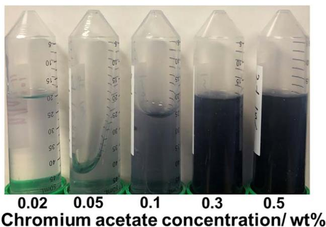
Fig. 7—Gelant samples after 150 days at 45°C (1 wt% polymer, pH 3.5).
