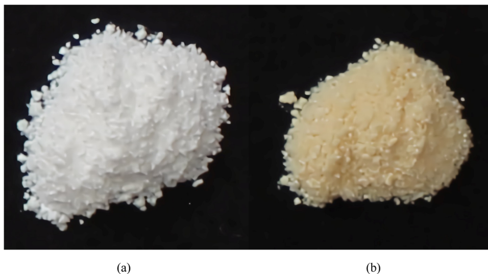
Figure 11. Photographs of (a) as-made Fe-SSZ-70 and (b) calcined Fe-SSZ-70.
