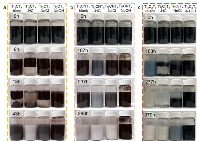
Figure 1. Photographs of MXene aqueous colloids being stored at 70 ^{\circ}\text{C} for the indicated times: (a) \text{Ti}_2\text{CT}_x\text{-blank} , \text{Ti}_2\text{CT}_x\text{-HCl} , \text{Ti}_2\text{CT}_x\text{-NaCl} , and \text{Ti}_2\text{CT}_x\text{-NaOH} ; (b) \text{Ti}_3\text{CNT}_x\text{-blank} , \text{Ti}_3\text{CNT}_x\text{-HCl} , \text{Ti}_3\text{CNT}_x\text{-NaCl} , and \text{Ti}_3\text{CNT}_x\text{-NaOH} ; (c) \text{Ti}_3\text{C}_2\text{T}_x\text{-blank} , \text{Ti}_3\text{C}_2\text{T}_x\text{-HCl} , \text{Ti}_3\text{C}_2\text{T}_x\text{-NaCl} , and \text{Ti}_3\text{C}_2\text{T}_x\text{-NaOH} .
