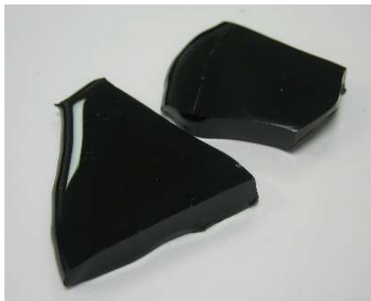
Figure 3.1. A typical black, opaque iron phosphate glass which results from melting, pouring and quenching.
