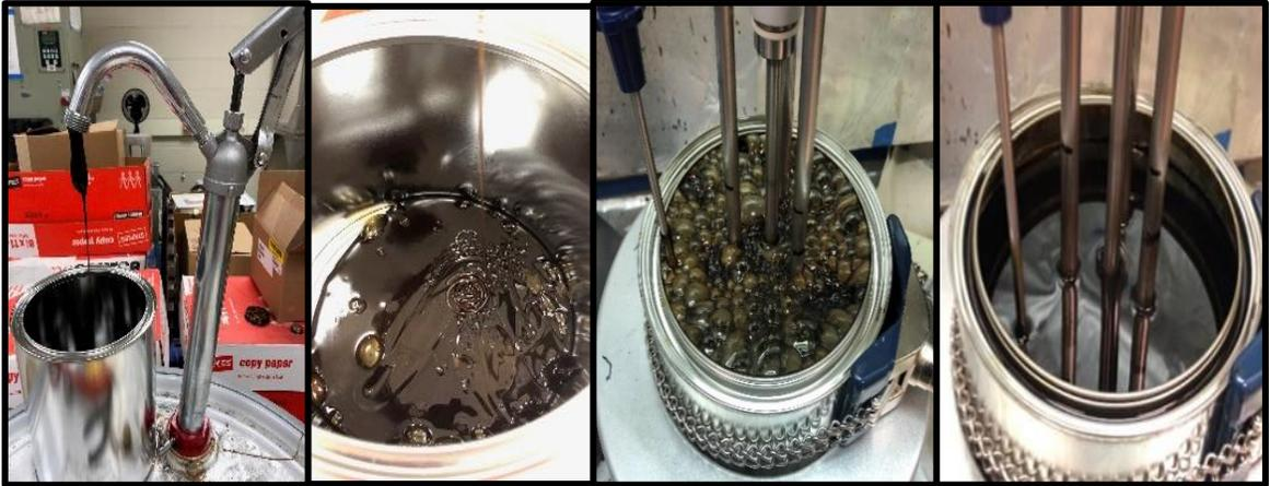
Figure 3.5 Guayule Resin Stages from Barrel to Heat Treatment.
