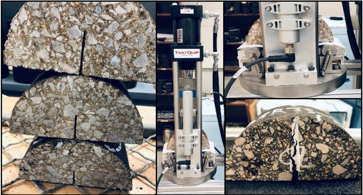
Figure 3.16 Technical Steps from the SCB Test Procedures [90].
