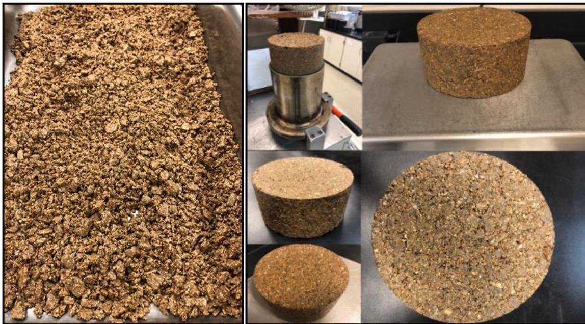
Figure 3.12 Pure Guayule Mixture (G2-Mix): Loose (Left) and Compacted (Right) [90].
