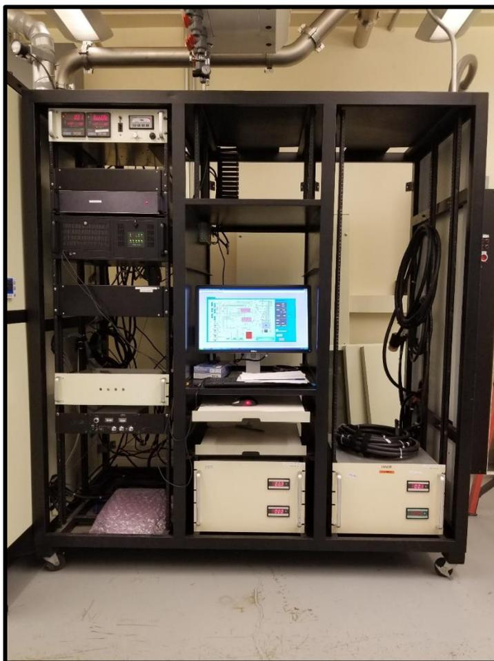
Figure 4.9 Metal-organic vapor deposition system for growth of un-doped and transition-metal doped zinc oxide – Control panel.
