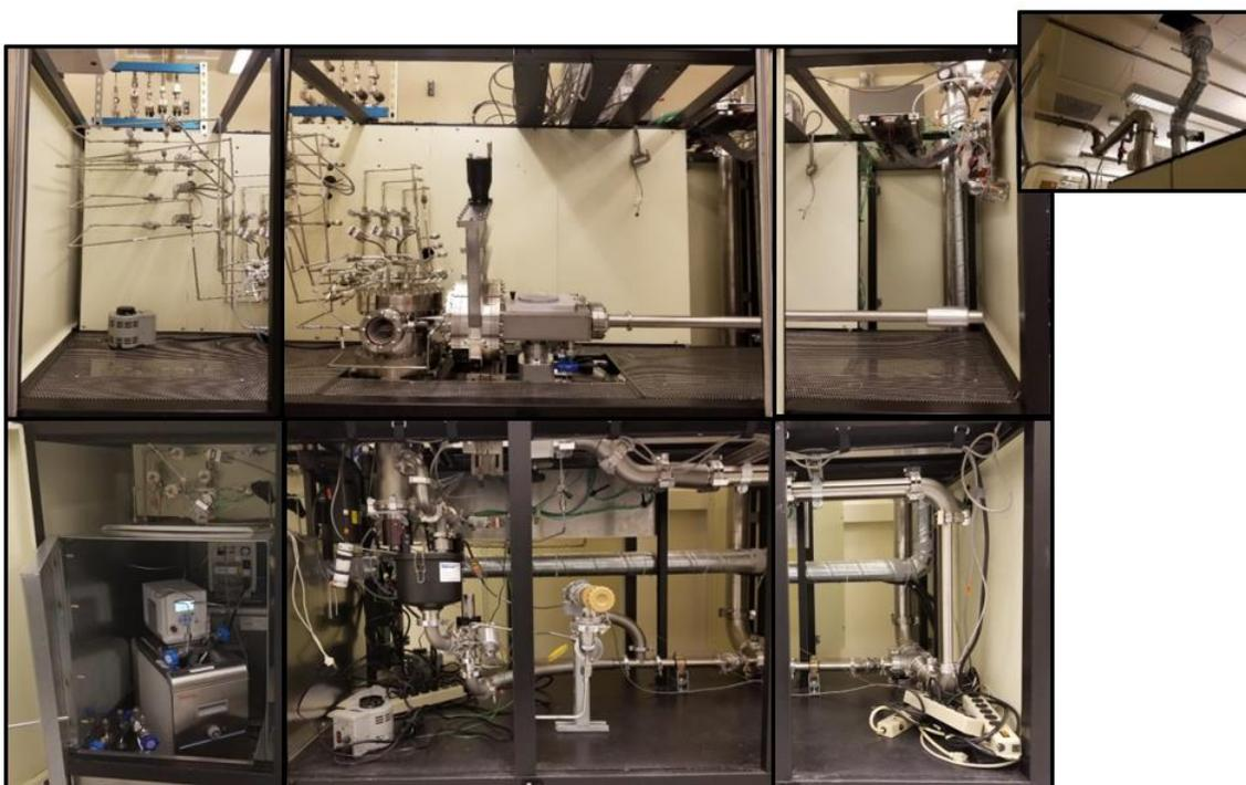
Figure 4.8 Metal-organic vapor deposition system for growth of un-doped and transition-metal doped zinc oxide.
