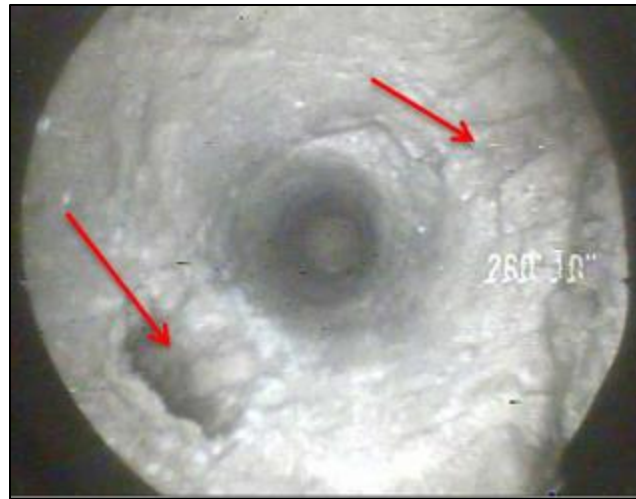
Figure 1. Downhole Camera Shows a 3-in Channel (Bijjani et al., 2018)
