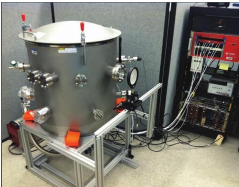
Figure 1.5. Outside View of Ohio State University NDP Instrument (from [8]).
