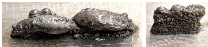
Figure 5. 2inch long deposit of Al4047 on an Al6061 substrate at room temperature (left) and 1inch long deposit of Al4047 on an Al6061 substrate preheated to 473K (right).
