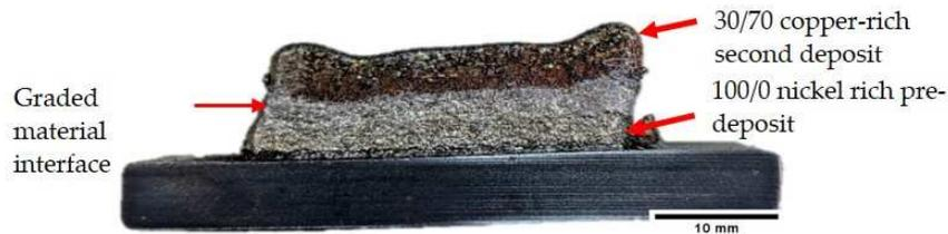
Figure 9. Copper-nickel FGM deposit fabricated with 100/0 as the pre-deposit and 30/70 as the second deposit. Set 3 duty cycle ramp down parameter were used at the dissimilar material interface.
