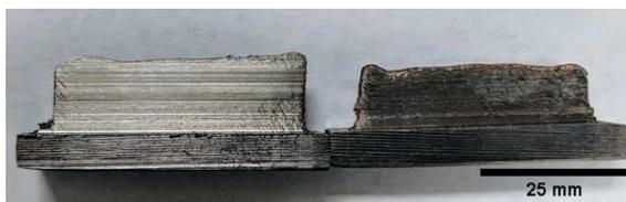
Figure 4. Machined thin-wall deposits of solely nickel-rich 100/0 (left) and copper-rich 30/70 (right) with a significant difference in overall height for the same 40 layers of deposition.
