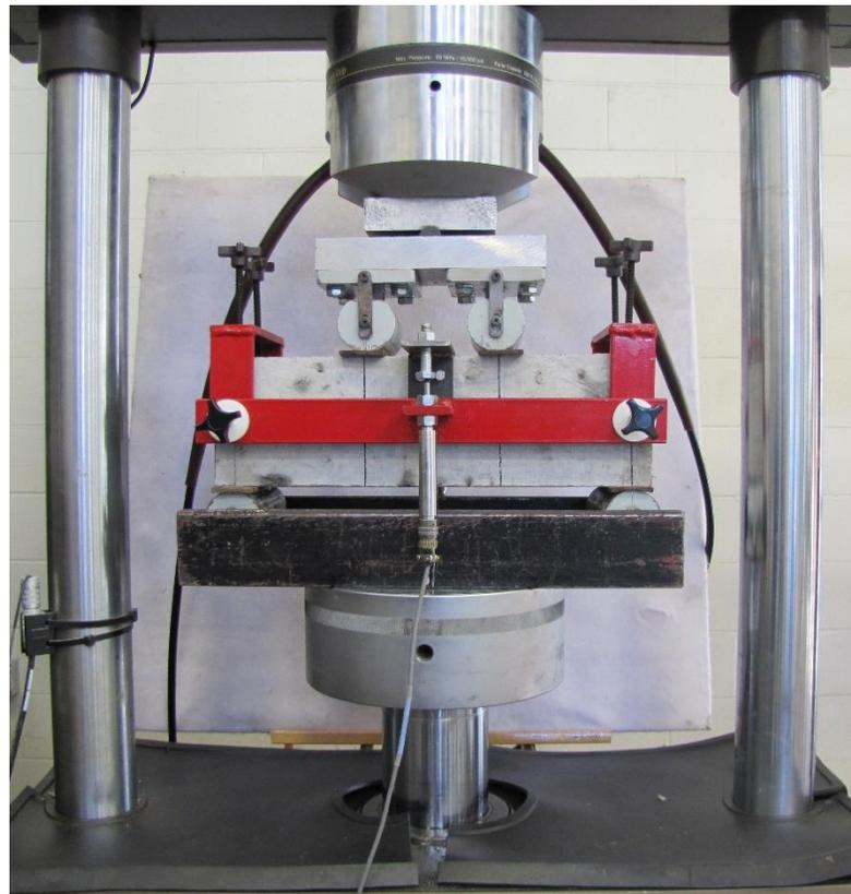
Figure 3.16. ASTM C1609 test setup
