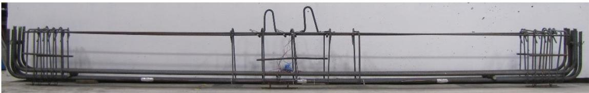
Figure 3.11. Reinforcing cage for B18
