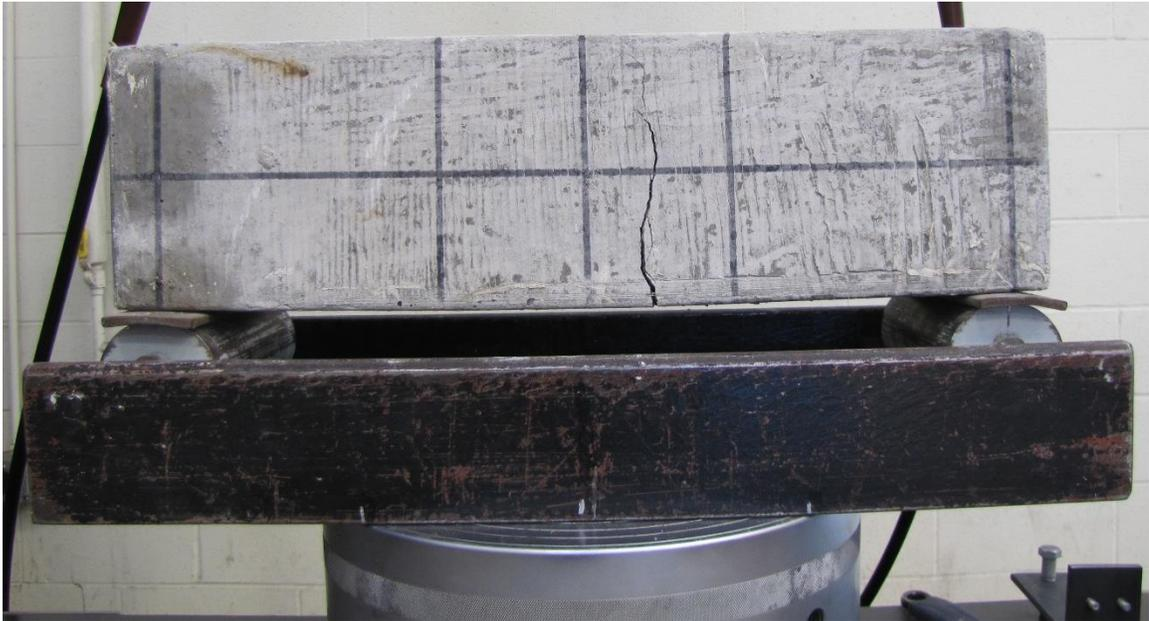
Figure 4.1. Typical ASTM C1609 beam after testing
