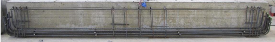
Figure 3.12. Reinforcing cage for B24
