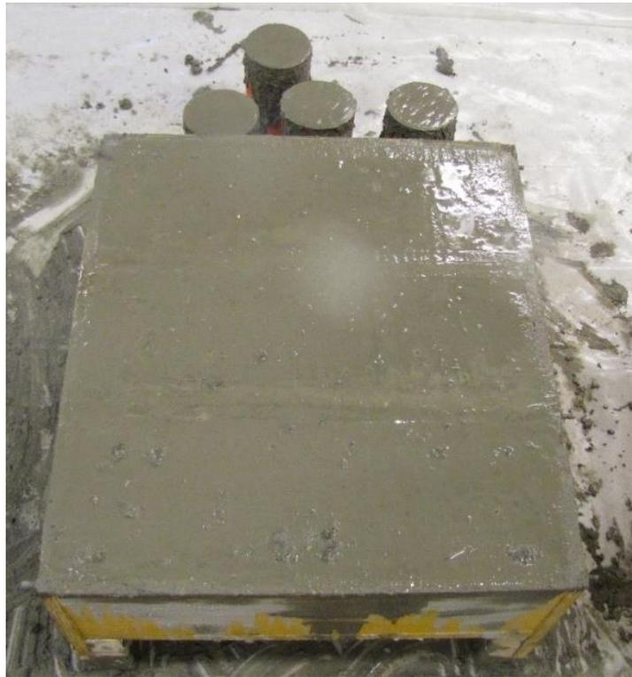
Figure 3.6. Beams and cylinders after consolidation
