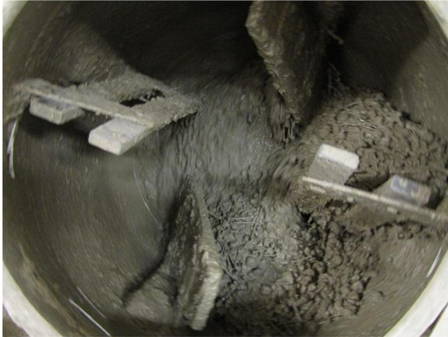
Figure 3.5. Concrete batching process after fiber addition
