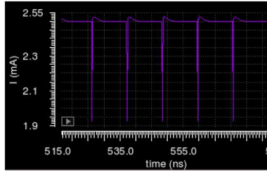
Figure 2.23 Current Drawn on Power Net for Current Mode Differential Driver.
