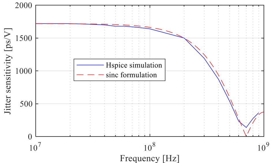
Figure 3.44 Calculated and Simulated PSIJ Sensitivity Comparison.
