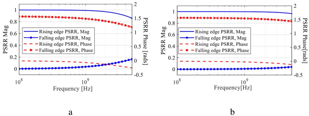
Figure 2.12 PSRR for Each stage in Inverter Chain. a) #1-#7 Stages. b) Output Stage.
