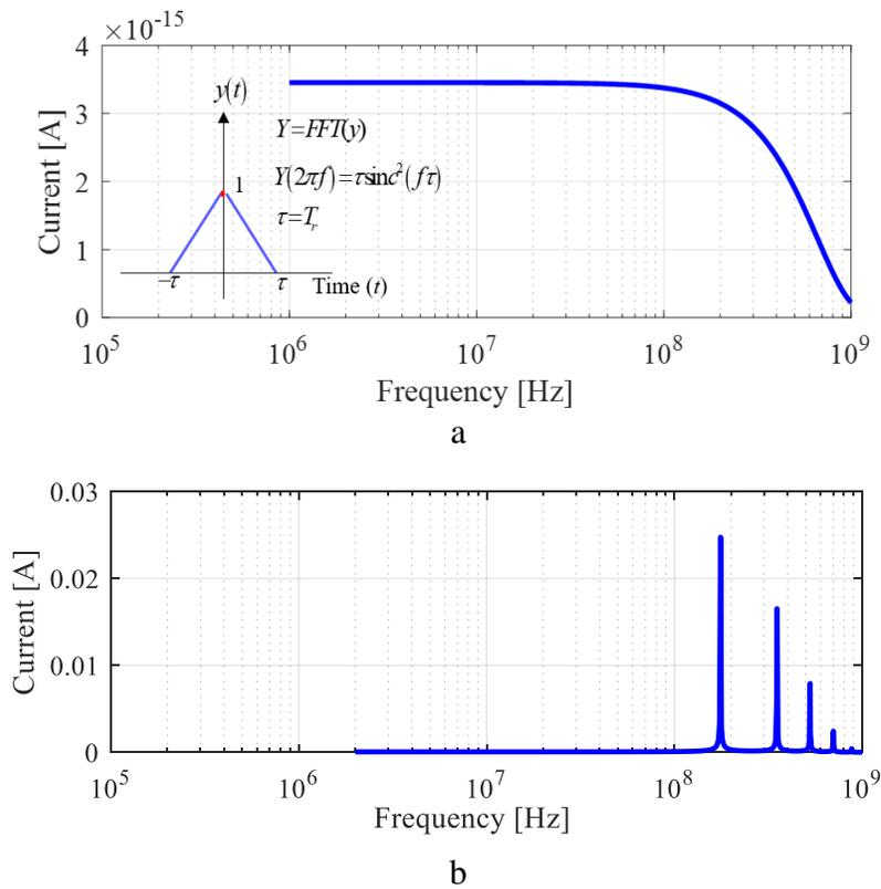
Figure 3.13 IC Current Spectrum. a) Single Current Pulse. b) Periodic Current.
