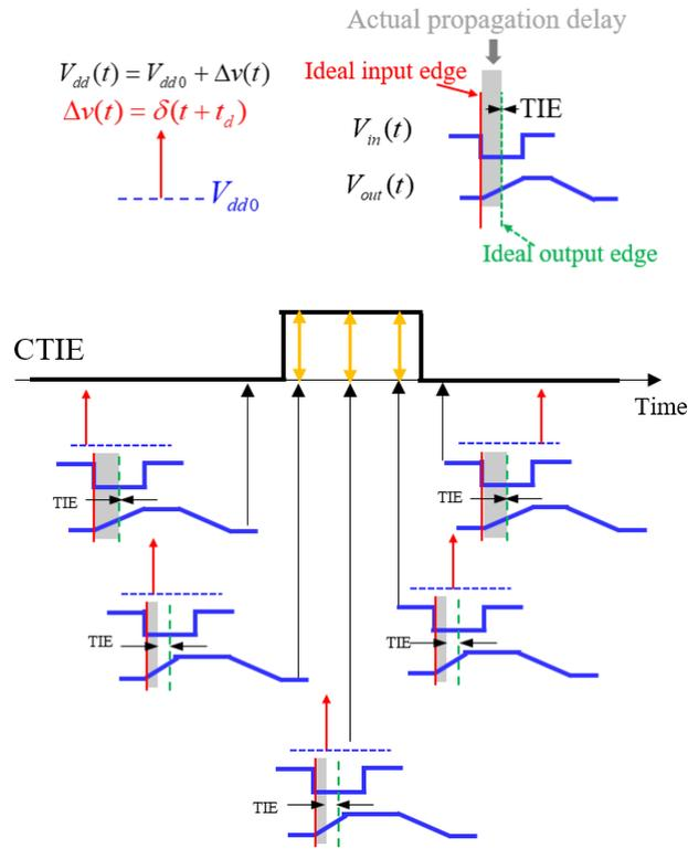
Figure 3.4 Interpretation of Time Domain PSIJ Transfer Relationship as System Impulse Response.
