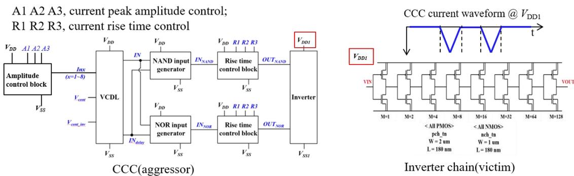
Figure 3.25 Design Block for CCC and Victim Driver.
