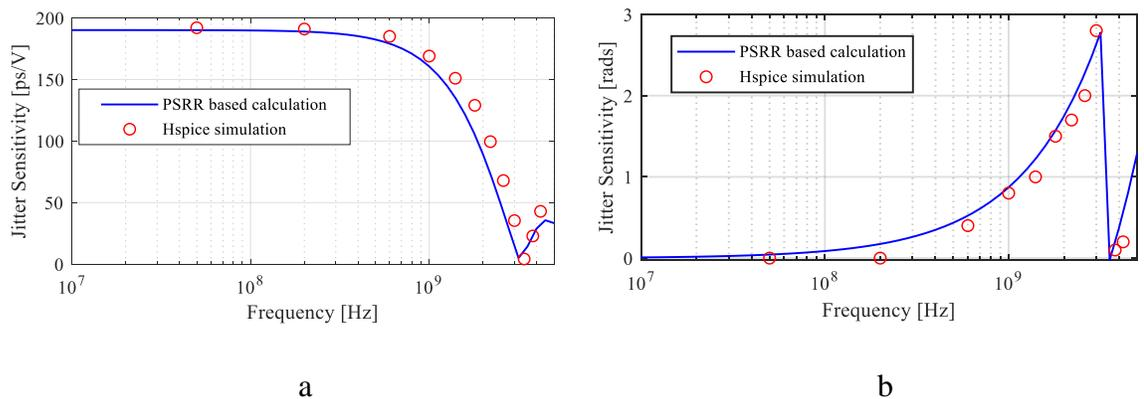
Figure 2.14 Inverter Chain Falling Edge PSIJ Sensitivity Results Comparison between PSRR Based Model and HSPICE Simulation. a) Magnitude. b) Phase.
