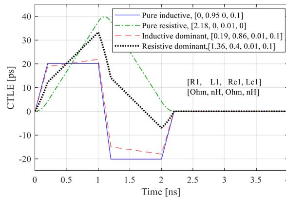
Figure 3.16 CTIE of Four Calculated Cases with the Same Peak-To-Peak Value (40 ps) for Single Stage Inverter.
