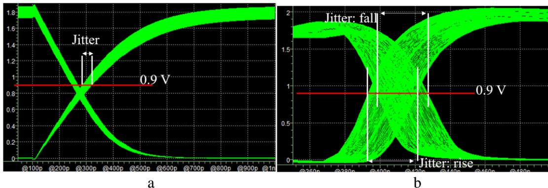
Figure 3.14 Jitter Value Reading Form Simulation. a) Single Stage Buffer, Rising Edge. b) Inverter Chain, Rising and Falling Edge.
