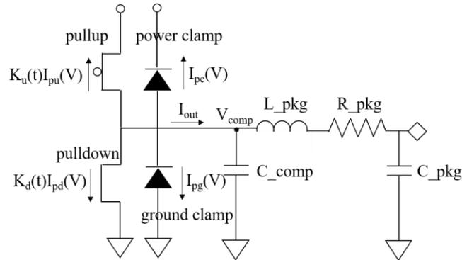
Figure 2.28 IBIS Output Model Structure.
