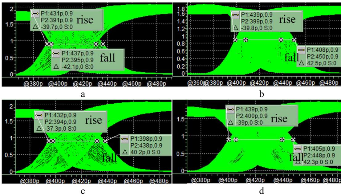
Figure 3.20 Validation of the Predicted Jitter for the Four Cases for Inverter Chain. a) Pure Inductive. b) Pure Resistive. c) Inductive Dominant. d) Resistive Dominant.
