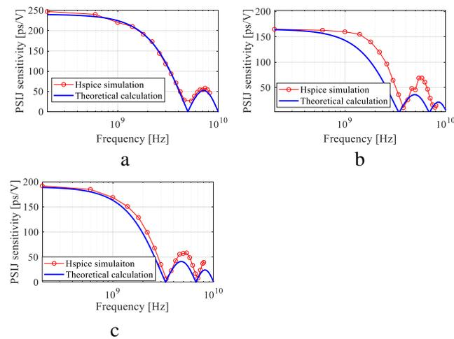
Figure 3.10 PSIJ Transfer Function HSPICE Simulation and Theoretical Calculation Comparison. a) Single Stage Buffer, Rising Edge. b) Inverter Chain, Rising Edge. c) Inverter Chain, Falling Edge.
