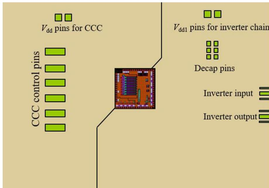
Figure 3.24 Designed PCB for Test IC.
