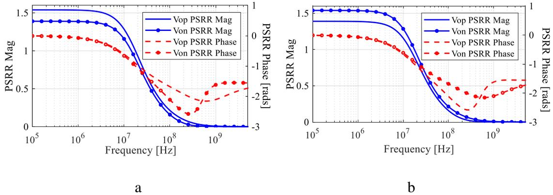
Figure 2.15 PSRR of Differential Driver. a) Positive Input Low, Negative Input High. b) Positive Input High, Negative Input Low.
