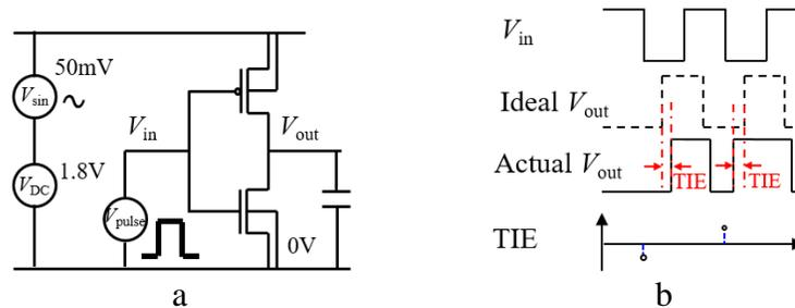
Figure 2.8 Simulation Setup for Jitter Extraction. a) Setup. b) Extraction of TIE Sequence.
