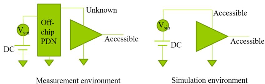
Figure 3.34 Proposed Procedure for Evaluating PSIJ Sensitivity from Off-Chip Environment.
