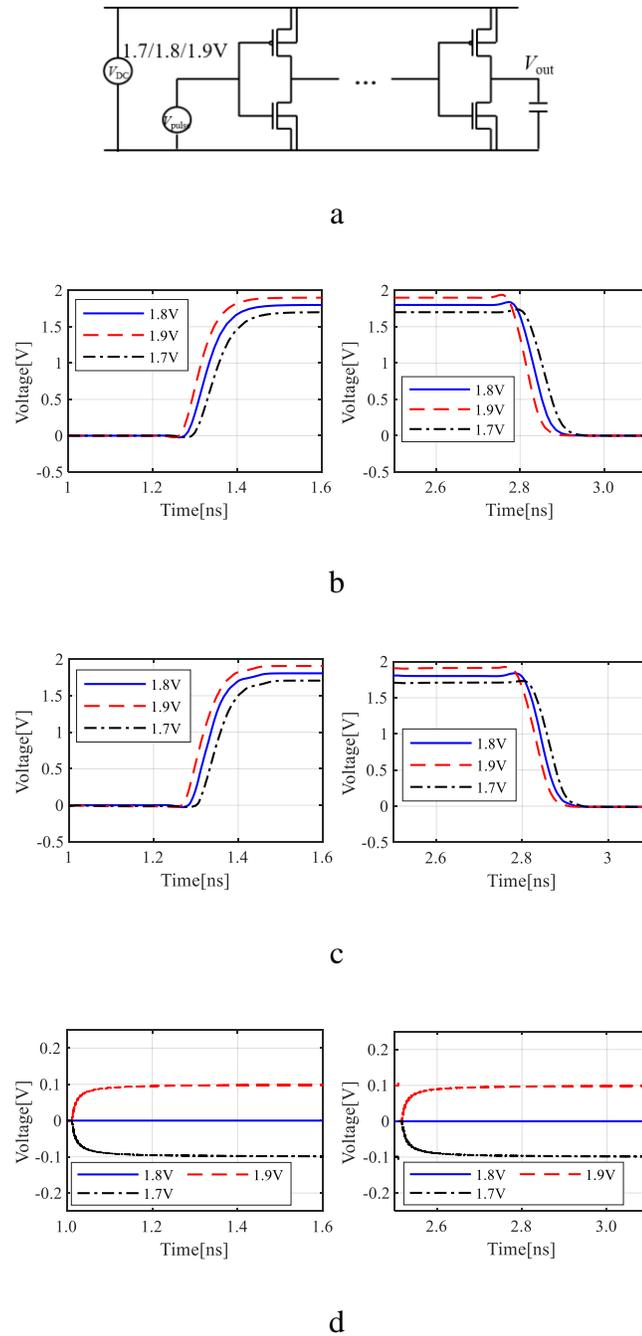
Figure 2.35 Test Case1. a) Simulation Setup. b) HSPICE Output Results. c) Proposed Model Output Results. d) Proposed Model Time Averaged Power Noise Results.
