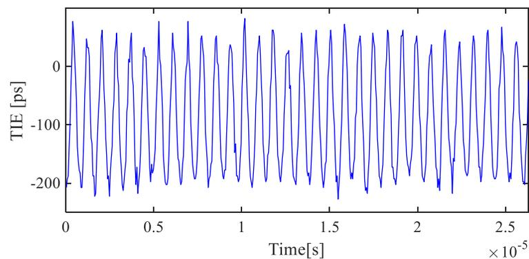
Figure 3.38 Extracted TIE Sequence with 18MHz Noise.
