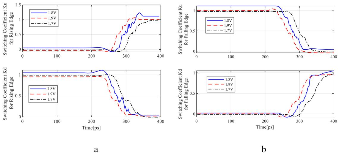
Figure 2.33 Switching Coefficients  $K_u$ ,  $K_d$ . a) Rising Edge. b) Falling Edge.
