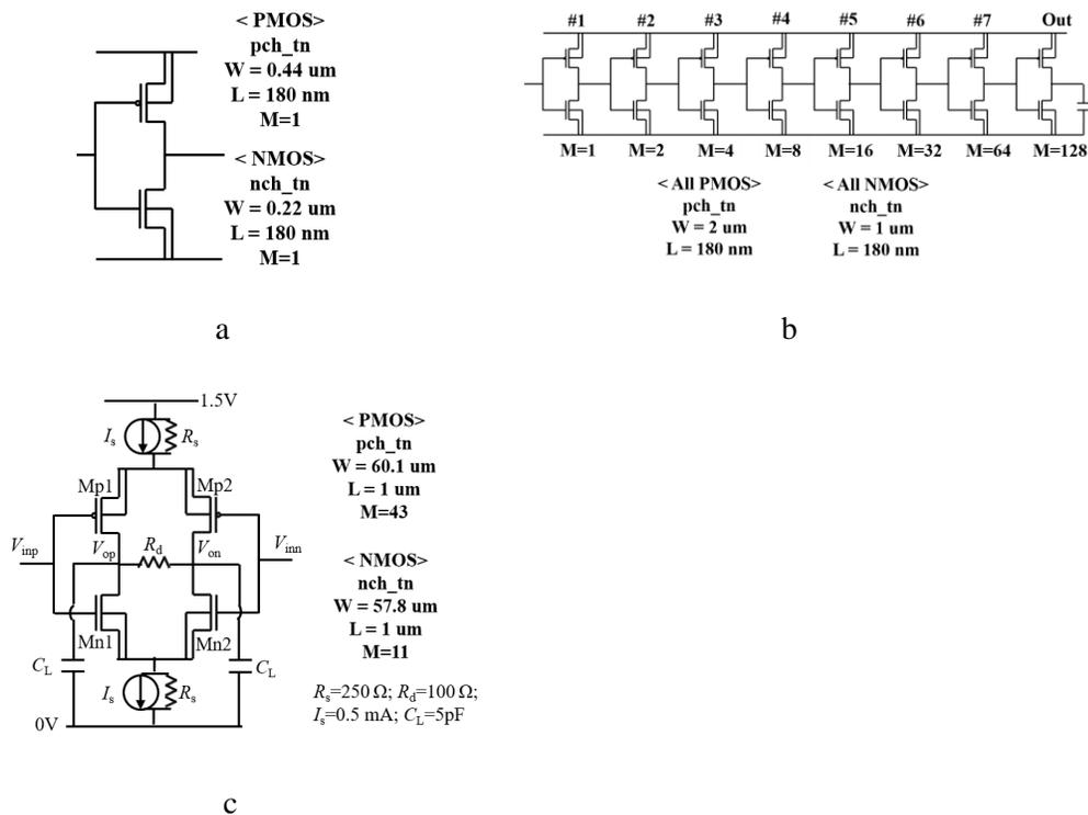
Figure 2.4 Tested Drivers. a) Inverter. b) Inverter Chain. c) Current Mode Differential Driver.
