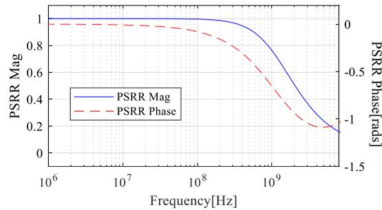
Figure 2.7 PSRR Simulation Result for Single Stage Inverter.
