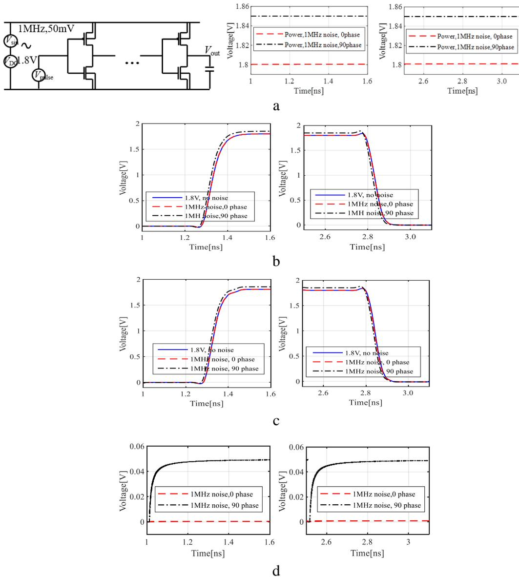
Figure 2.37 Test Case2. a) Simulation Setup. b) Hspice Output Results ;(C) Proposed Model Output Results; (D) Proposed Model Time Averaged Power Noise Results.
