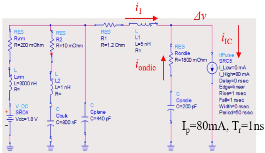
Figure 3.30 ADS Simulation Setup.
