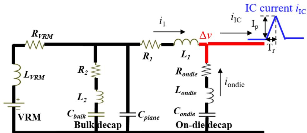
Figure 3.29 Triangular IC Current Passing Through PDN Model.
