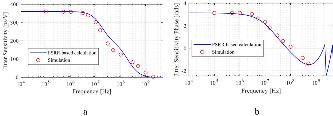
Figure 2.17 Differential Transmitter PSIJ Sensitivity Results Comparison between PSRR Based Model and HSPICE Simulation. a) Differential Output PSIJ Magnitude. b) Differential Output PSIJ Phase.
