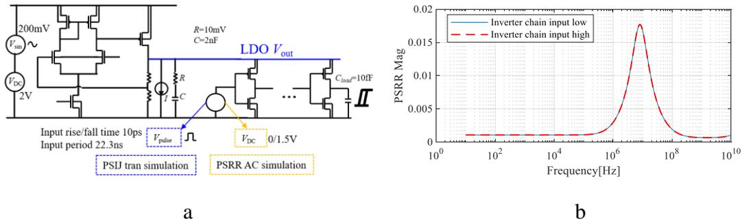
Figure 2.22 PSRR Response of LDO Block with Inverter Chain Buffer. a) Simulation Setup. b) PSRR Response.
