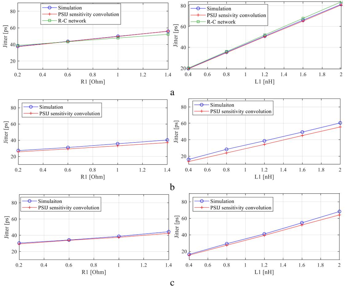
Figure 3.15 Predicted Jitter and HSPICE Simulation Comparison. a) Single Stage Buffer, Rising Edge. b) Inverter Chain, Rising Edge. c) Inverter Chain, Falling Edge.
