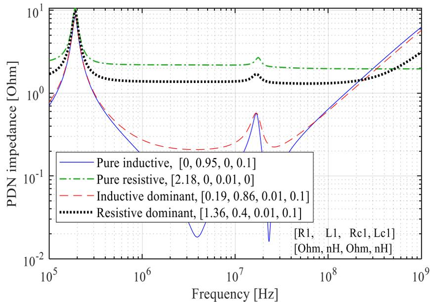
Figure 3.18 Target Impedance Defined Based on Jitter Specification Corresponds to the Four Cases for the Single Stage Buffer.
