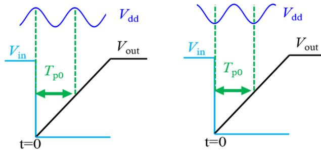
Figure 2.3 Power Noise Time Averaged Effect during Propagation Delay.
