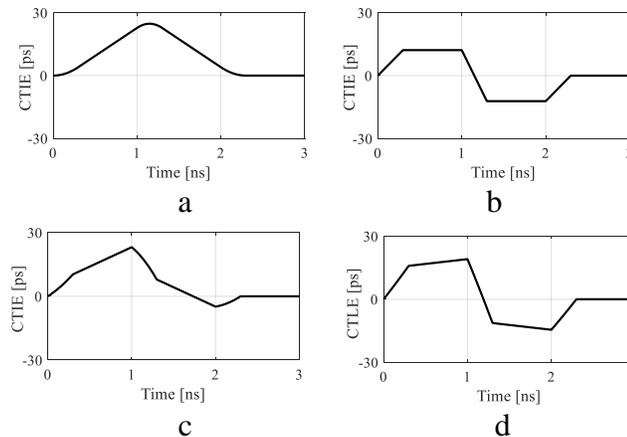
Figure 3.7 CTIE Curve Shape Calculated Using PSIJ Sensitivity Convolution with Different PDN  $R_{PDN}$  and  $L_{PDN}$  Combinations. a) Pure Resistive. b) Pure Inductive. c) Resistive Dominant ( $R_{PDN} > L_{PDN}/T_r$ ). d) Inductive Dominant ( $R_{PDN} < L_{PDN}/T_r$ ).
