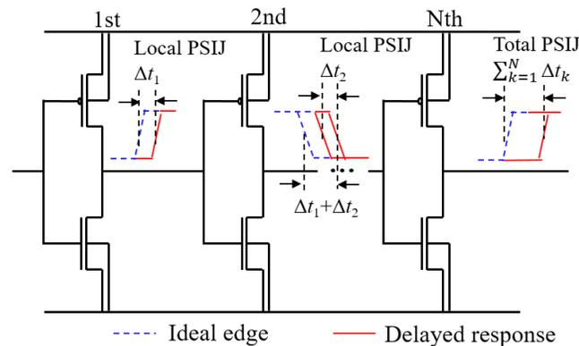
Figure 2.11 Inverter Chain Total PSIJ as Sum of Each Stage Local PSIJ.
