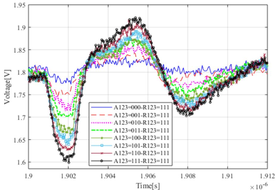
Figure 3.32 Measured On-Die Power Noise under 8 Different Amplitude Control Bits Combinations.
