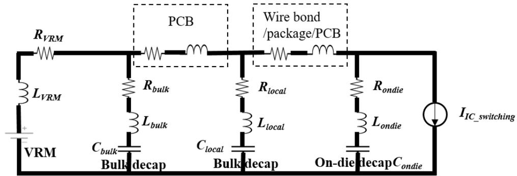
Figure 1.1 A Typical PDN Equivalent Circuit.
