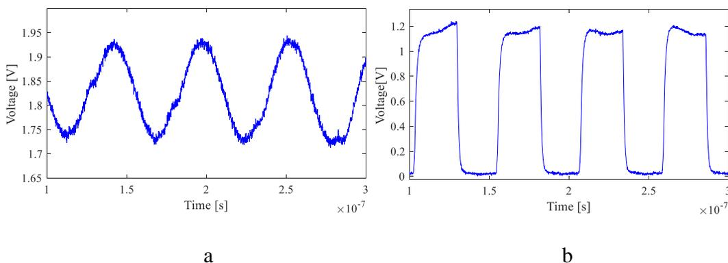
Figure 3.36 Measured Time Domain Waveform. a) On-Die Power Net. b) Output Waveform.
