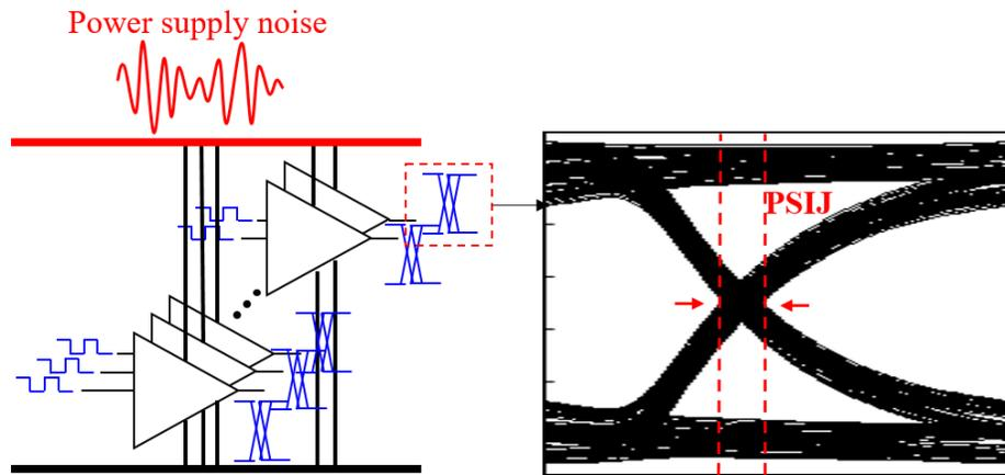
Figure 1.2 PSIJ as a Result of Power Supply Noise.
