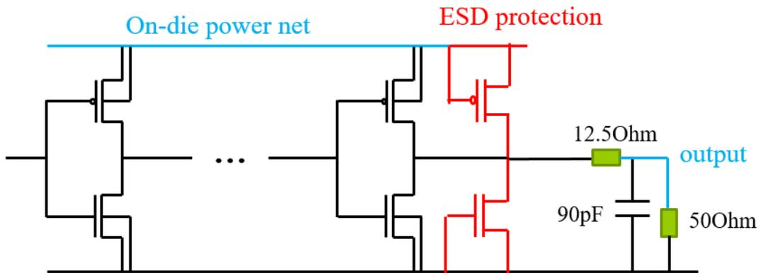
Figure 3.43 Equivalent Simulation Setup.
