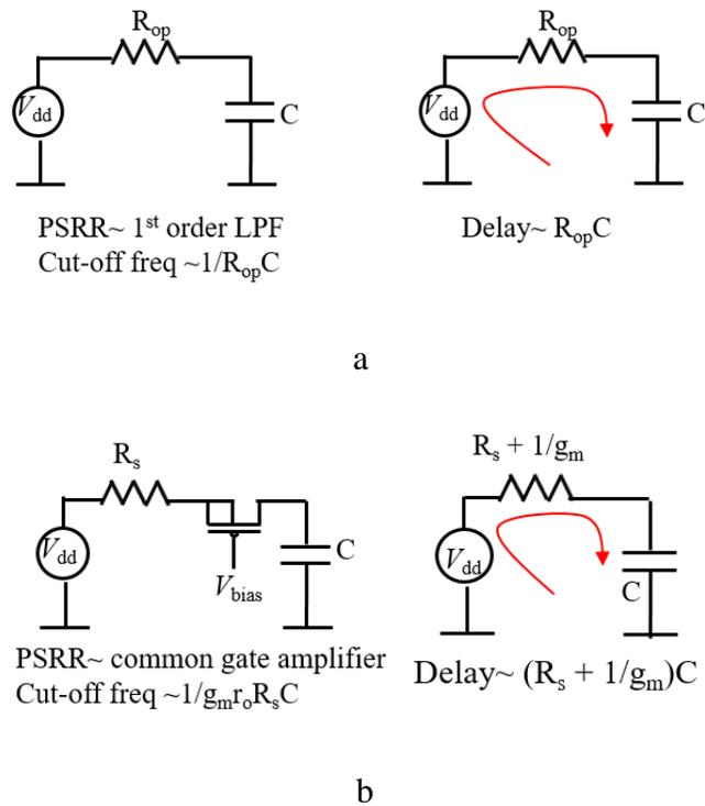
Figure 2.5 Comparison of Frequency Dependency Due to PSRR and Propagation Delay.
