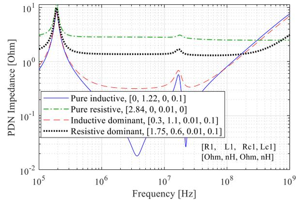
Figure 3.21 Target Impedance Defined Based on Jitter Specification Corresponds to the Four Cases for the Inverter Chain.
