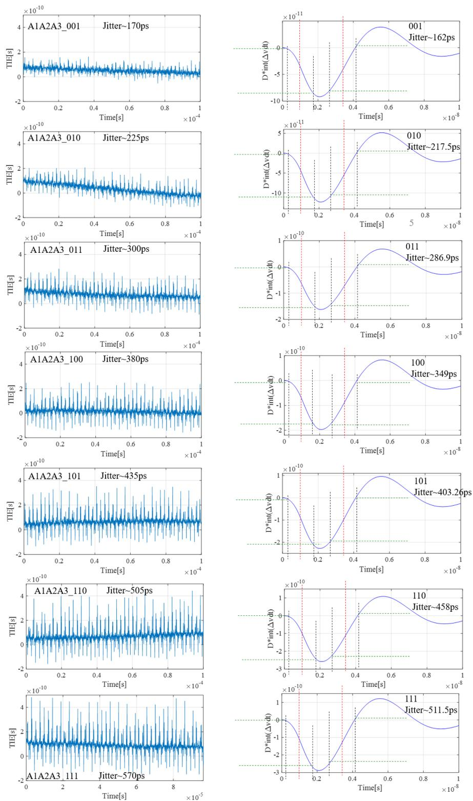
Figure 3.47 Measured and Calculated Jitter for Other Cases.
