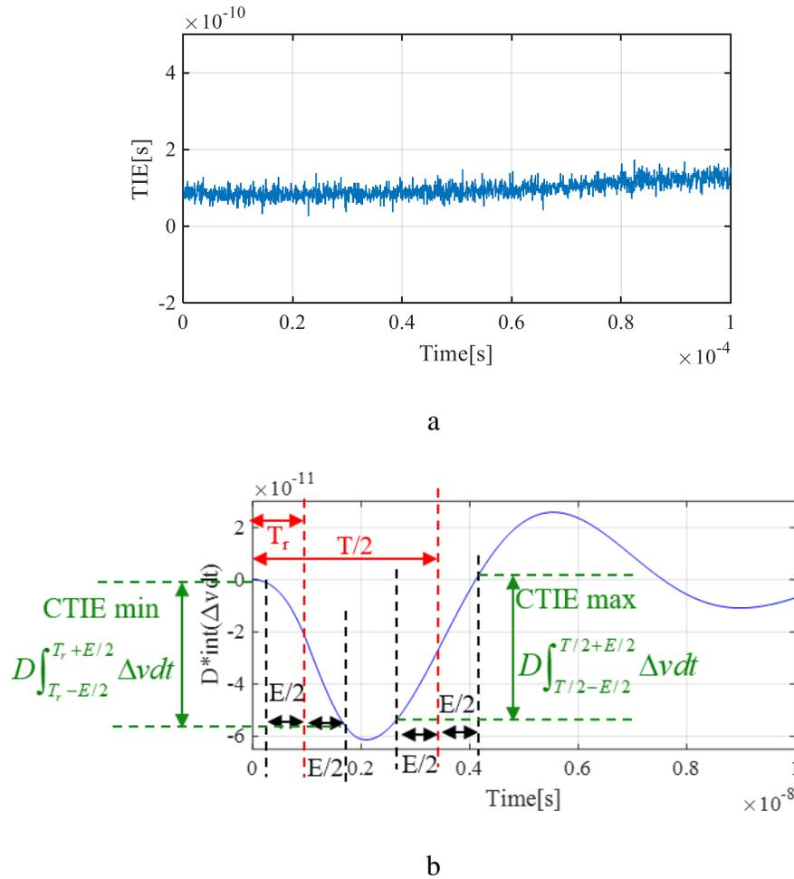
Figure 3.46 Measured and Calculated Jitter for 000 Case. a) Measured TIE. b) Calculated Jitter.
