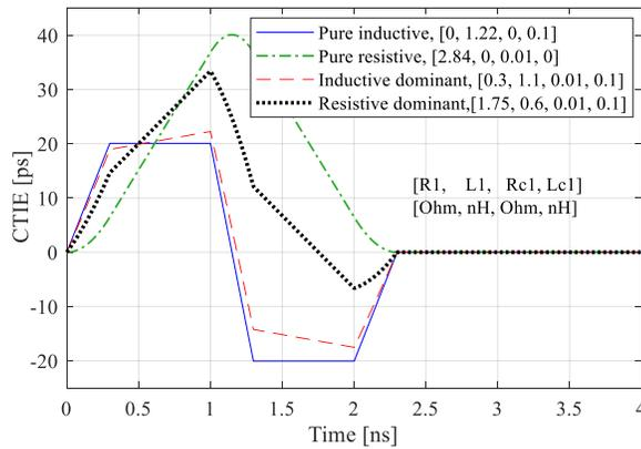
Figure 3.19 CTIE of Four Calculated Cases with the Same Peak-To-Peak Value (40 Ps) for Inverter Chain Falling Edge.
