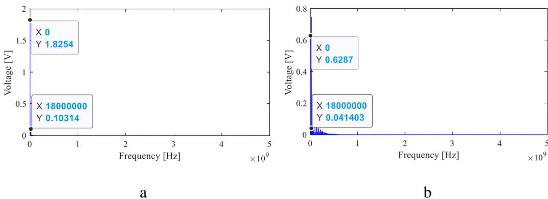
Figure 3.37 FFT of Measured Waveforms. a) On-Die Power Net. b) Output Waveform.
