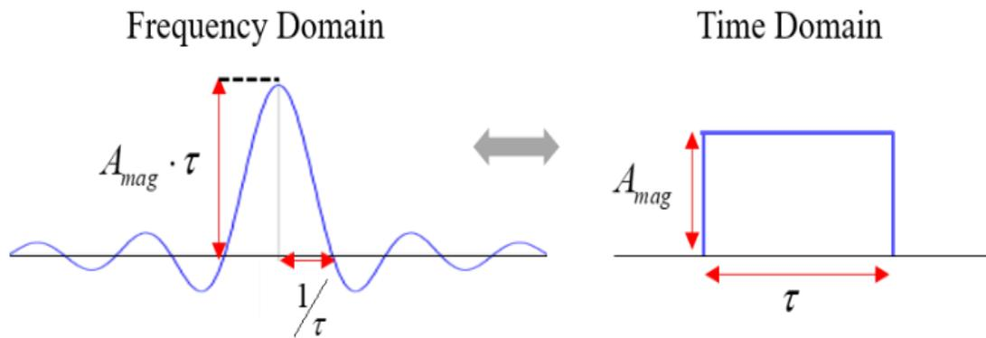
Figure 3.3 Frequency Domain PSIJ Transfer Function vs. Time Domain PSIJ Transfer Relationship.
