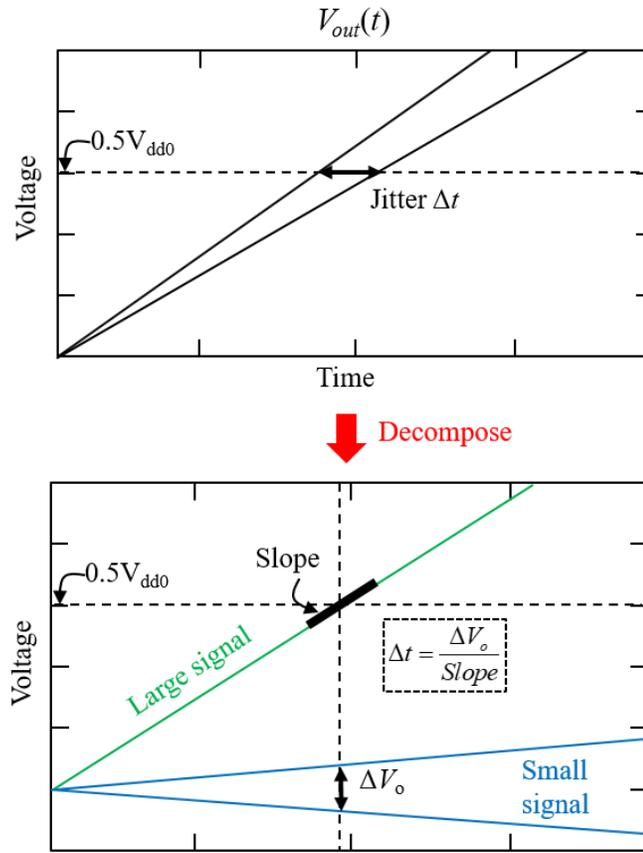
Figure 2.1 Jitter Derivation from Decomposed Multiple Output Voltage Transition Edges.
