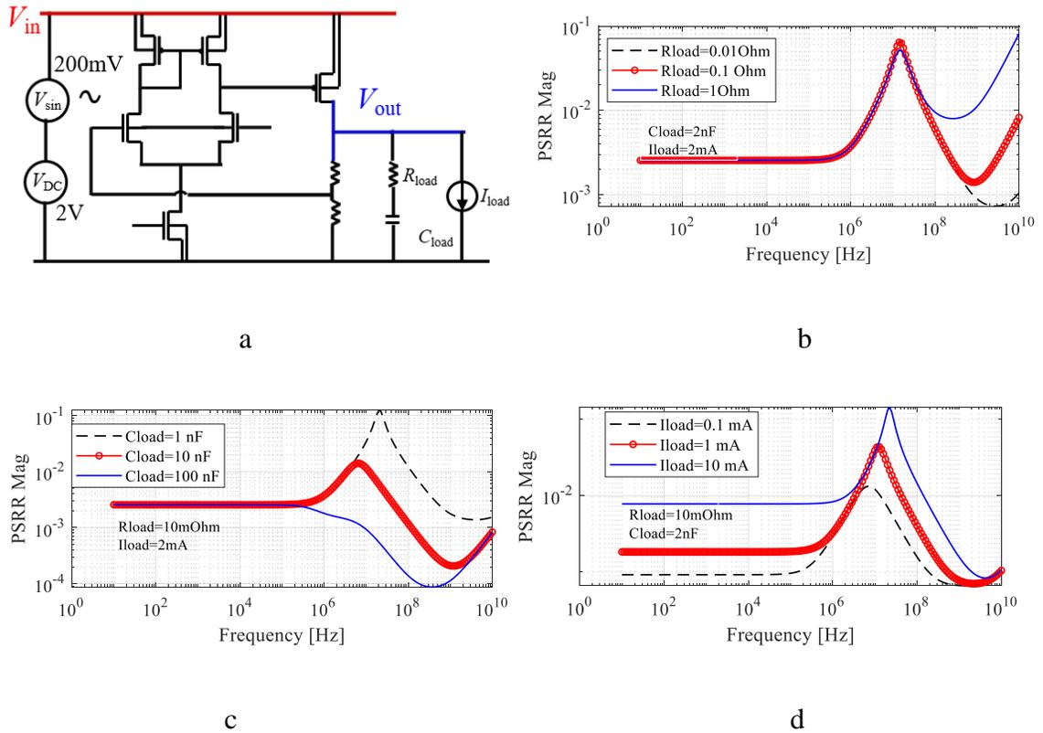
Figure 2.20 Loading Effect to LDO PSRR Response. a) Simulation Setup. b) Load Resistance Effect. c) Load Capacitance Effect. d) Load Current Effect.
