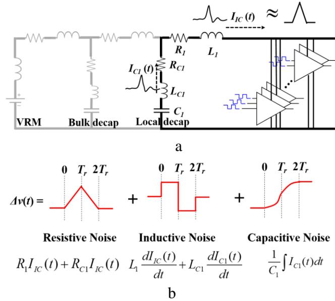
Figure 3.5 PDB Model and Time Domain Voltage Ripple. a) Typical PDN Model with Fast Rise Time Current Pulse. b) Voltage Ripple Components with Fast Rise Time Current Pulse.
