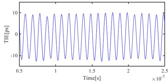
Figure 2.9 Extracted TIE Sequence for the Case with 100 MHz Power Noise.
