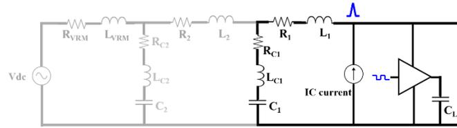
Figure 3.11 Target Impedance with Jitter Specification Validation HSPICE Simulation Setup.
