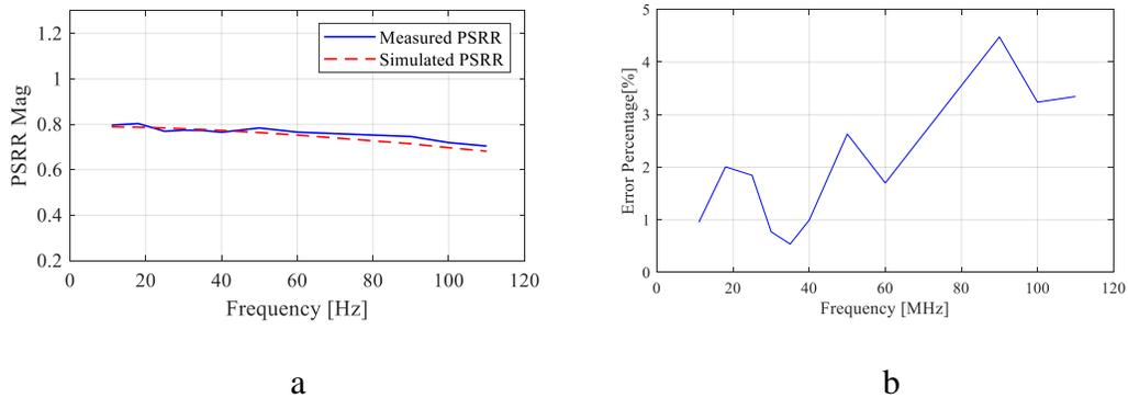
Figure 3.40 PSRR Response. a) Measured and Simulated PSRR Comparison. b) Error Percentage.
