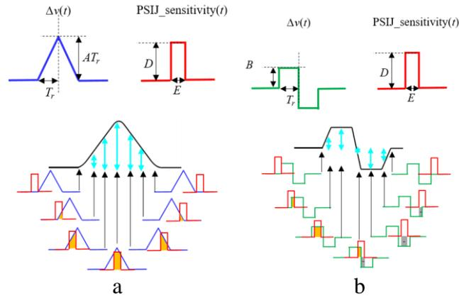
Figure 3.6 Convolution Process Illustration. a) Resistive Noise Convolution. b) Inductive Noise Convolution.
