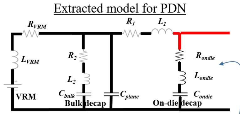
$R_{ondie}=1.8\Omega$ , on die resistance     $L_{ondie}=0$ , on die inductance
