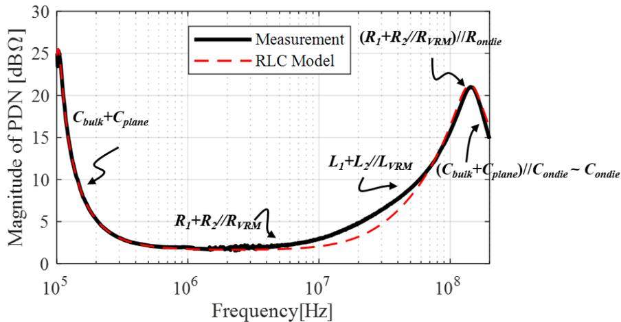
Figure 3.28 Comparison of Measured and Simulated PDN Impedance.
