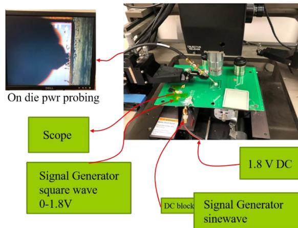
Figure 3.35 Test Board and Measurement Setup.
