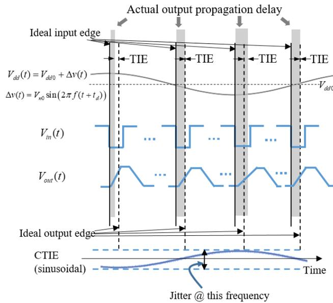
Figure 3.2 Single Tone Power Supply Noise and Resulted CTIE.
