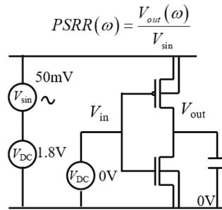
Figure 2.6 PSRR Simulation Test for Single Stage Inverter.
