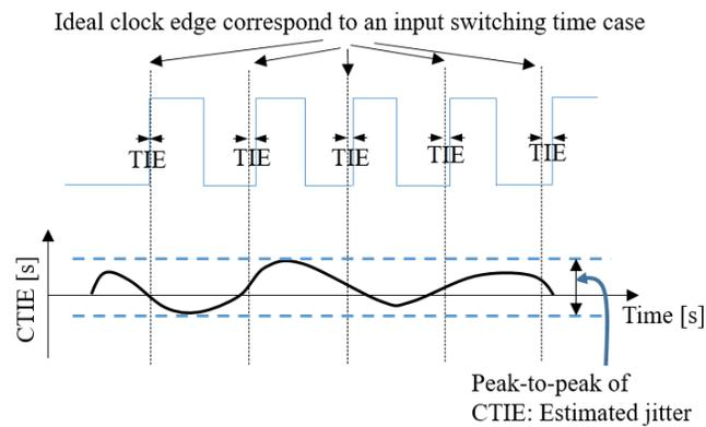
Figure 3.1 CTIE and Jitter Definition.
