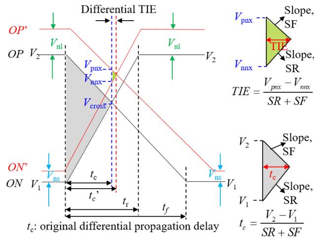
Figure 2.16 Differential Driver Output TIE Analysis Illustration.
