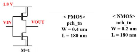
Figure 3.9 Designed Single Stage Buffer for Validation.
