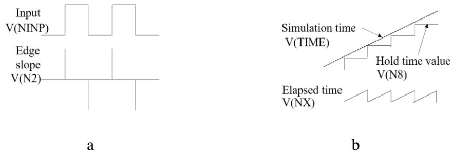
Figure 2.30 Control Signal Calculation. a) Find Switching Edges. b) Obtain Elapsed Time Since Switching Event Happens.
