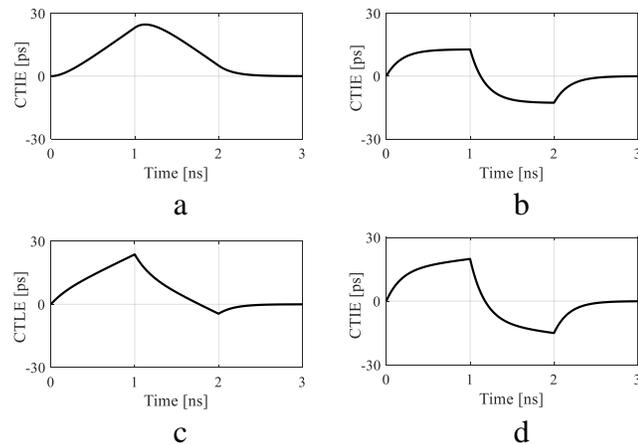
Figure 3.8 CTIE Curve Shape Calculated Using R-C Network Model with Different PDN  $R_{PDN}$  and  $L_{PDN}$  Combinations. a) Pure Resistive. b) Pure Inductive. c) Resistive Dominant ( $R_{PDN} > L_{PDN}/T_r$ ). d) Inductive Dominant ( $R_{PDN} < L_{PDN}/T_r$ ).
