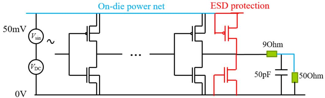
Figure 3.39 Equivalent Simulation Setup for the Real Measurement Case.
