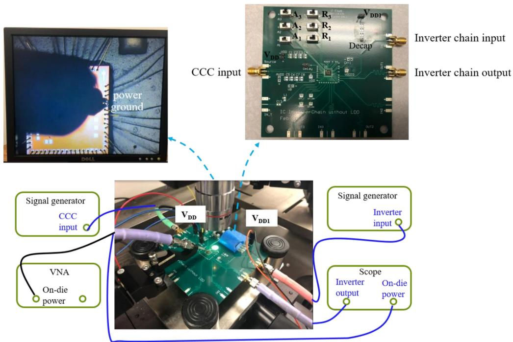
Figure 3.26 Measurement Setup for PSIJ-PDN Correlation Validation.
