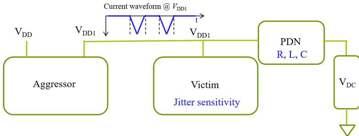
Figure 3.22 PSIJ-PDN Correlation Measurement Procedure.
