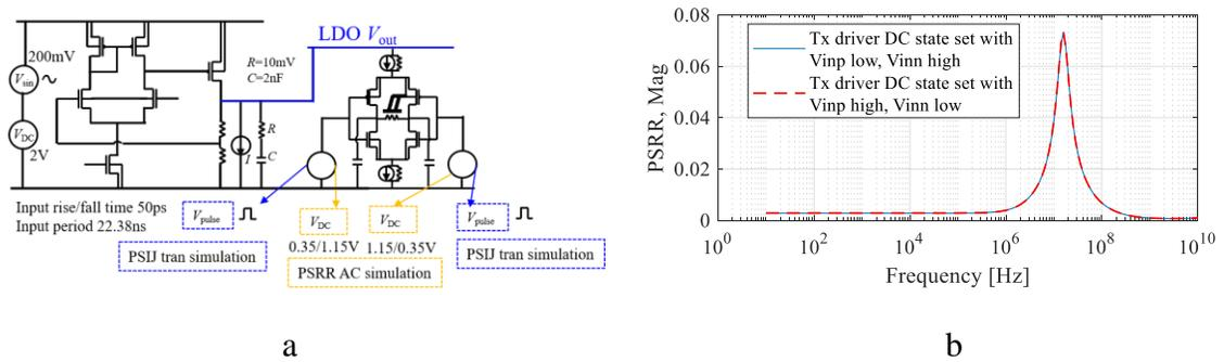
Figure 2.24 PSRR Response of LDO Block with Current Mode Differential Driver. a) Simulation Setup. b) PSRR Response.
