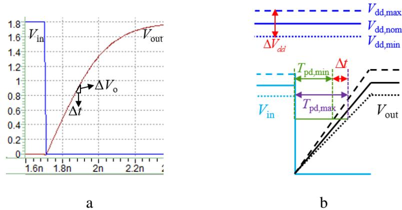
Figure 2.2 Rising Edge Slope Estimation. a) Direct Estimation. b) From DC Delay Change Test.
