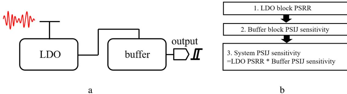
Figure 2.18 System Analysis Method. a) Overall System Block Diagram. b) Proposed Analysis Procedure.
