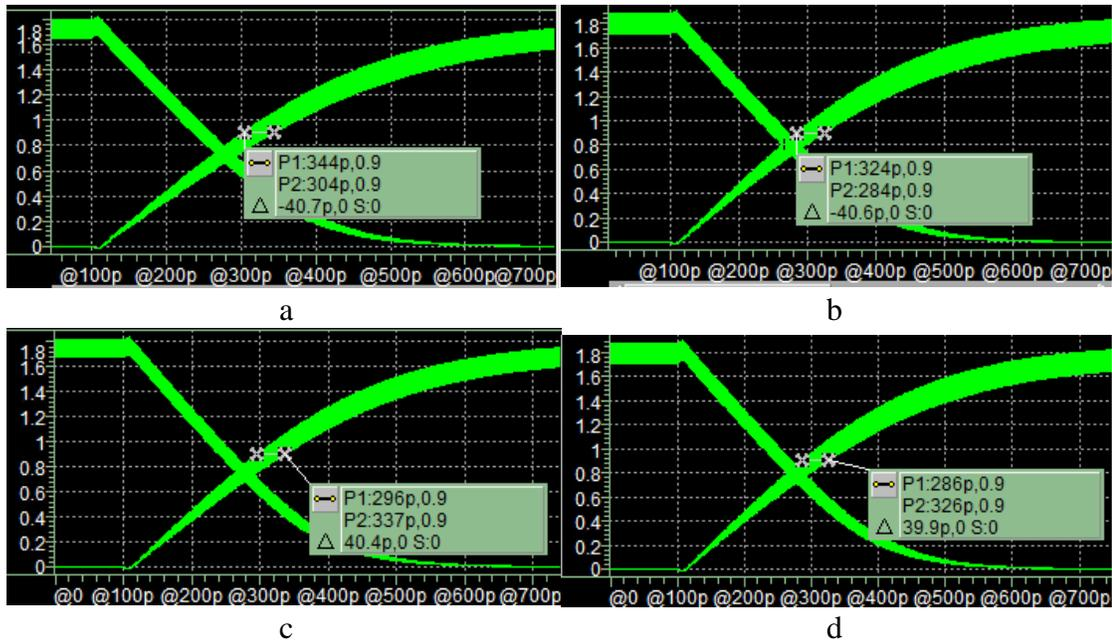
Figure 3.17 Validation of the Predicted Jitter for the Four Cases for Single Stage Inverter. a) Pure Inductive. b) Pure Resistive. c) Inductive Dominant. d) Resistive Dominant.
