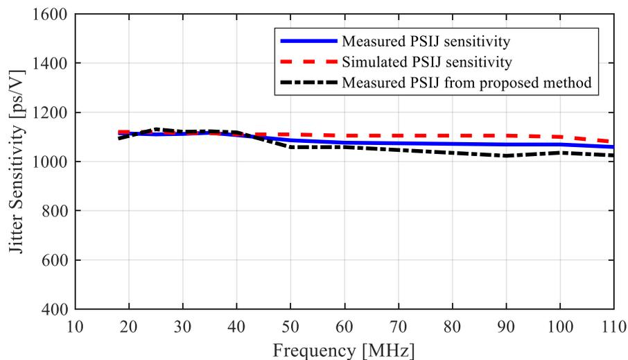
Figure 3.41 PSIJ Sensitivity Comparison between Measured Using On-Die Power Net Noise, Simulation and Proposed Method.
