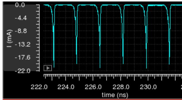
Figure 2.21 Current Drawn on Power Net for Inverter Chain Driver.
