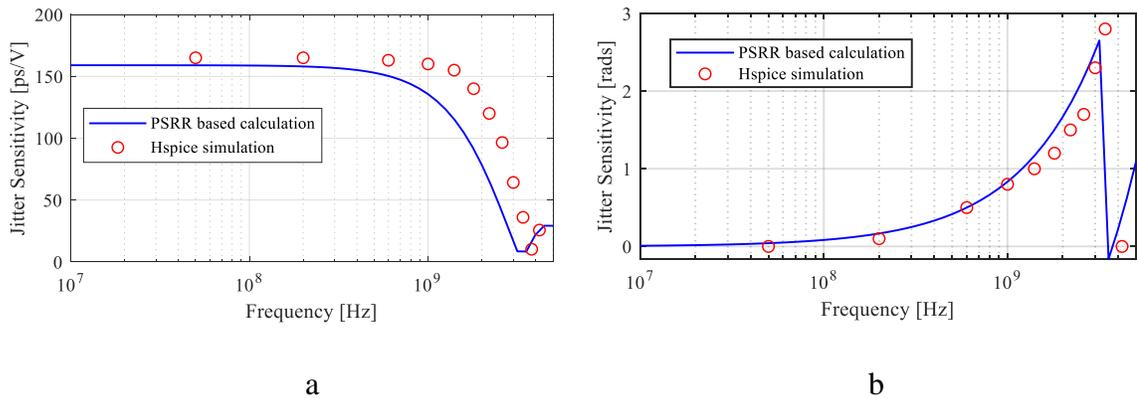
Figure 2.13 Inverter Chain Rising Edge PSIJ Sensitivity Results Comparison between PSRR Based Model and HSPICE Simulation. a) Magnitude. b) Phase.
