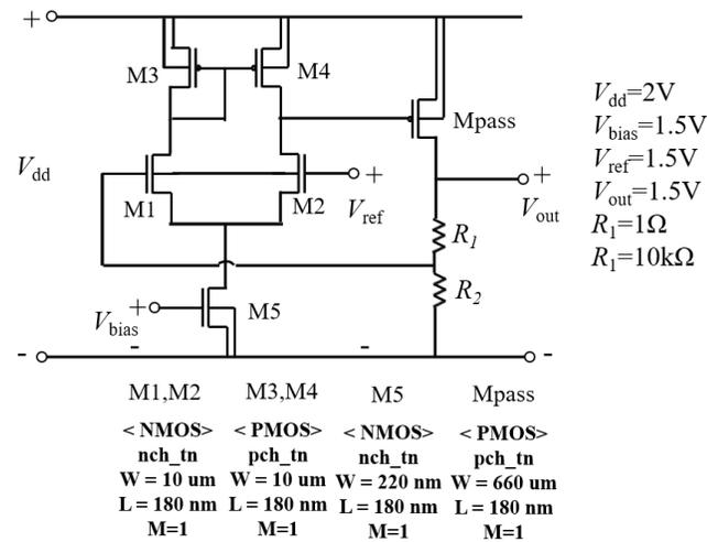
Figure 2.19 Designed LDO Parameters.
