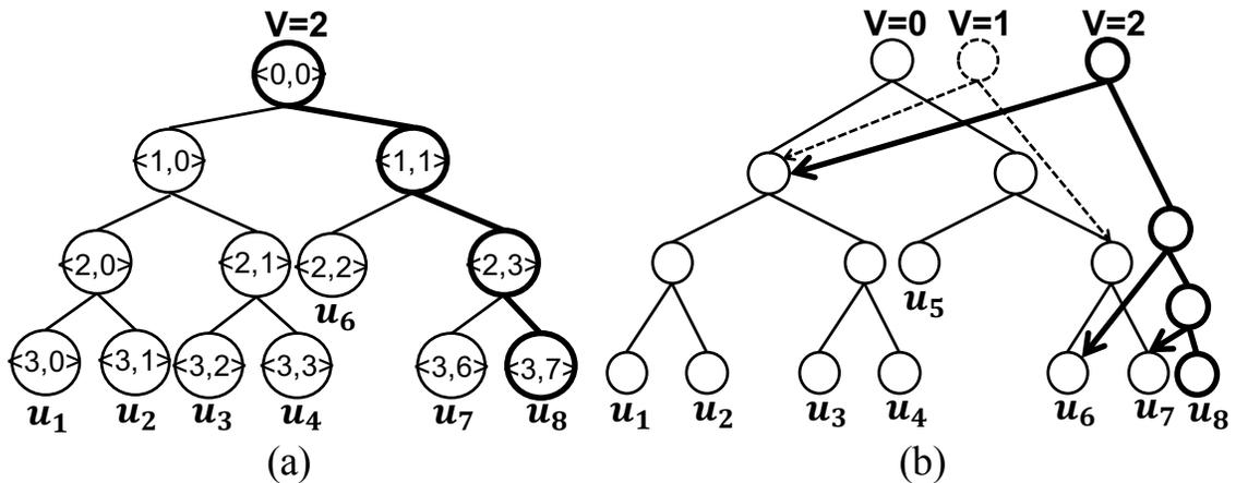
Figure 4. Group admin and cloud's view of the TGDH and e-TGDH tree respectively after adding user  $u_8$  in the group
