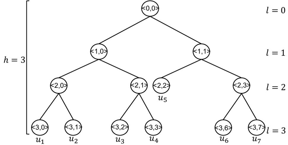
Figure 1. A TGDH Key Tree of height 3 consisting of seven members
