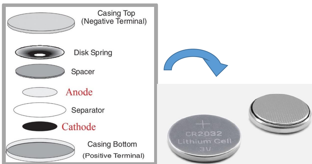
Figure 1.7. Coin cell structure.
