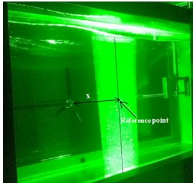
Figure 8. Centered laser sheet at distance x behind the rotor
