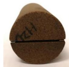
(b) The model before filling sand in the fracture space.
