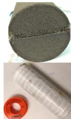
(d) Model is assembled. Gaps between strips and fracture faces are sealed with epoxy to prevent gels migrating along the gaps.
