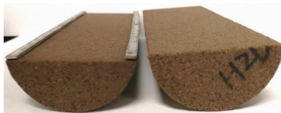
(a) An intact core plug is cut into two halves. A pair of supporting strips are placed to ensure a fracture space between the half plugs.
