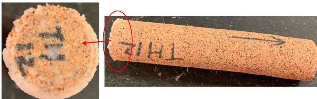
Figure 9. Gel cake formed at the inlet surface of an intact core (Exp #11, 693 md, MSR=20.46). (Due to the large gel particle sizes relative to the pore throats in the core, a high threshold penetration pressure, larger than 1200 psi, was required to drive the gel particles to invade the core. The gel particles accumulated at the inlet surface, and a gel cake was gradually formed. The gel cake further prevented the gel particles from entering the core.)
