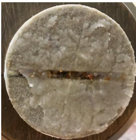
Figure 8. Surface cake at the inlet face.
