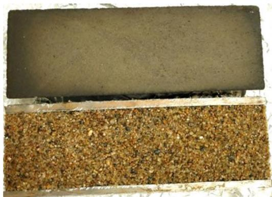
(c) Sand is filled into the fracture space. The sand should be tightly packed to avoid movement and repacking during flooding and gel injection process.
