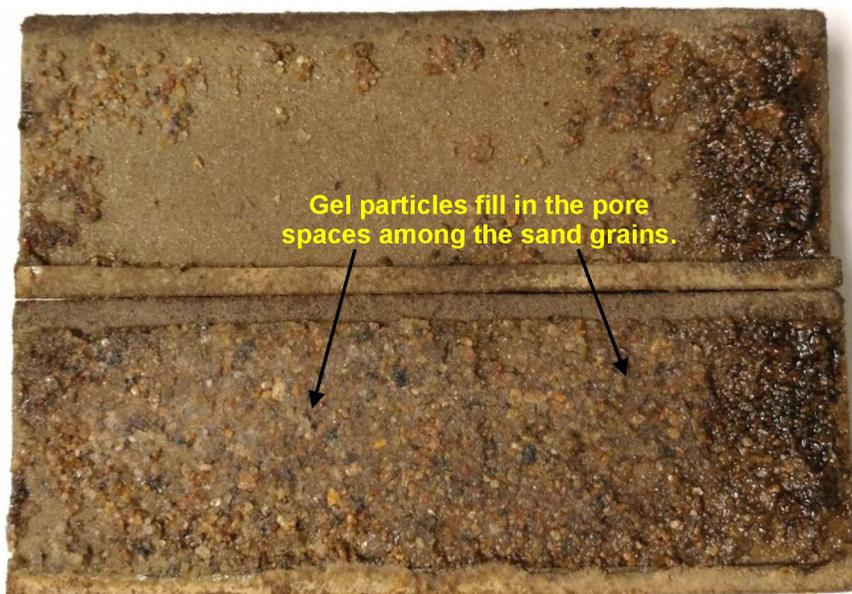
Figure 13. Gel placement in the channel (sand size=10/20 mesh).
