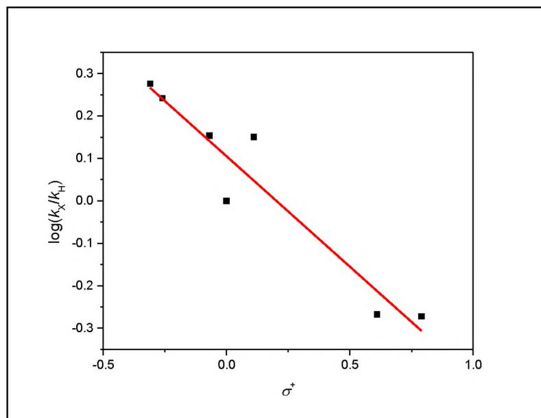
Figure S6. Linear free energy correlation of  $\log(k_X/k_H)$  vs.  $\sigma^+$  for aziridination of para-substituted styrenes by  $[L^8M^{II}\text{-solv}]^-$  (M = Mn (top) or Co (bottom)). Fe provides a poor correlation.
