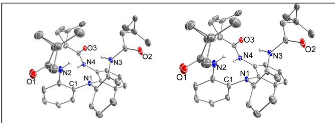
Figure S1. ORTEP diagrams of ligands  $L^{16}H_3$  (left) and  $L^{17}H_3$  (right), drawn with 40% thermal ellipsoids. Selective interatomic distances ( $\text{\AA}$ ) and angles ( $^\circ$ ).
