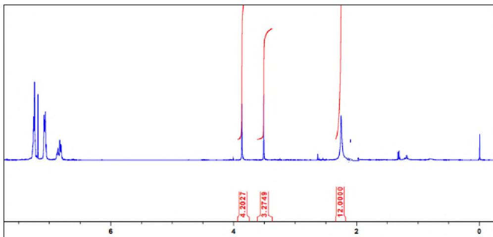
Figure 5. <sup>1</sup>H NMR of DMDPI<sub>3</sub>- biphen Ligand **11** in CDCl<sub>3</sub>
