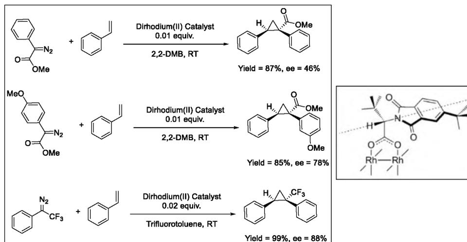
Scheme 13. Chiral Dirhodium(II) Carboxylate Catalyzed Asymmetric Cyclopropanation Reaction
