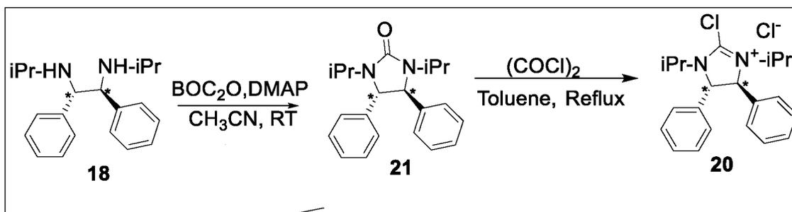
Scheme S16. Synthesis of N-isopropyl imidazolium chloro salt (Method B).
