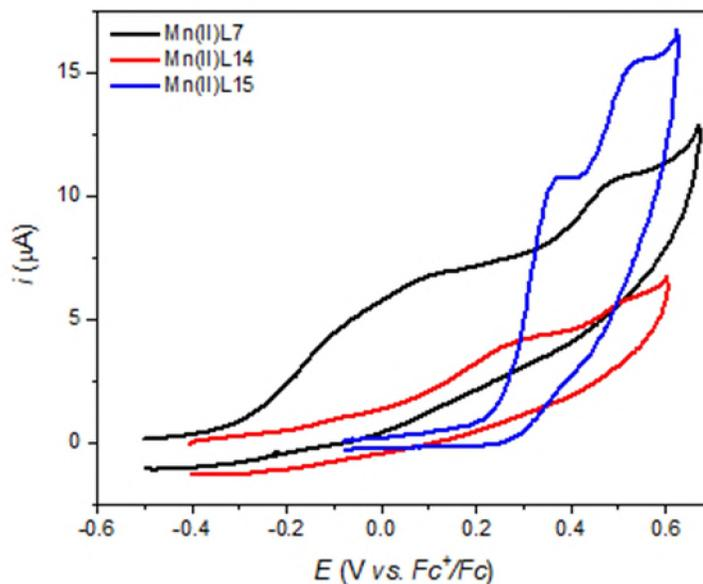
Figure S5. Cyclic voltammograms of  $\text{Mn}^{\text{II}}$  compounds bearing acyl-ligands:
