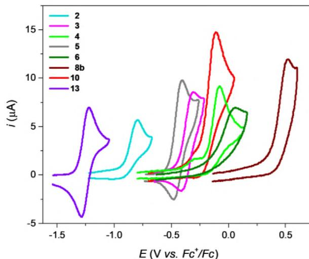
Figure 7. Cyclic voltammograms (first oxidation wave) of selected Mn<sup>II</sup> compounds:
