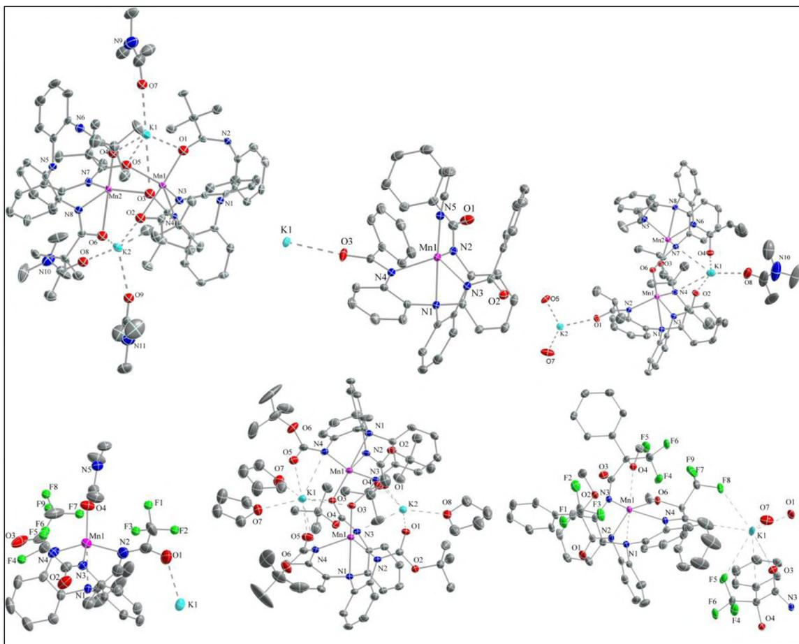
Figure 4. ORTEP Diagrams of  $Mn^{II}$  Compounds **4**, **6**, **7**, **8a**, **10**, and **15**, Bearing Acyl Arms. Drawn with 40% thermal ellipsoids. Selective interatomic distances [ $\text{\AA}$ ] and angles [ $^\circ$ ]
