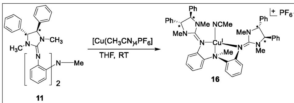
Scheme S11. Synthesis of  $[\text{Cu}^{\text{I}}(\text{DMDPI}_3\text{-biphen})][\text{PF}_6]$ .  $\text{Et}_2\text{O}$ .
