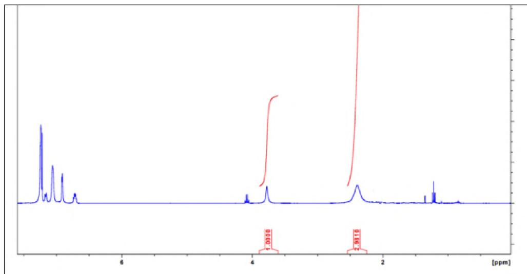
Figure 4. <sup>1</sup>H NMR of DMDPI<sub>3</sub>-trphen Ligand **4** in CDCl<sub>3</sub>
