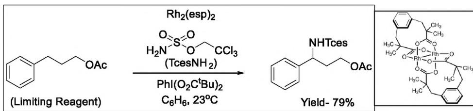
Scheme 5. C—H Amination Using  $\text{Rh}_2(\text{esp})_2$  and  $\text{TcesNH}_2$
