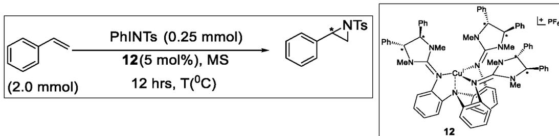
Scheme 24. Asymmetric Aziridination Reaction with  $[\text{Cu}^{\text{I}}(\text{DMDPI}_3\text{-trphen})][\text{PF}_6]$  (**12**)
