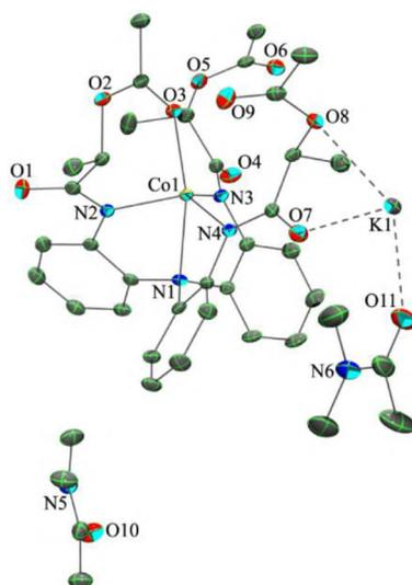
Figure S4. ORTEP Diagram of Compound  $[K(DMA)(L^{14})Co^{II}] \cdot DMA$  (**14c**; drawn with 40% thermal ellipsoids). Selective interatomic distances [ $\text{\AA}$ ] and angles [ $^\circ$ ].
