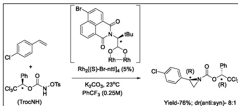
Scheme 4. Stereoselective Intermolecular Aziridination in the Presence of a Chiral Rhodium Catalyst
