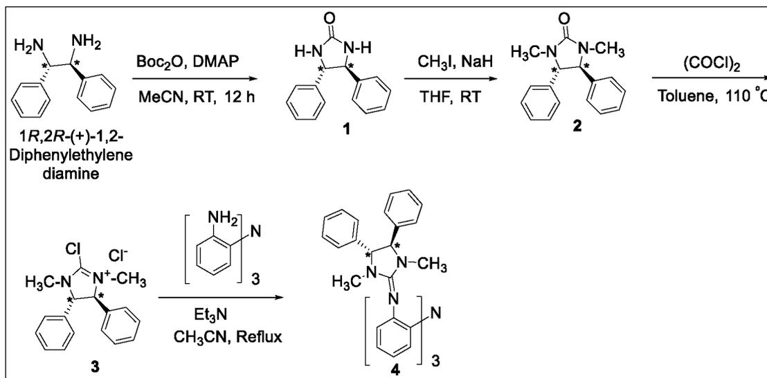
Scheme 15. Synthesis of DMDPI<sub>3</sub>-triphen- Ligand **4**
