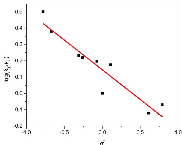
Figure S6. Linear free energy correlation of  $\log(k_X/k_H)$  vs.  $\sigma^+$  for aziridination of para-substituted styrenes by  $[L^8M^{II}\text{-solv}]^-$  (M = Mn (top) or Co (bottom)). Fe provides a poor correlation.(cont.)
