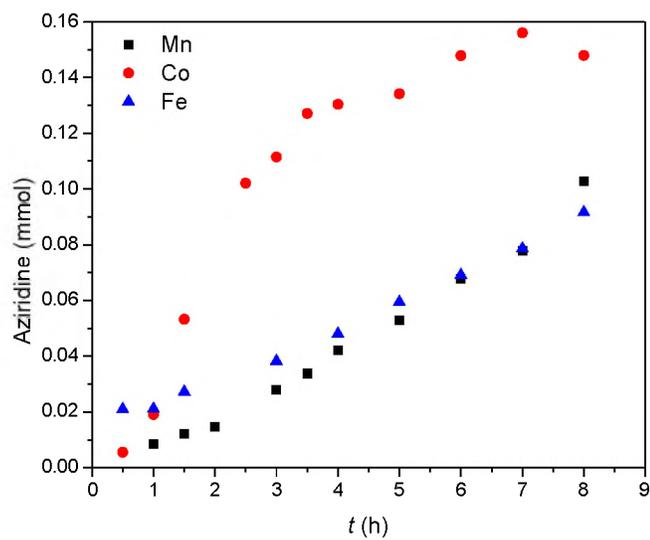
Figure 9. Production of Aziridine as a Function of Time. Reaction of Styrene (2.0 mmol) by  $\text{PhiI=NTs}$  (0.25 mmol) Catalyzed by  $[\text{K}(\text{NCMe})(\text{L}^8)\text{M}^{\text{II}}-\text{NCMe}]$  ( $\text{M} = \text{Mn}, \text{Fe}, \text{Co}$ ; 0.0125 mmol) in  $d_5$ -chlorobenzene (0.50 mL) at 30 °C.
