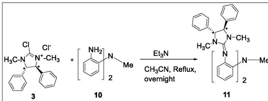
The chloro salt **3** (3 equiv.) noted above, is then coupled with our parent *N*-methyl-2,2'-diamino-diphenylamine **10** in the presence of 2 equiv. of triethylamine in acetonitrile under reflux to afford the bipodal chiral ligand, (4*R*,5*R*)-1,3-bis(methyl)-4,5-diphenylimidazolidin-2-imine- biphen (DMDPI<sub>3</sub>-biphen, 75%) (**11**), featuring the same chiral cyclic guanidinyll residue as the one used in the tripodal analog (Scheme 18).
