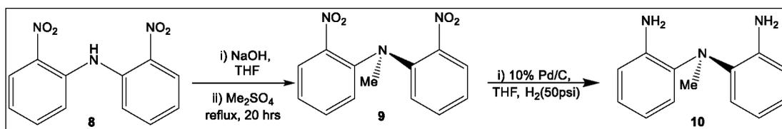
Scheme 17. Synthesis of *N*-methyl-2,2'-diamino-diphenylamine **10**
