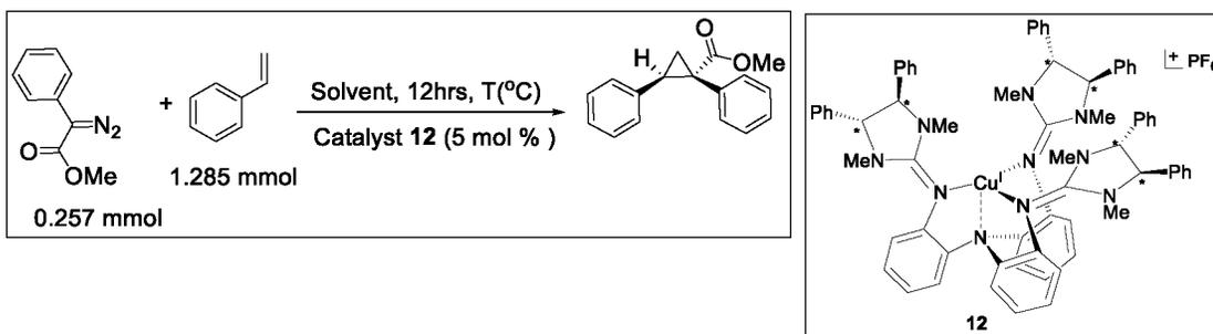
Scheme 27. Asymmetric Cyclopropanation Reaction of Styrene Mediated by Catalyst **12**
