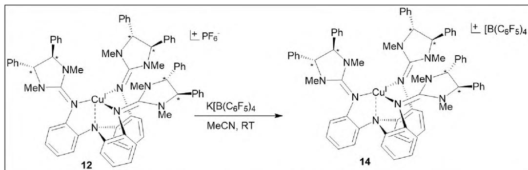
Scheme S9. Synthesis of [Cu<sup>I</sup>(DMDPI<sub>3</sub>-trphen)][(B(C<sub>6</sub>F<sub>5</sub>)<sub>4</sub>)].
