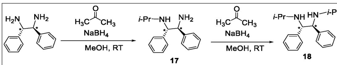
Scheme 28. Synthesis of (1*R*,2*R*)-*N,N'*-Diisopropyl 1,2-diphenylethylenediamine **18**
