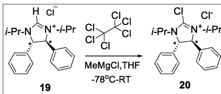
Scheme S15. Synthesis of N-isoprpyl imidazolium chloro salt.
