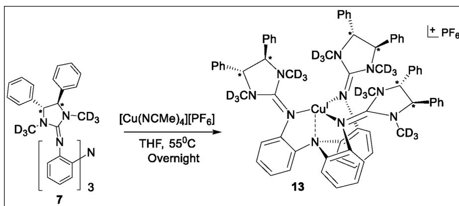
Scheme S8. Synthesis of  $[\text{Cu}^{\text{I}}(\text{d-DMDPI}_3\text{-trphen})][\text{PF}_6]$ .
