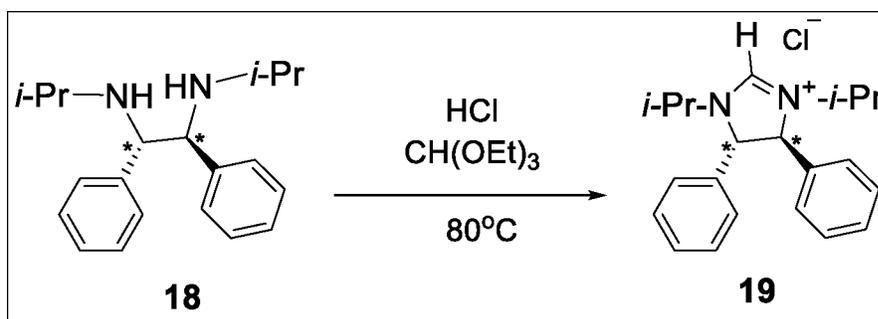
Scheme S14. Synthesis of N-isopropyl imidazolium salt.
