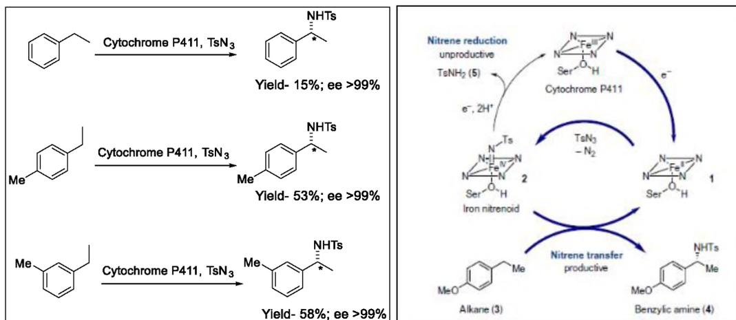
Scheme 8. P411 Catalyzed Enantioselective Amination and Proposed Mechanism of Nitrene Transfer
