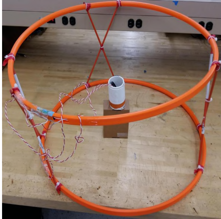
Figure 4. Validation of the receiving coil probe factor using a Helmholtz coil.
