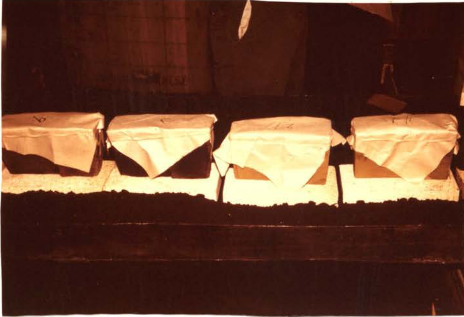
A. Molds placed on firebricks and covered for protection. Next green sand was heaped up around the molds.
