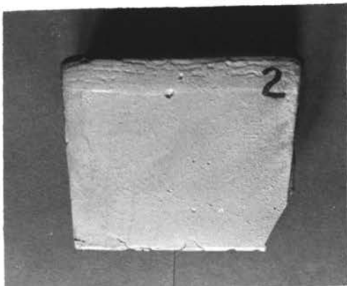
E. Casting #2 30% Magnetite (+200)
