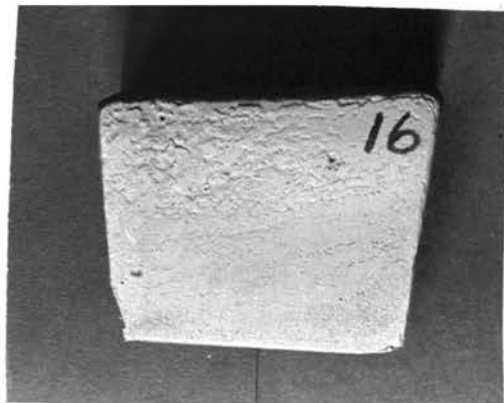
B. Casting #16 10% Magnetite (+200)
