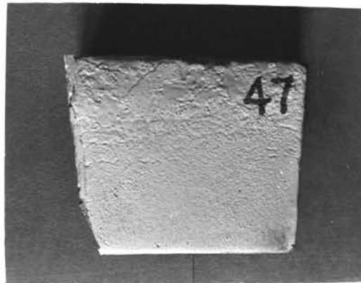
C. Casting #47 20% Magnetite (+100)
