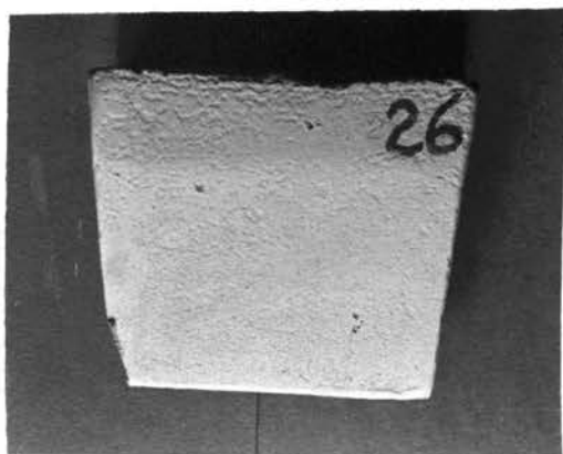
B. Casting #26 10% Magnetite (+150)
