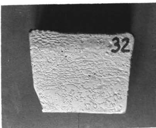
E. Casting #32 50% Magnetite (+325)
