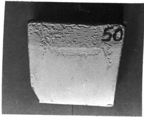
B. Casting #50 Zircon Sand
