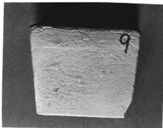
A. Casting #9 10% Magnetite (-325)
