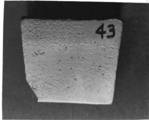
G. Casting #43 40% Magnetite (+100)
