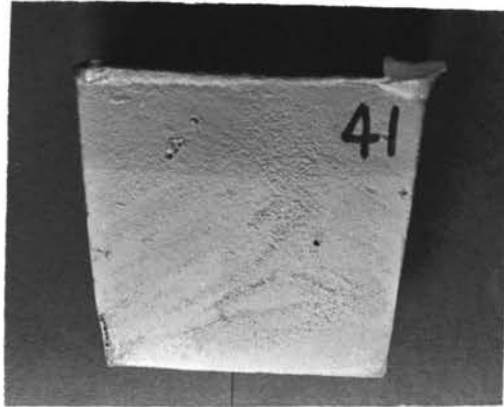
A. Casting #41 (Right Side) Silica Sand 30% Magnetite (+200)
