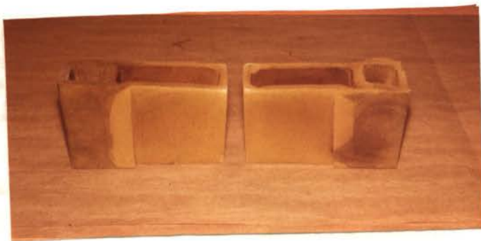
C. Composite molds made with aluminum pattern.
