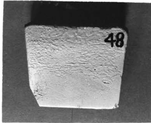
H. Casting #48 40% Magnetite (+200)
