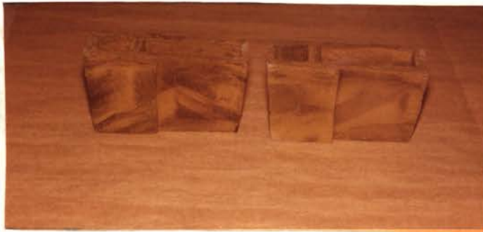
B. Segregation of magnetite in molds containing 50% +65 mesh magnetite (left) and 50% +100 mesh magnetite (right).
