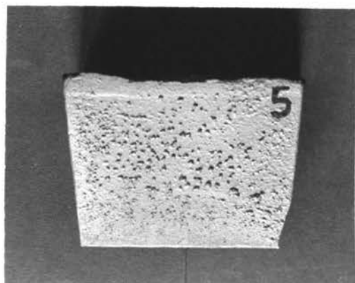
D. Casting #5 50% Magnetite (+65)
