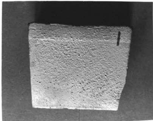
D. Casting #1 30% Magnetite (+100)
