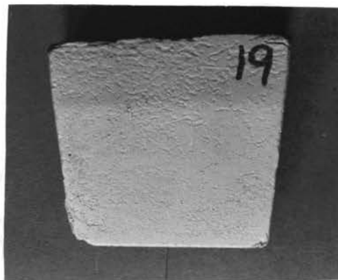
B. Casting #19 10% Magnetite (-325)
