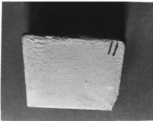
A. Casting #11 10% Magnetite (+200)
