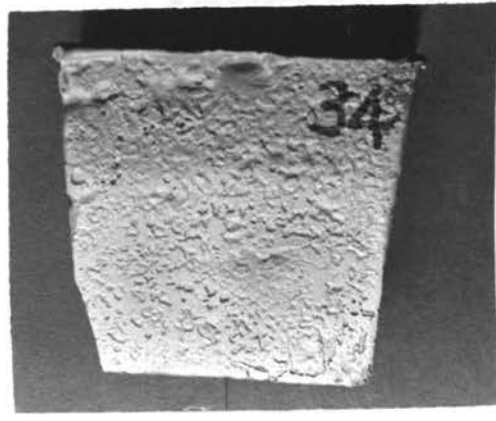
F. Casting #34 50% Magnetite (+325)
