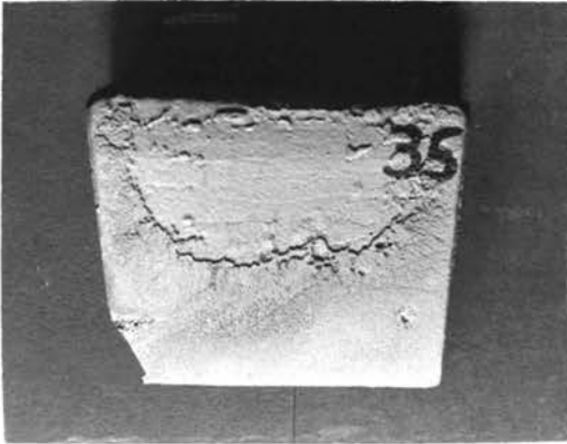
A. Casting #35 Silica Sand
