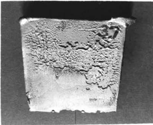
B. Casting #37 Silica Sand
