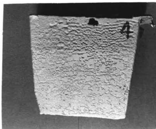
C. Casting #4 30% Magnetite (-325)
