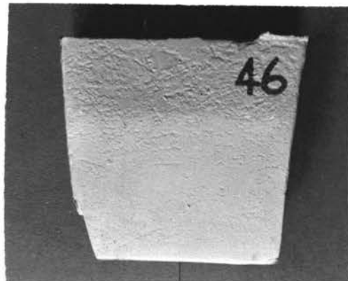
D. Casting #46 20% Magnetite (+200)
