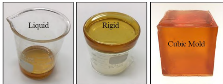
Figure 12. Pictures of the sealant in liquid, solid state and cured sealant in cubic form.
