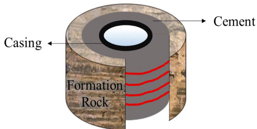
Figure 4. Cement dinking caused by axial shrinkage.
