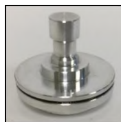
Figure 12. The cured sealant between the parallel plates.
