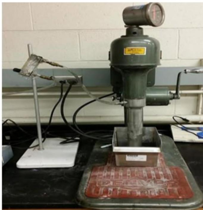
Figure 3.13 A photograph of denver flotation cell used in this study.
