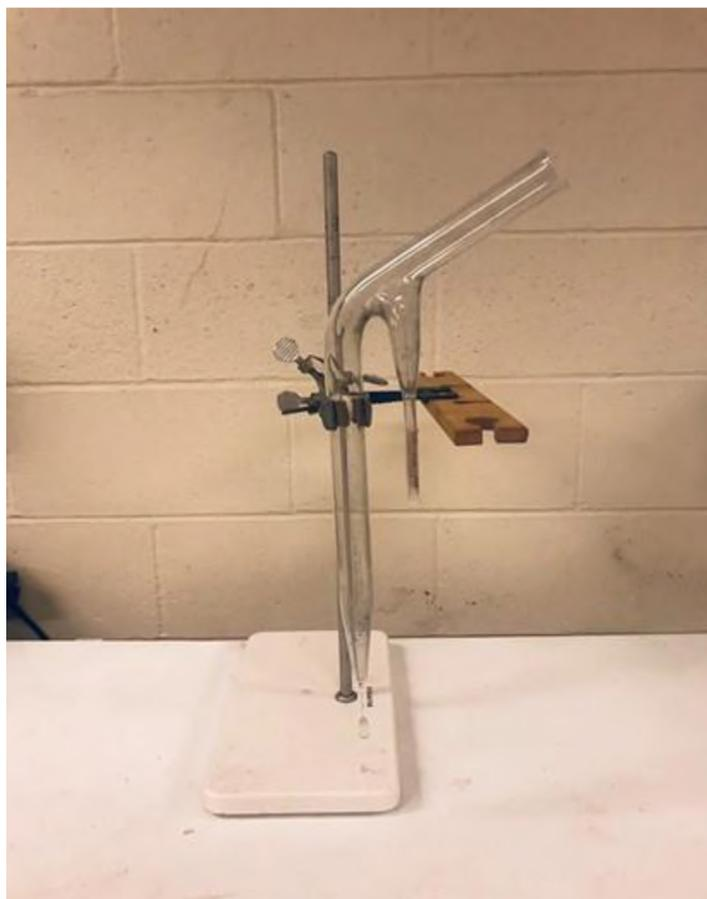
Figure 4.2 A photograph of hallimond micro-flotation tube used in this study.
