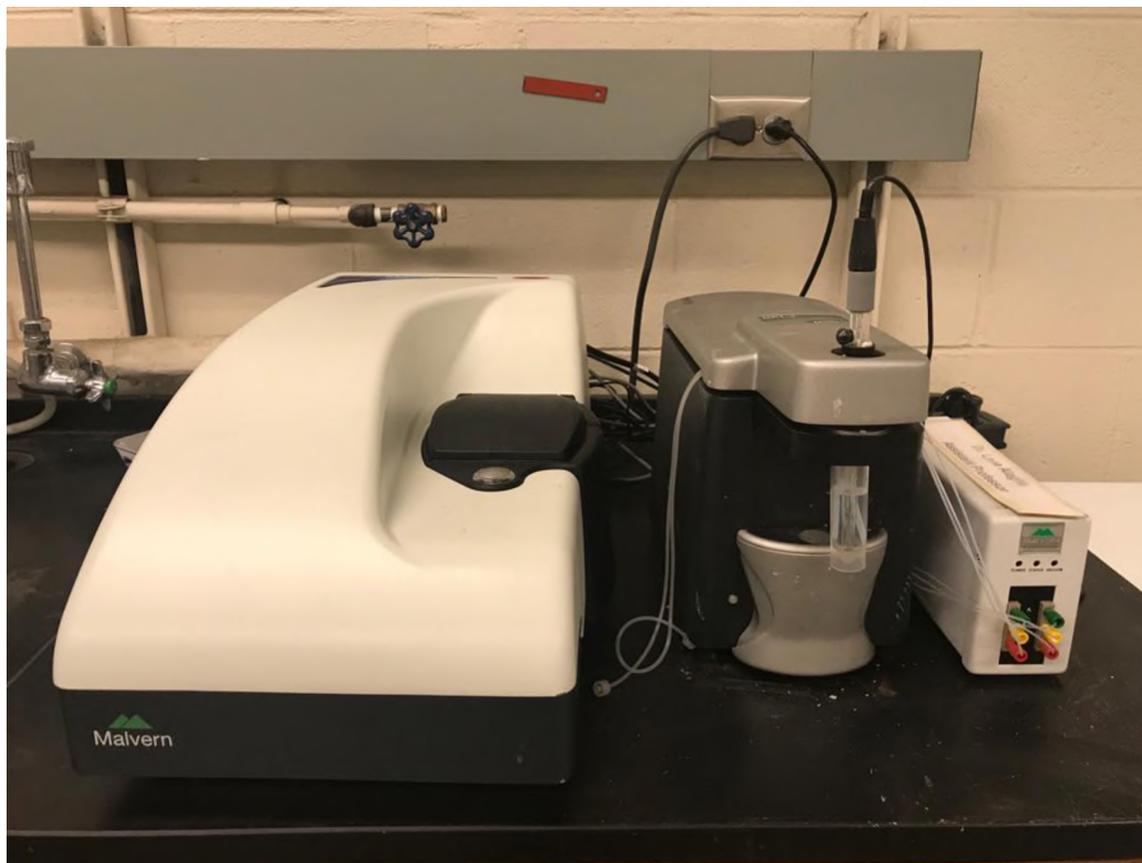
Figure 3.12 A photograph of zetasizer nano ZS instrument used in this study.
