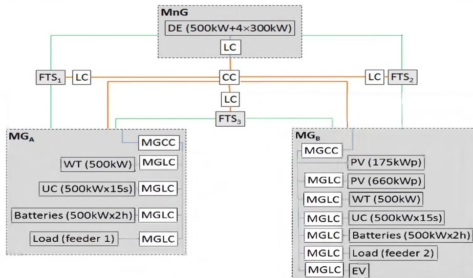
Figure 4.2 Configuration of the SoS network with dual microgrids and diesel engine generators.
