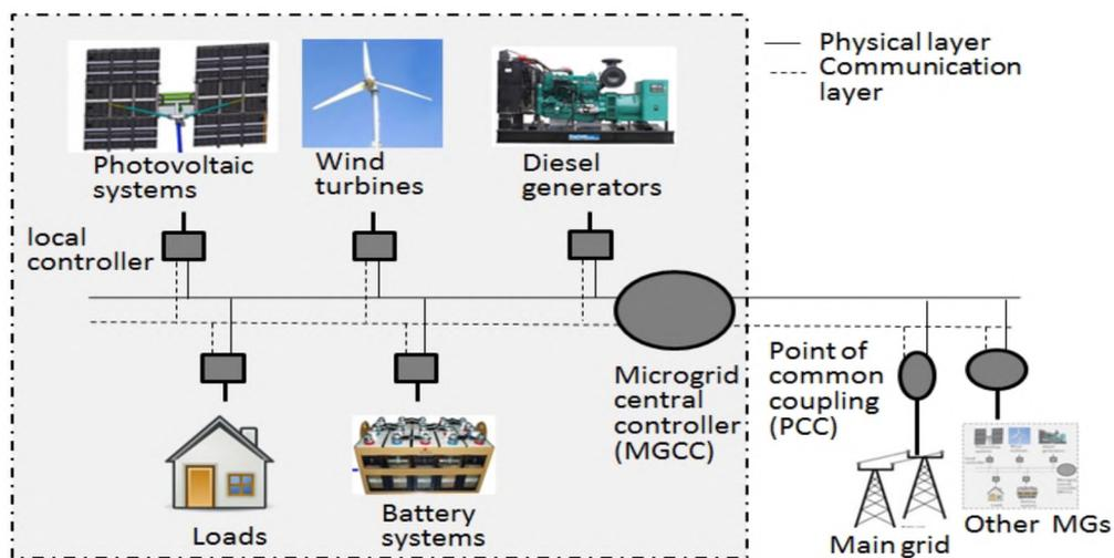
Figure 3.1 A microgrid with renewable energy sources.
