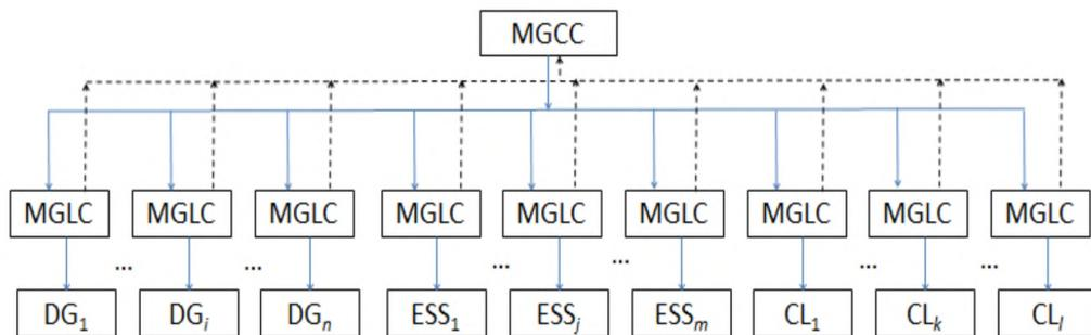
Figure 4.3 The schematic diagram of the hierarchical coordinating strategy for SoS.
