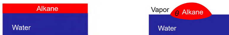
Figure 1.1. Two possible wetting configurations for alkane on water in bulk system: (a) perfect wetting (left) and (b) partial wetting (right).
