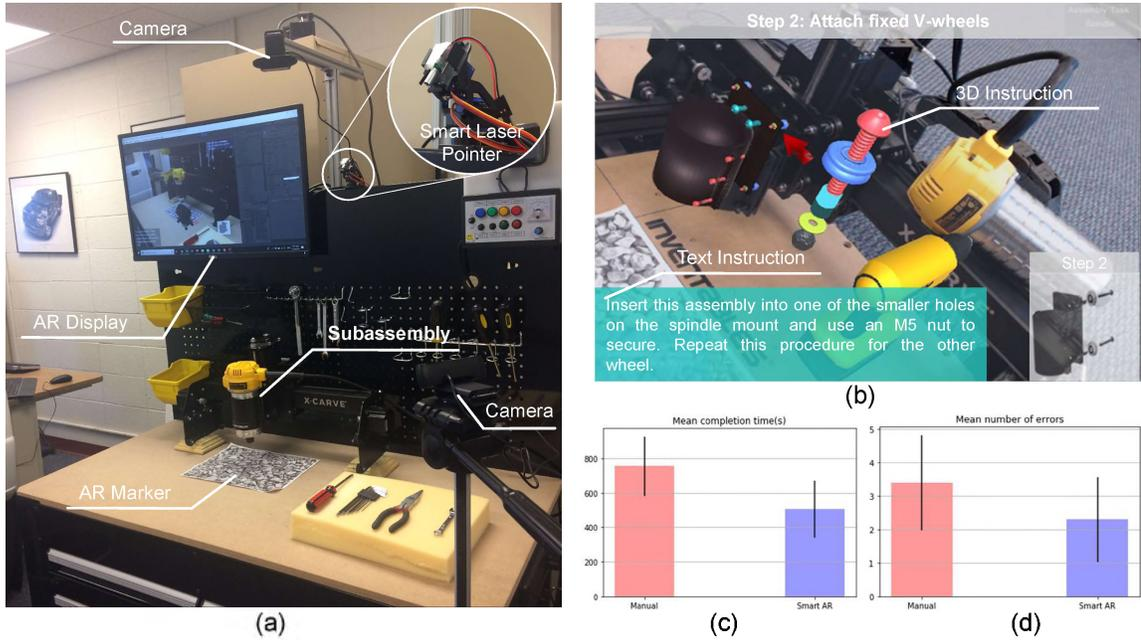
Figure 5. (a) Experimental setup; (b) AR display content; Performance comparison between manual and AR guidance: (c) completion time and (d) number of errors.
