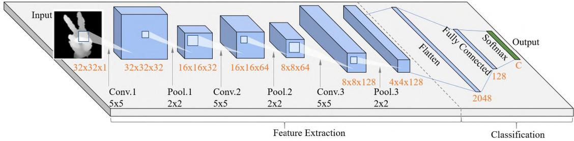
Figure 3. The overall architecture of our CNN model.
