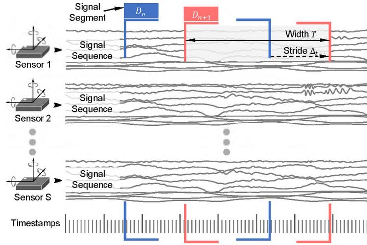
Figure 3. Scheme of the signal sampling method.
