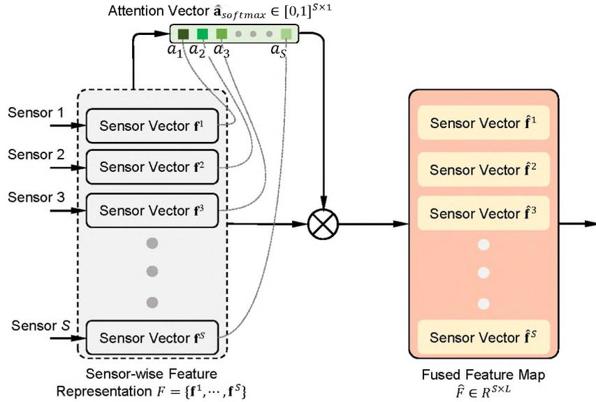
Figure 7. Illustration of the sensor attention mechanism.
