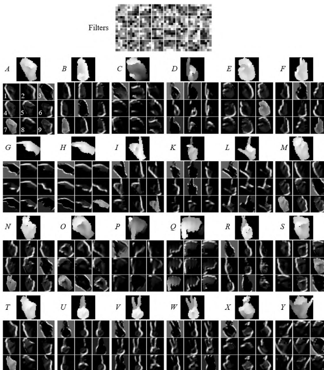
Figure 12. Visualization of the 32 ( $4 \text{ rows} \times 8 \text{ columns}$ ) learned filters (top) of the first convolutional layer, and the top 9 feature maps (the sequence is indexed as shown in A's feature maps) for each of the 24 signs in a trained model on the ASL benchmark dataset.
