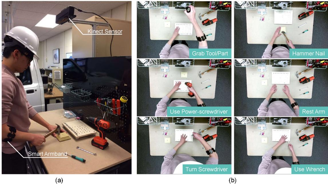
Figure 4. (a) Experimental setup and (b) examples of the six worker activities.
