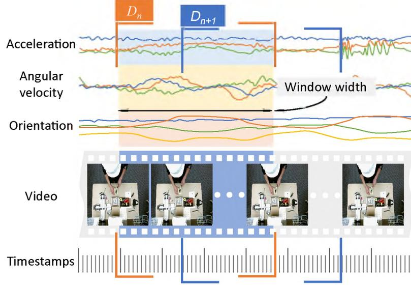
Figure 4. Scheme of the signal sampling method.
