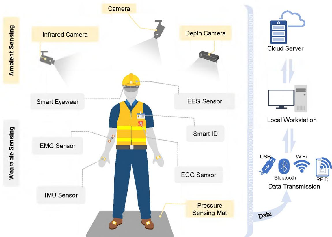
Figure 2. Schematic of the proposed multi-modal sensing system.
