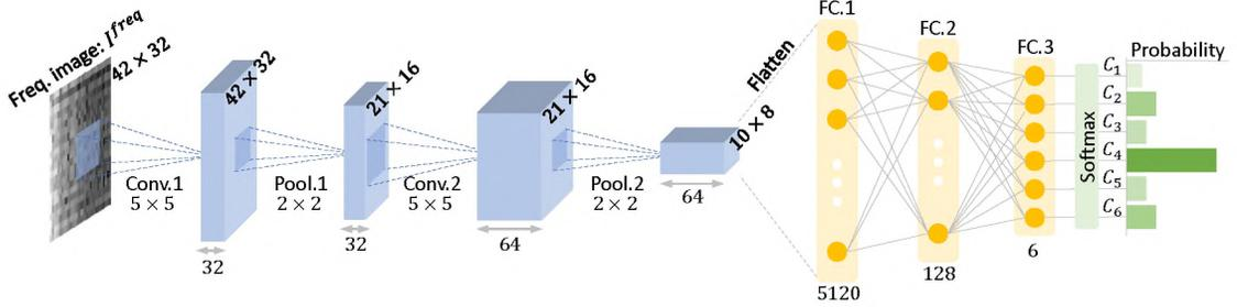
Figure 7. The architecture of our CNN model for  $I_n^{freq}$ .
