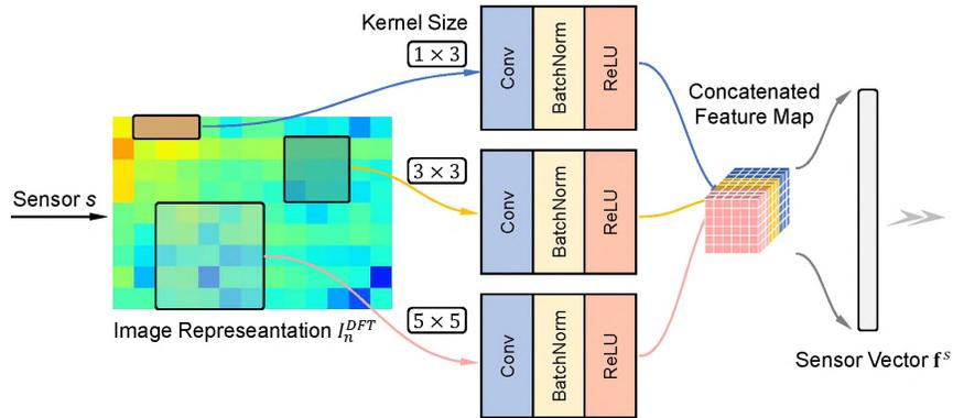
Figure 6. Illustration of the feature extraction module.
