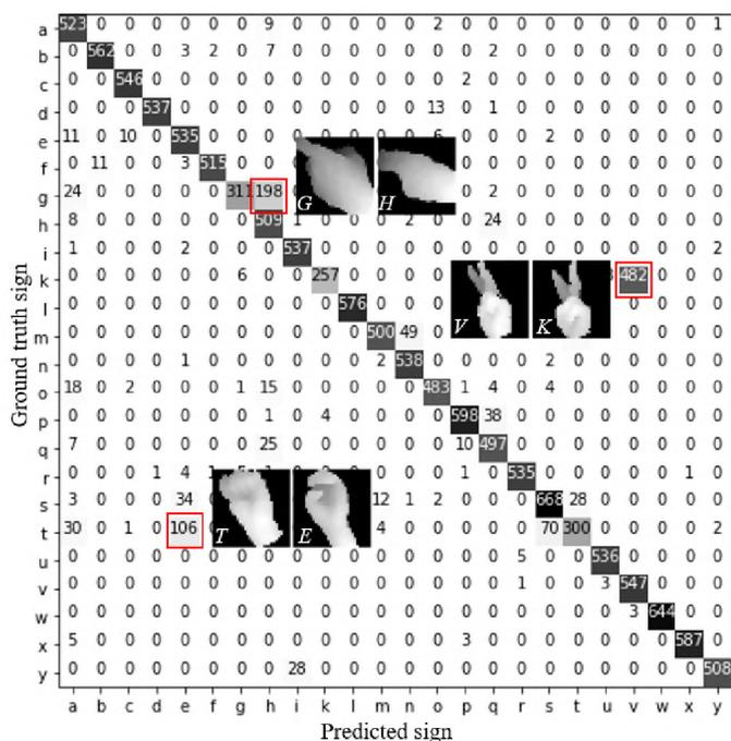
Figure 15. Confusion matrix and the most confusing pairs of the leave-one-out evaluation on the ASL benchmark dataset tested on the 2nd subject.
