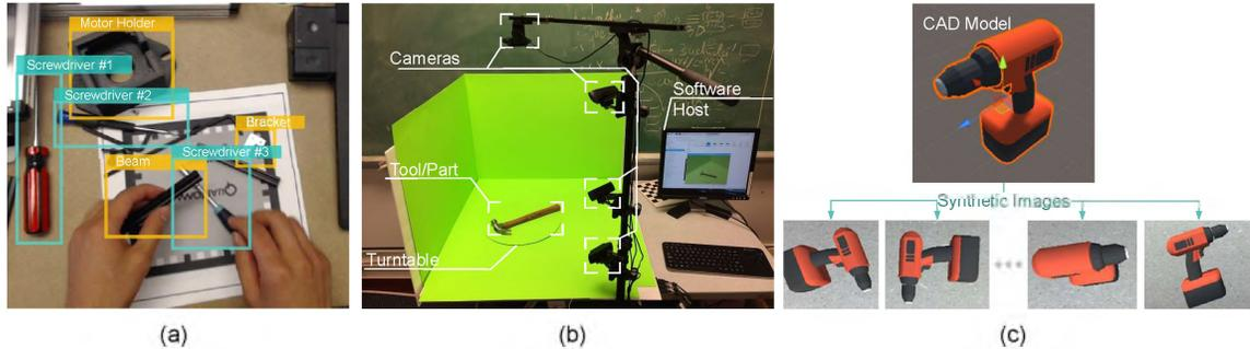
Figure 3. (a) Part/Tool detection results with highlighted bounding boxes; (b) Our developed data collecting system; (c) Image data synthesis rendered from a CAD model.
