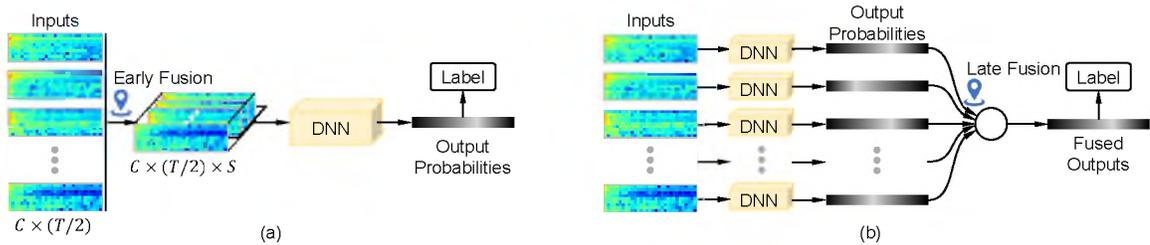
Figure 9. Architectures of different fusion methods.
