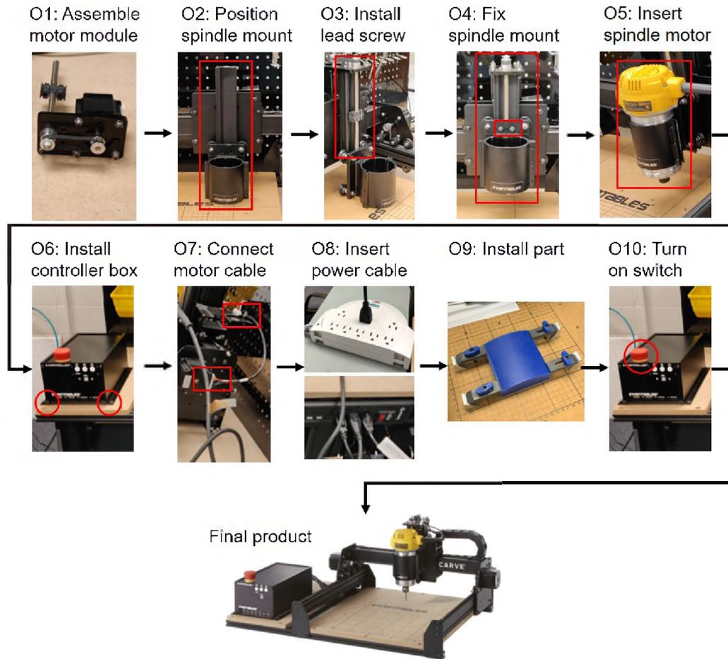
Figure 2. Illustration of the assembly task containing 10 operations from O1 to O10.
