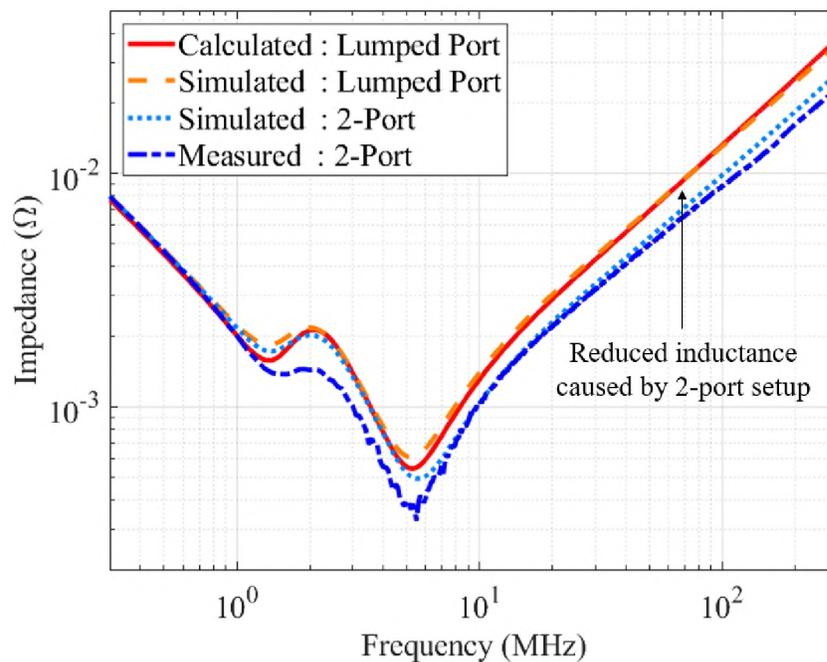
Figure 16. Comparison of the PDN impedance for the whole PCB structure.
