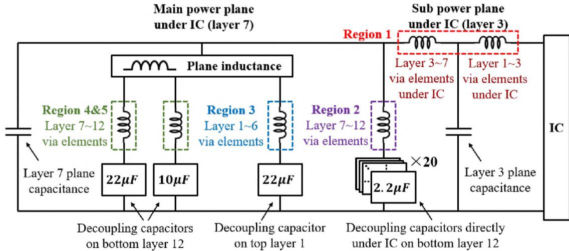
Figure 12. The equivalent circuit corresponding to the PCB under investigation.
