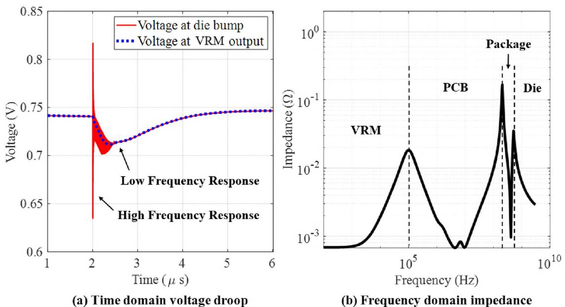
Figure 2. System-level PDN performance.
