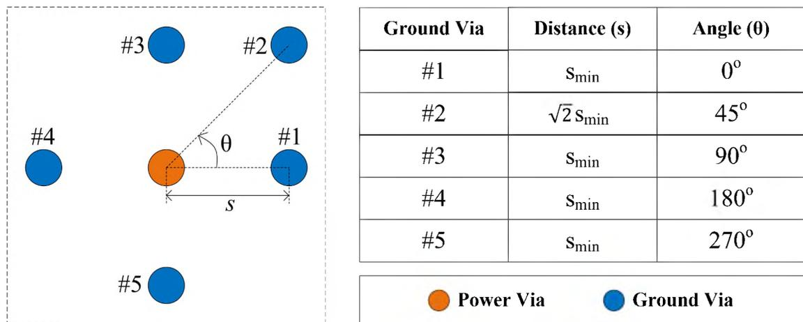
Figure 3. Localized via pattern around the power via.
