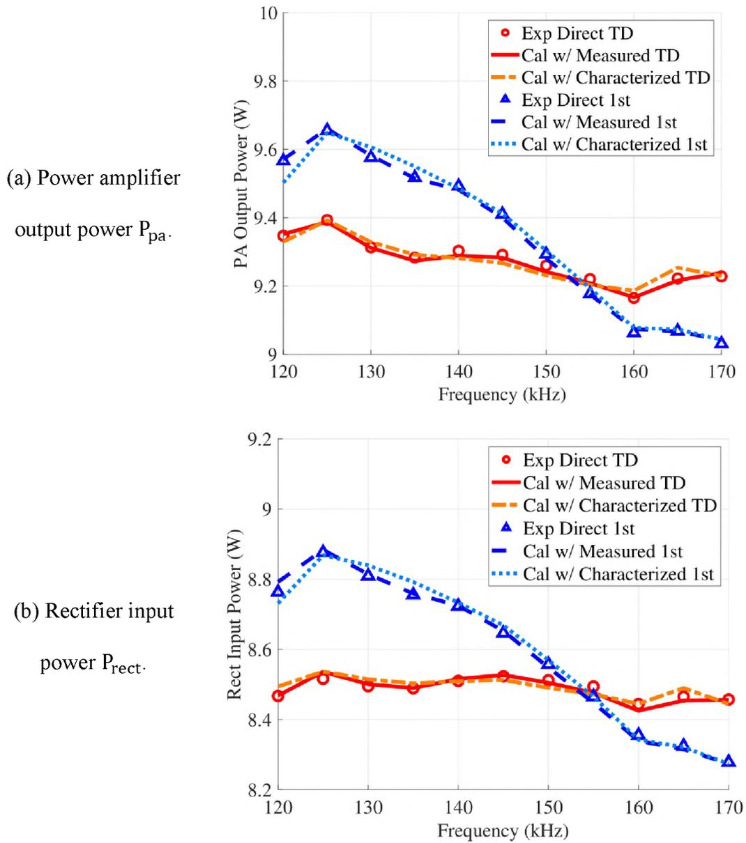
Figure 13. Comparison of intermediate ac powers.
