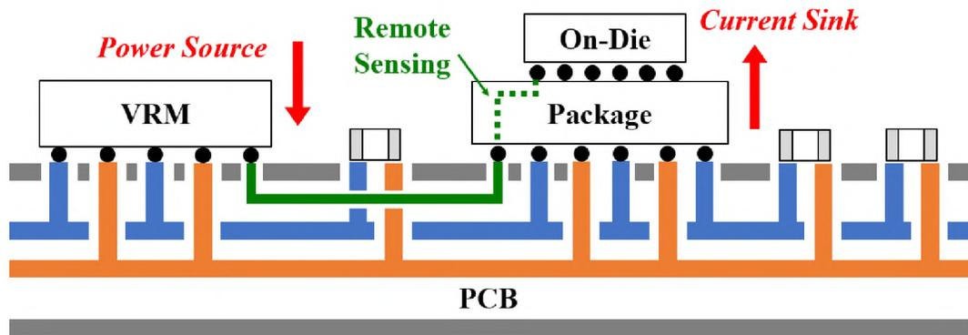
Figure 1. Main elements in the end-to-end PDN.
