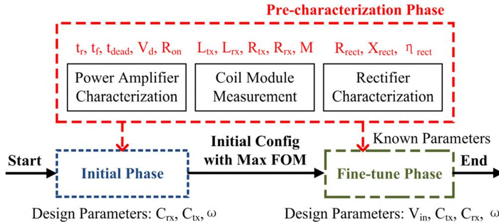
Figure 10. Flowchart of the design methodology.
