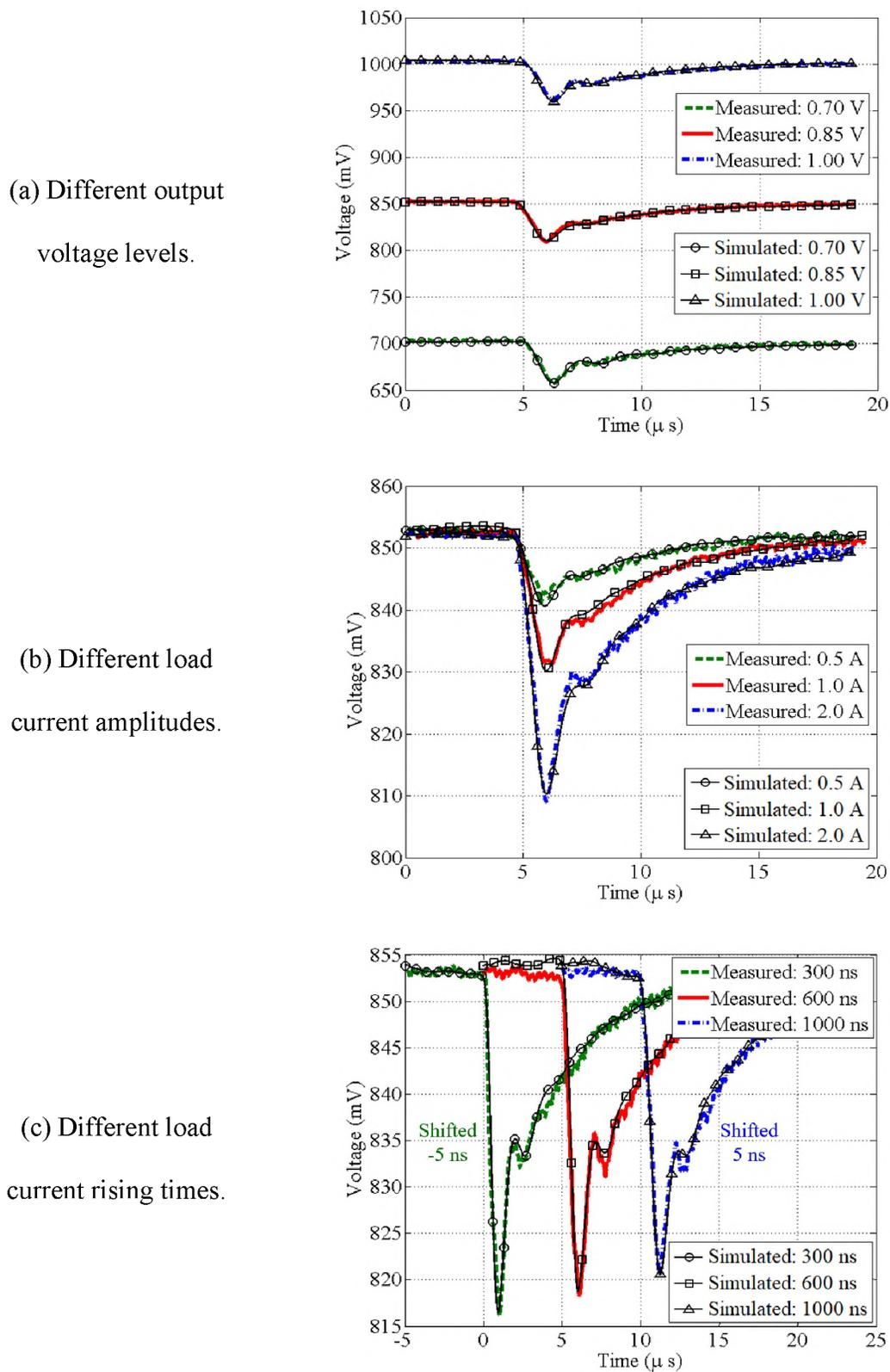
Figure 11. Comparison of voltage droop waveforms for single-phase VRM.
