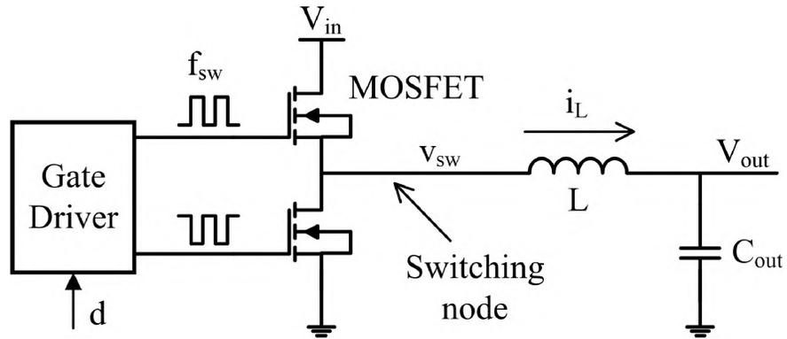
Figure 3. Diagram of an open-loop dc-dc buck converter.
