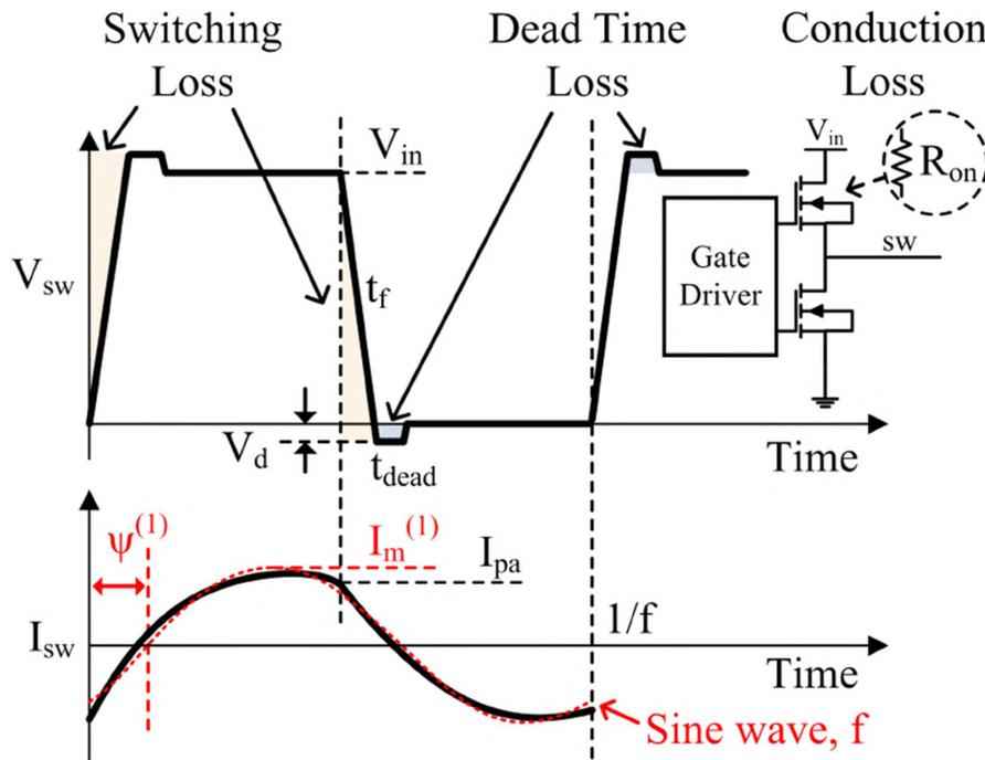
Figure 9. Time-domain voltage and current waveforms at the switching node.
