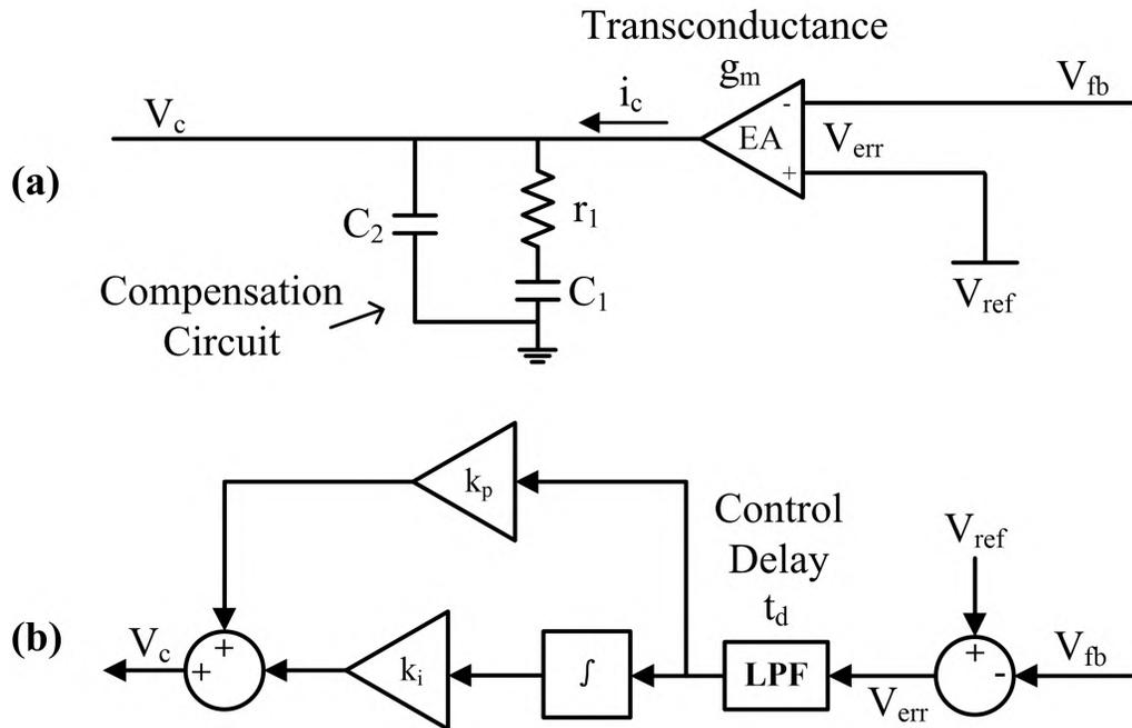
Figure 5. Modeling of the voltage control loop.
