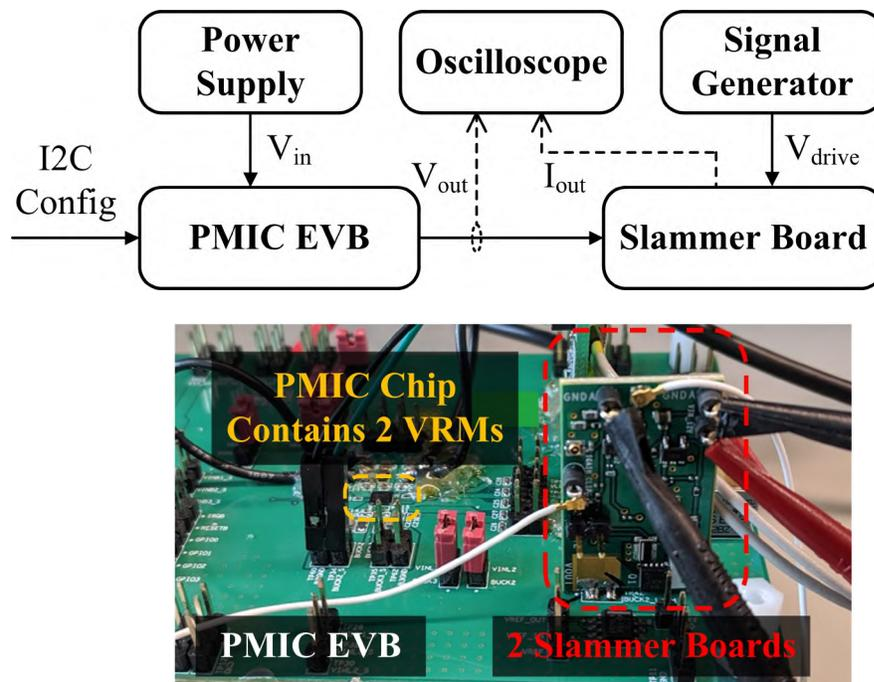
Figure 8. Diagram and photograph of the measurement setup.
