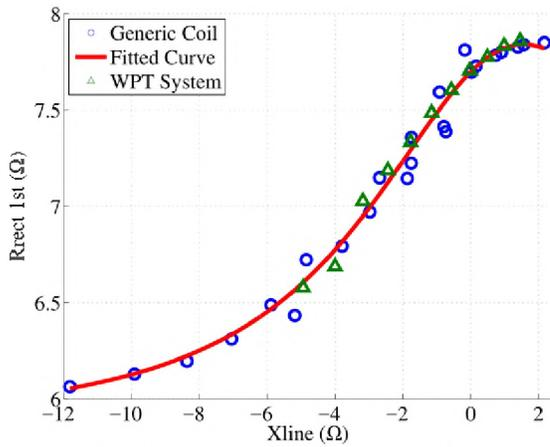
(a)  $R_{\text{rect}}$  1<sup>st</sup> Frequency vs.  $X_{\text{line}}$
