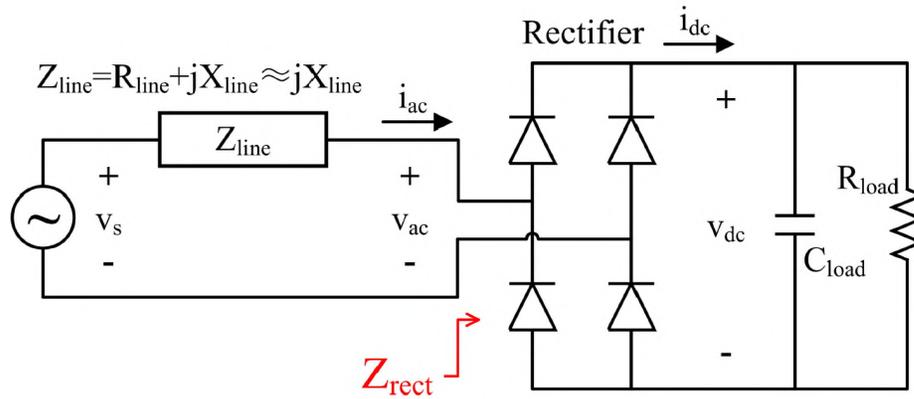
Figure 4. Circuit model of a full-wave diode rectifier.
