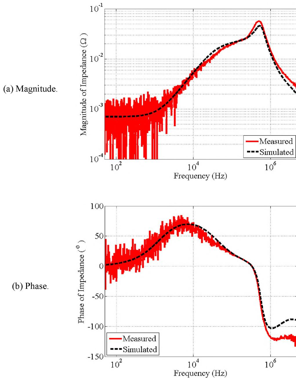
Figure 13. Comparison of simulated and measured impedance for single-phase VRM.
