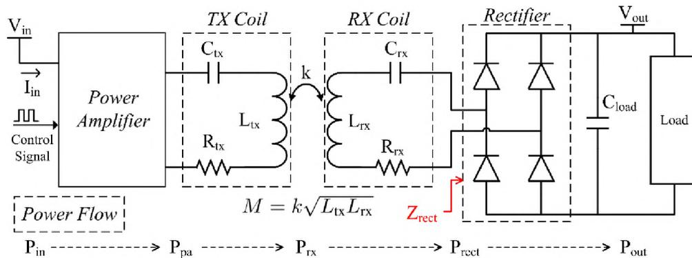
Figure 1. Typical WPT system with the SS topology.
