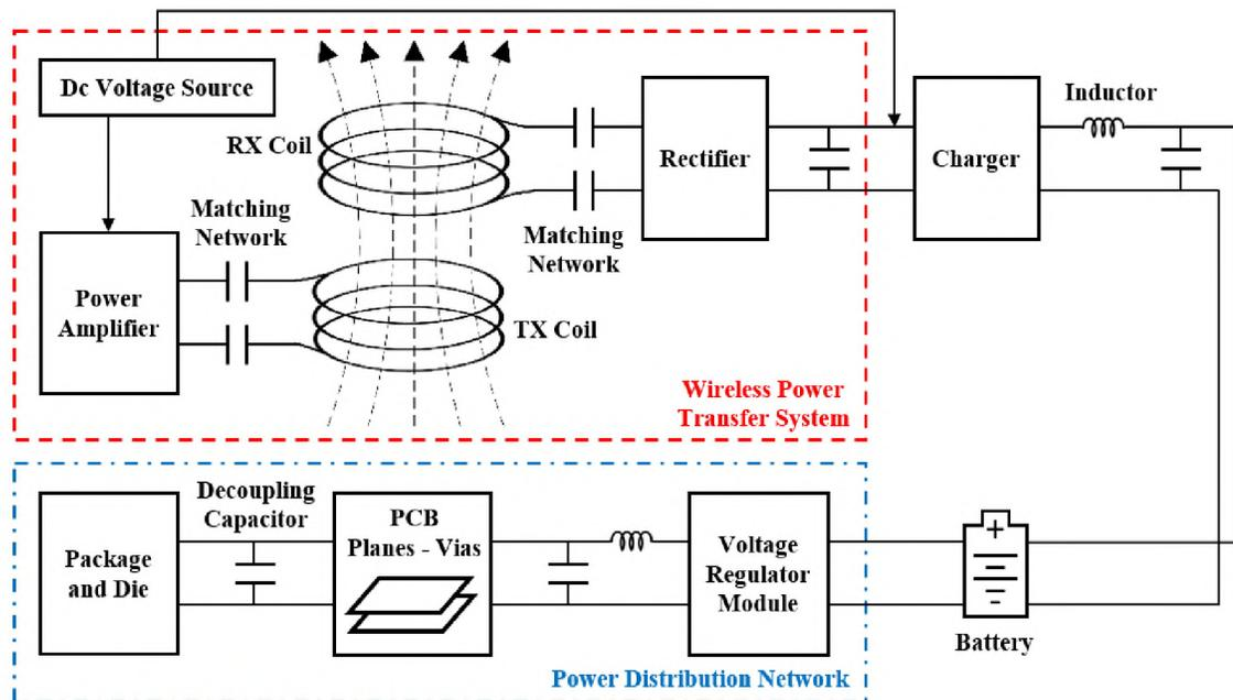
Figure 1.1. Power delivery paths in electronic devices.
