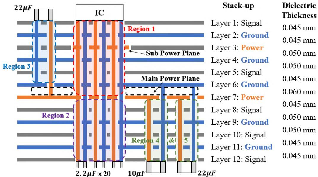
Figure 11. Physical geometry and region division of the mobile phone PCB.
