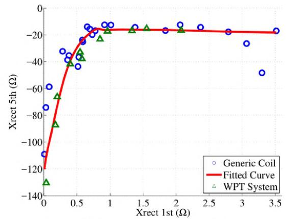
(f)  $X_{\text{rect}}$  5<sup>th</sup> Frequency vs. 1<sup>st</sup> Frequency
