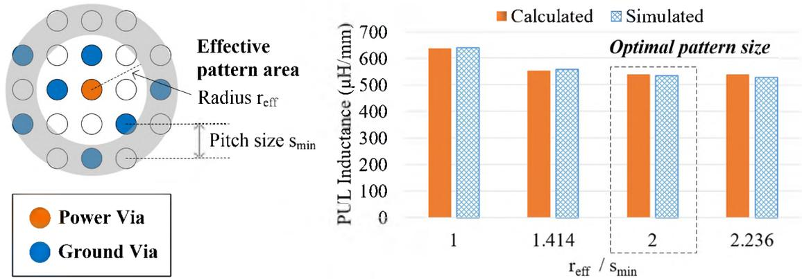
Figure 13. Selection of the optimal pattern size.
