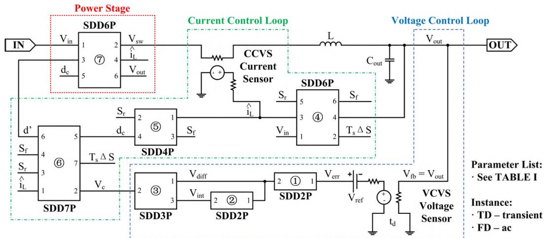
Figure 7. Schematic of the behavior model in the circuit simulator.
