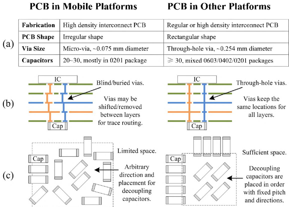
Figure 1. Comparison of PCB in mobile platforms and PCB in other platforms.
