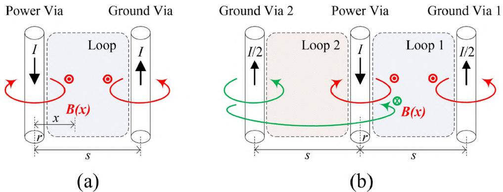
Figure 5. Magnetic flux through the loop formed by adjacent vias.
