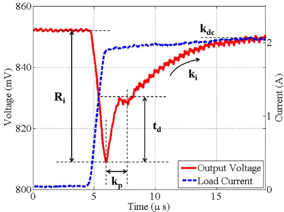
Figure 9. Measured voltage and current waveforms for characterization.
