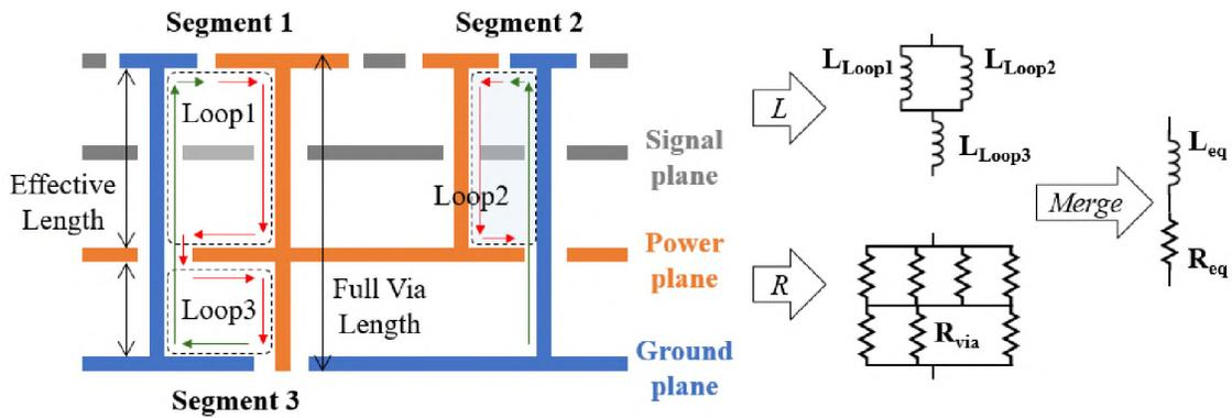
Figure 14. Calculation of the equivalent inductance and resistance in one region.
