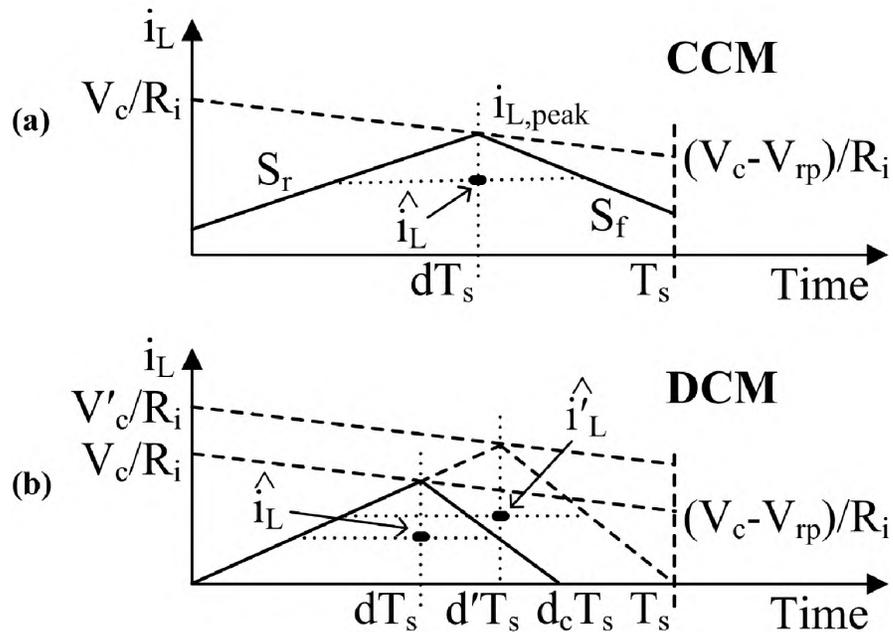
Figure 6. The inductor current in one switching period.
