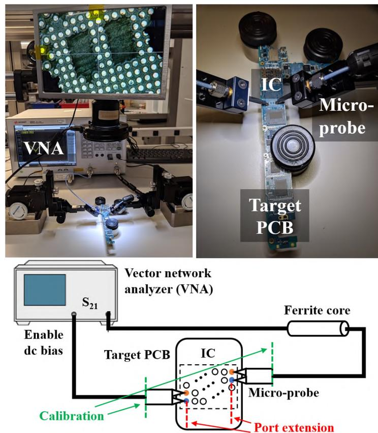
Figure 15. Photograph and diagram of the shunt-thru measurement setup.
