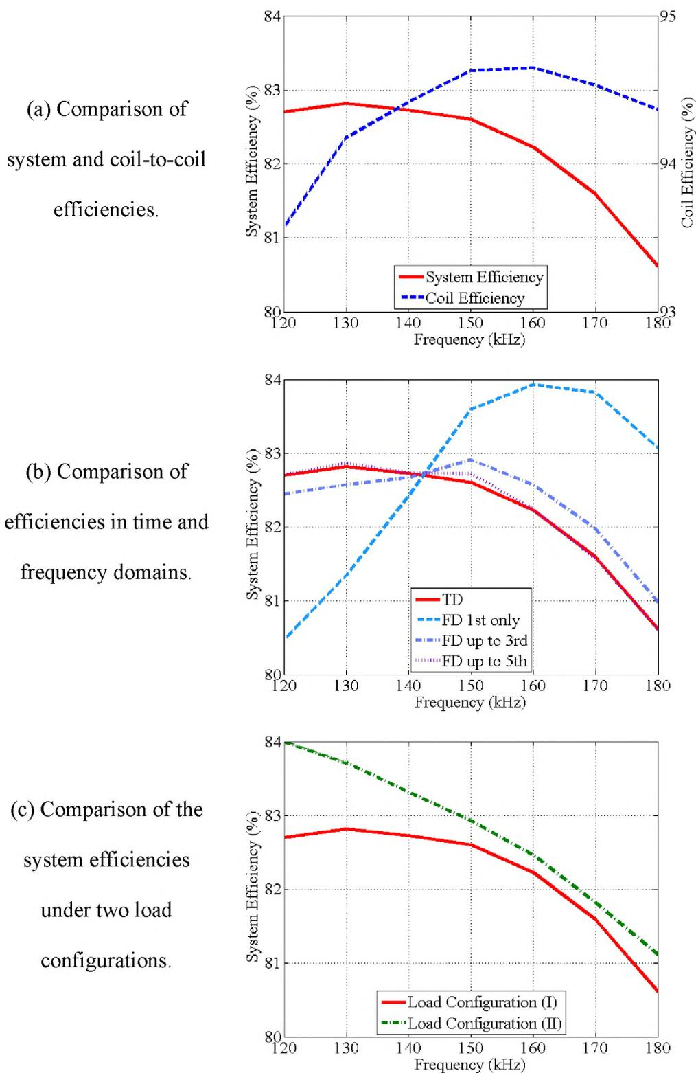
Figure 3. Simulation results of the circuit model.
