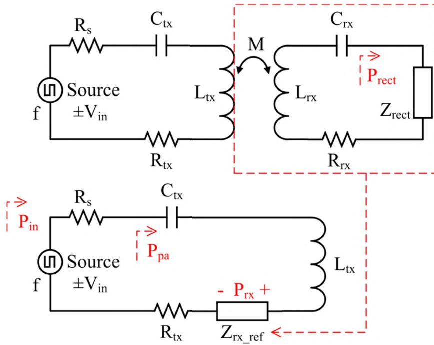
Figure 8. Formulation for the improved modeling of the WPT system.
