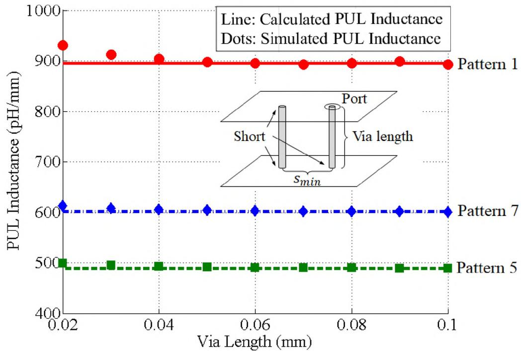
Figure 9. Simulation results of via inductance for different via lengths.
