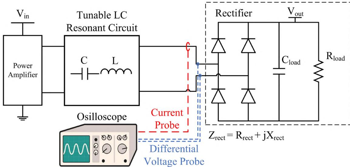
Figure 6. Measurement-based rectifier impedance characterization setup.
