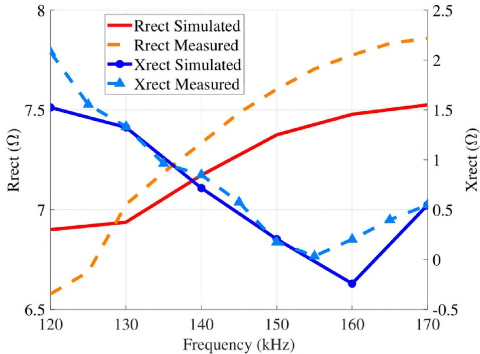
Figure 5. Comparison of simulated and measured rectifier impedance.
