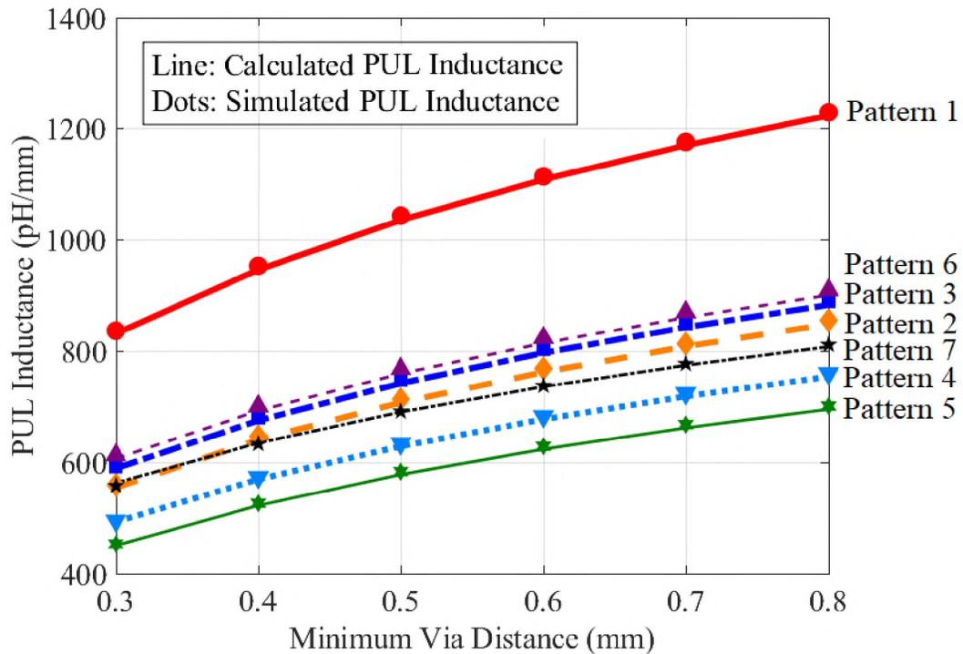
Figure 8. Comparison of via inductance for different patterns and distances.
