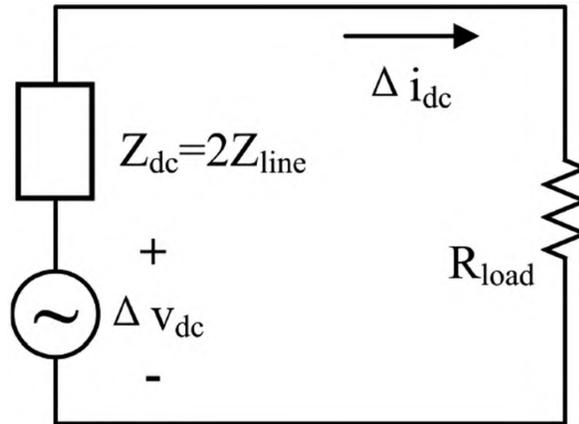
Figure A.1. Thevenin equivalent circuit for the output side of the rectifier.
