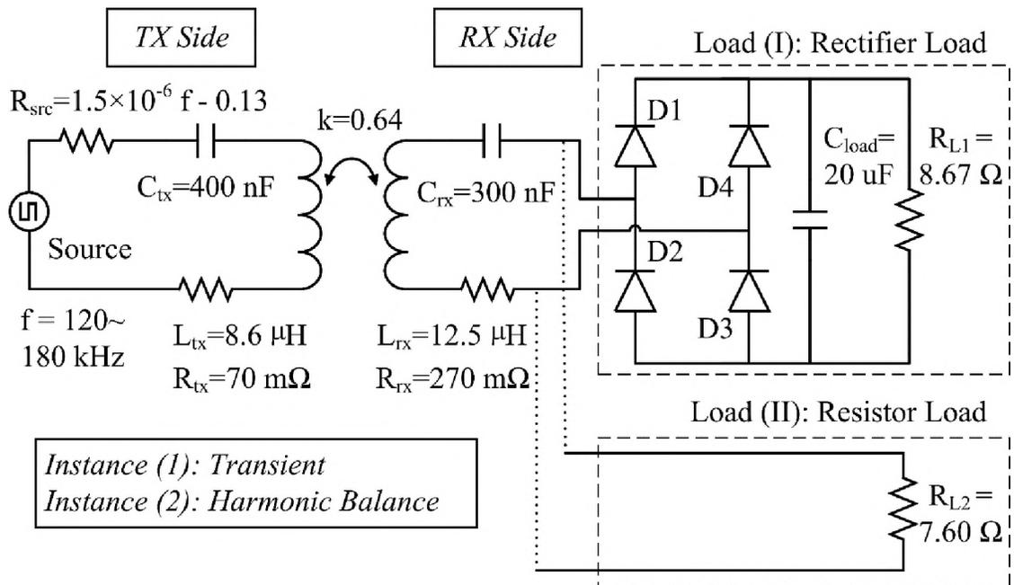
Figure 2. Diagram of the circuit model for preinvestigation.
