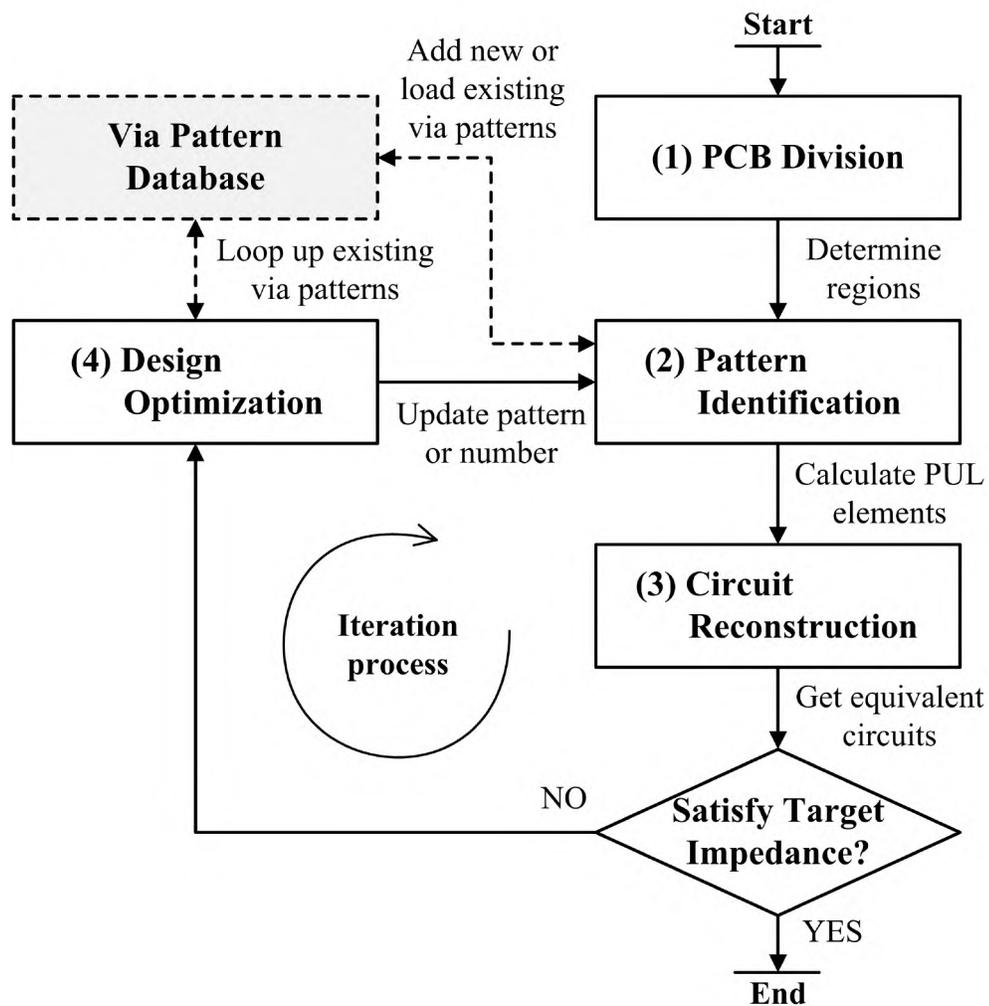
Figure 10. Flow diagram of the modeling methodology.
