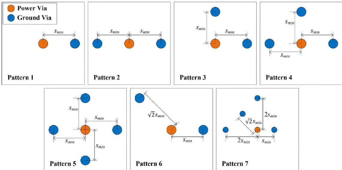
Figure 7. Arbitrary via patterns for validation.
