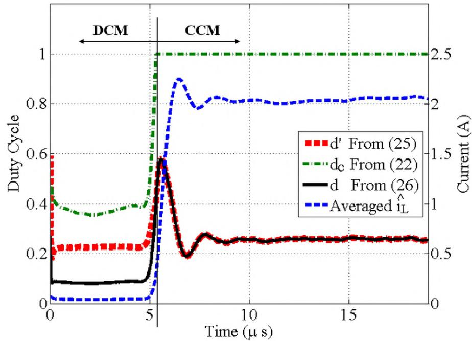
Figure 10. Validation of the unified equations for the CCM and DCM.
