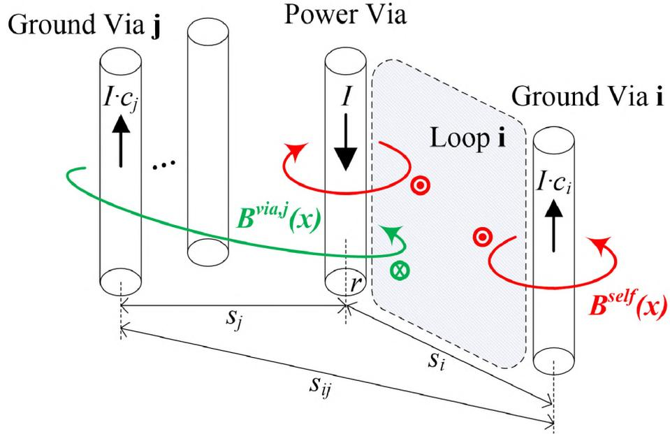
Figure 6. Illustration of the magnetic flux for an arbitrary via pattern.
