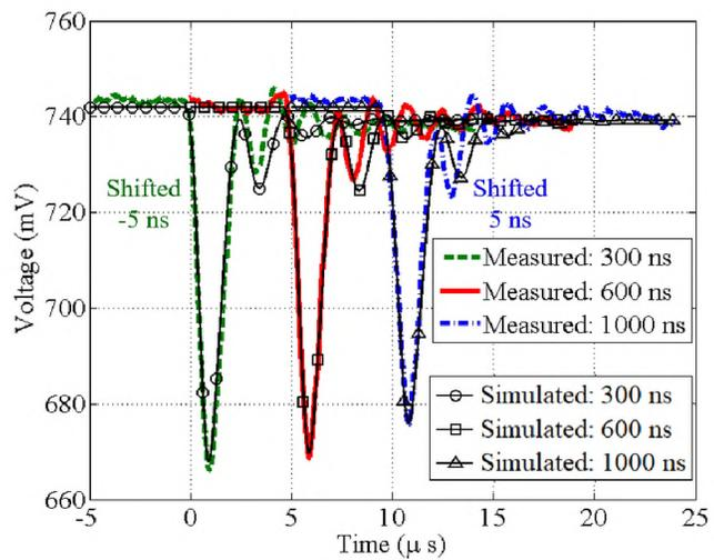
Figure 12. Comparison of voltage droop waveforms for 3-phase VRM.
