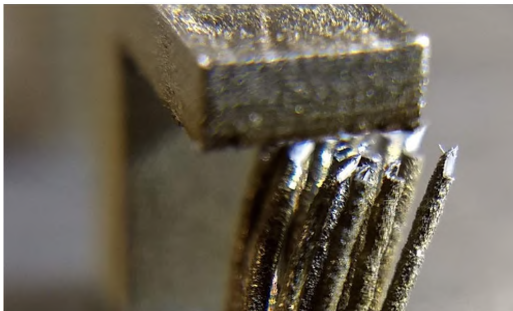
(a) The lower density support structures tended to deflect during the machining operation.
