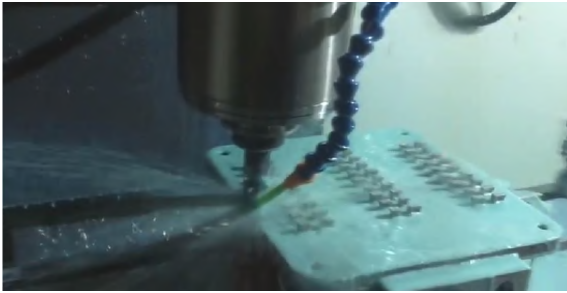
(a) Support removal was accomplished via a 2" diameter, 3/32in thick slitting saw.
