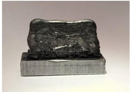
(b) FIRST: Thin wall deposit with the feedback system on, prior to PID loop fine tuning.
