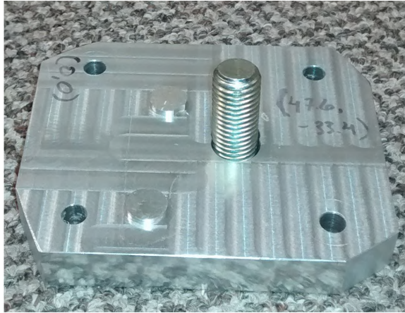
Figure 3. Aluminum fixture machined to hold the core on a 5th axis trunnion.
