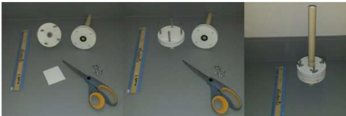
Figure S4. Experimental set up of a custom-made PVC column to sandwich CA membrane without and with PCL NPs in between two flow pipes. A piece of membrane was screw tightened between two flow pipes (top and bottom). Water and LPS containing water was fed on the top PVC pipe and let it flow by gravity. The permeability of membrane and % LPS removal were assessed using this set-up.
