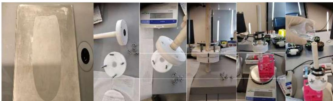
Figure S7. Custom-made membrane filtration set up made out of PVC. CA biofilter without and with PCL NPs are sandwiched between two blocks and butterfly screws are used to tighten the biofilter. Endotoxin spiked protein solution is fed from the top part of the pipe and permeate is collected from the bottom half of the pipe.
