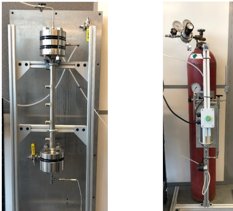
Figure C.4. Experimental setup used for Residence Time Distribution experiments using Liquid Tracer
