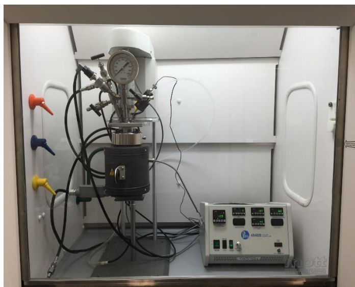
Figure C.3. Mini Basket Reactor - 300mL volume with Basket and Slurry compatibility, Maximum T-500°C and P-2000 psig
