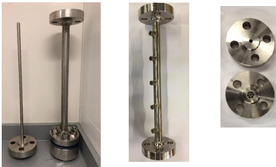
Figure C.2. Reactors (From left) Thermowell reactor, 1 inch ID, 60 cm long, Thermowell 1.4 cm OD, 54 cm long; reactor with distributor 1 inch ID, 60 cm long; gas-liquid distributor
