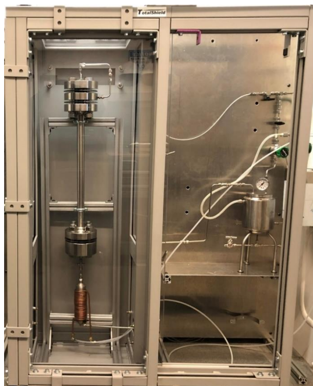
Figure C.1. High Pressure High Temperature Experimental facility with explosion shield
