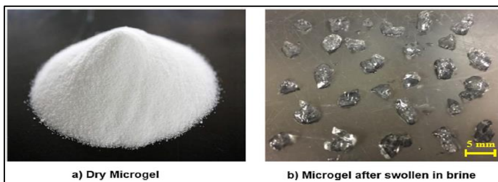
Figure 2.18. PPG before and after swelling in seawater (Alhuraishawy et al., 2018).
