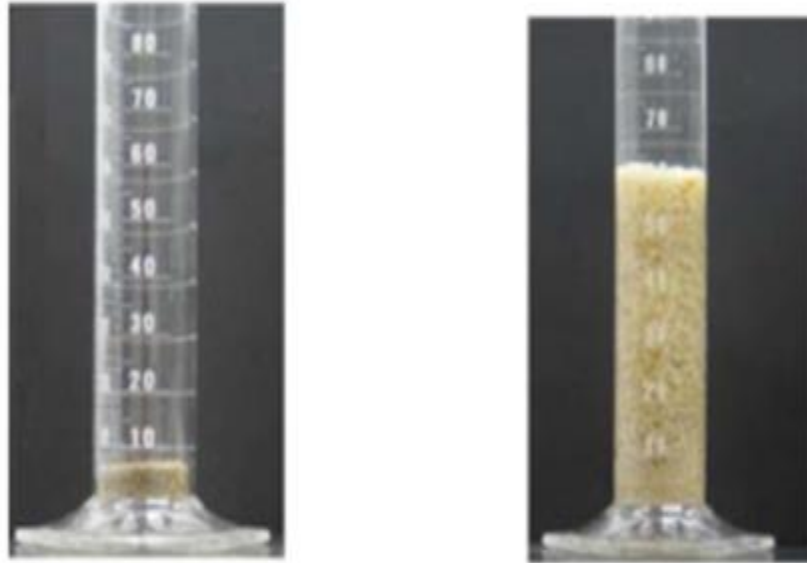
Figure 2.2. Comparison of millimeter PPG before and after swelling (40) Left tube: dried particles; right tube: swelling particles
