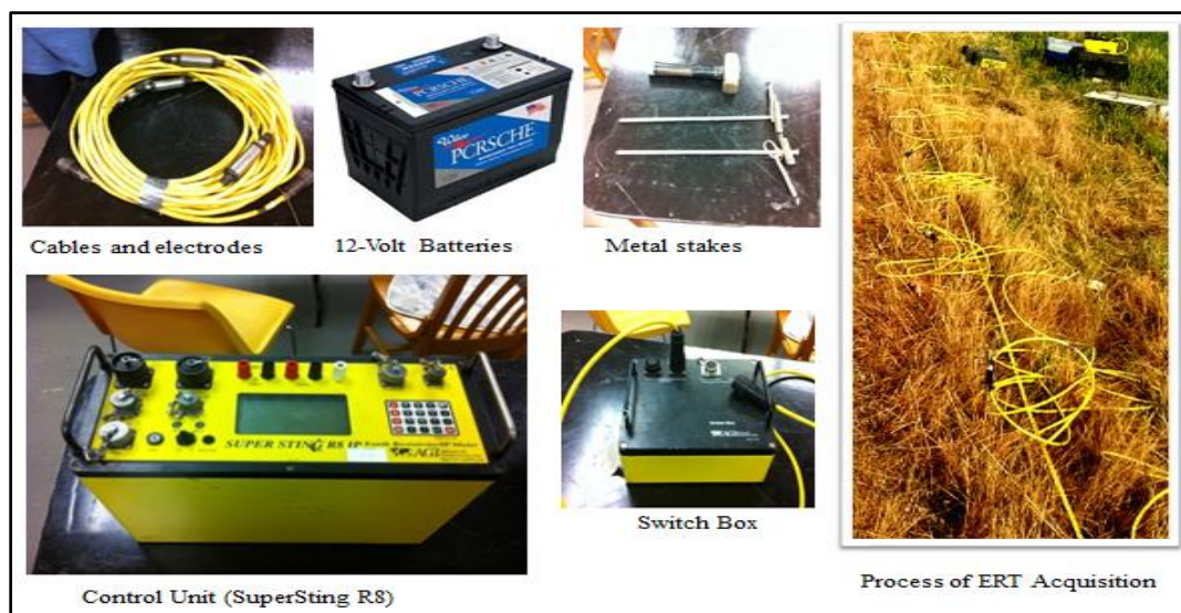
Figure 4.1. The equipment used for ERT data collection.
