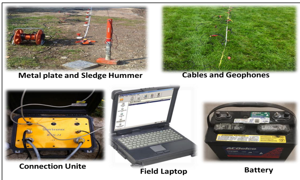
Figure 3.13. MASW equipment's and tools.
