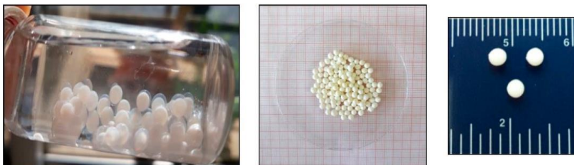
Figure 1.4. Polyurea wet-gel beads soaked in acetone (before drying) (left) and polyurea aerogels beads after supercritical drying (middle and right). 65
