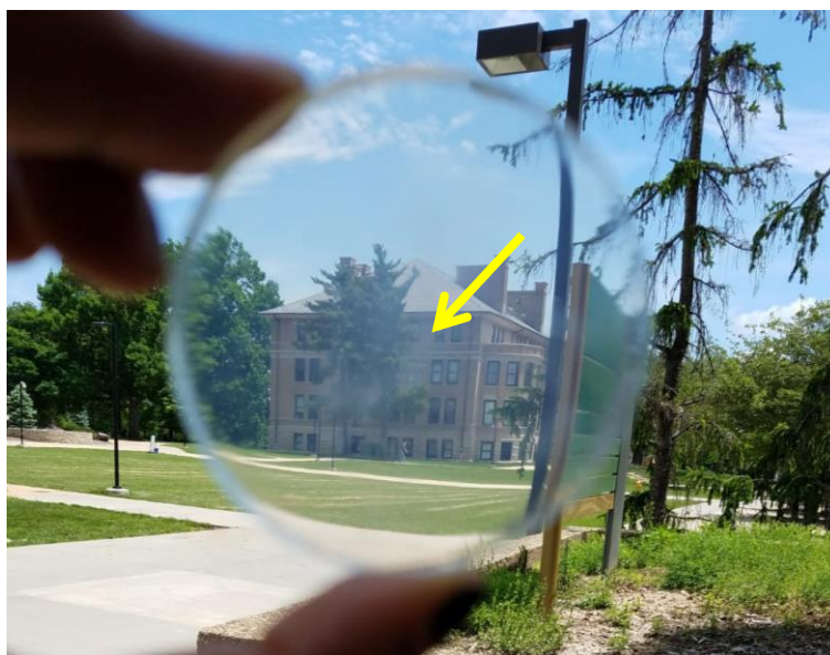
Figure 2. (A) Photograph of a K and a K/2 aerogel monolith in front of text. (B) An aerogel monolith of standard formulation (K) in front of landscape. Slight lensing is due to the curved surface of the monolith that was created by the meniscus of the sol. Yellow arrow points to surface scratches caused by handling
