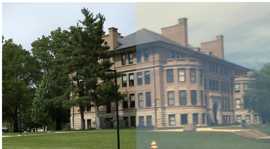
Figure 9. Unobstructed view and view through a cross-linked TMOS-co-APTES aerogel sample fabricated with the formulation shown with an arrow in Figure 6 (0.875,4.5).
