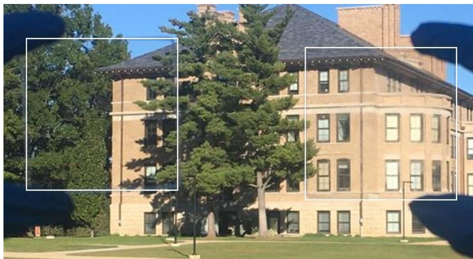
Figure 1.15. Picture comparing the clarity through a clean glass plate (left) and silica sol-gel coated glass plate (right)
