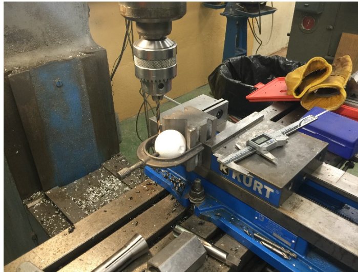
Figure 4.7 To fix the sphere scanning target to the metal rod and keep the three-dimensional error of scanning results to a minimum, all spherical targets used in this research are drilled precisely through their centers to let the rod pass precisely through the center of the sphere target.
