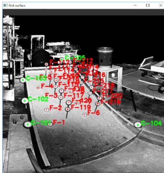
Figure 6.3 The scan result of the bench model by Lidarsw; the red targets are the floating targets and the green targets are the control targets.
