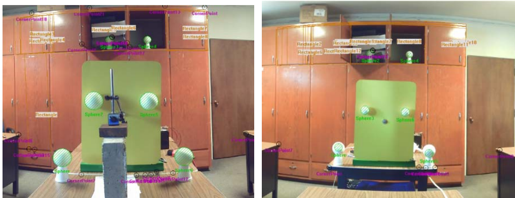
Figure 4.3 The controlled displacement device and the scanning targets. The spherical targets on the metal plate are the floating targets and the spherical targets on the table are the control targets. (a) The diameter of the floating target is 10.16 cm (4 inch); (b) The diameter of the floating target is 6.35 cm (2.5 inch).
