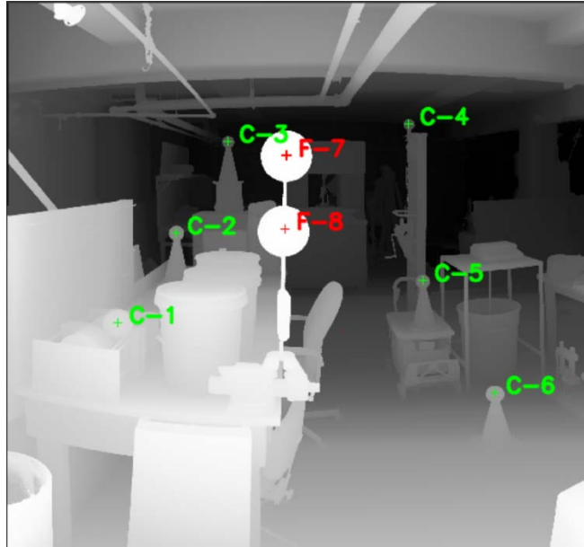
Figure 4.10 The scan points cloud figure shows the position of the control targets and floating targets. The green targets are the control sphere references and the red targets are the floating sphere targets. Green “C” is used to identify the control target; red “F” is used to identify floating targets in Lidarsw; and the number is the ID of the scanning targets.
