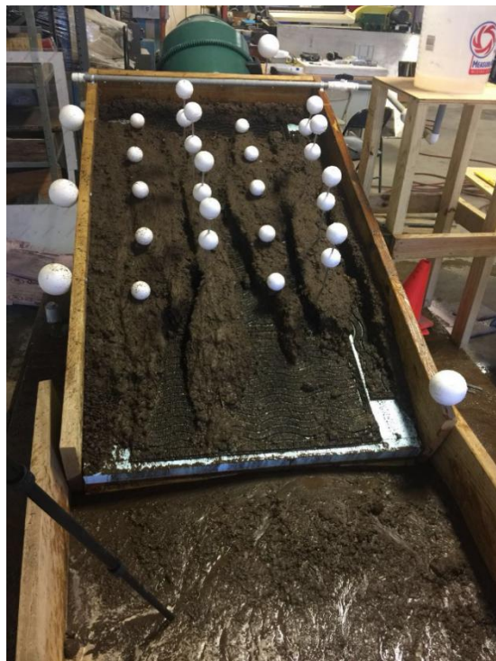
Figure 6.14 The gullying on the soil slope in bench model test. This is the scanning result from the late stage of the bench model test 6-2 and the gullying is generated by the water injection on the top of the slope. Therefore, the displacement of some scanning targets and the rotational angle of some scanning target rods are abnormally increasing. The abnormal scanning results have been deleted from the database.
