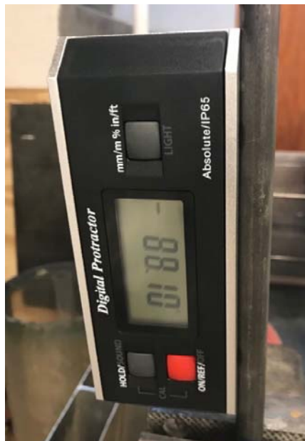
Figure 3.6 The digital protractor used in the research to monitor the rotational angle of the scanning target rod
