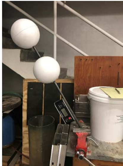
Figure 4.8 The designed scanning target which include two floating target spheres on a metal rod that can be rotated in one direction. A digital protractor is attached to the target rod to verify the angle changes.
