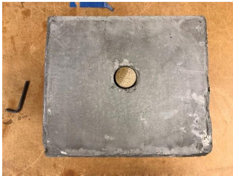
Figure 15. Paste sample with artificial defect (dowel).
